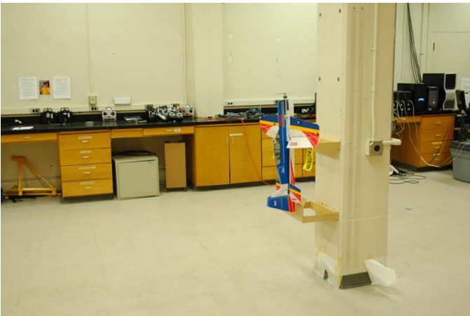
Figure 9: Autonomous landing in hover mode – perching on the fixed landing platform on a cement pole
