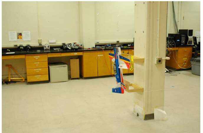
Figure 9: Autonomous landing in hover mode – perching on the fixed landing platform on a cement pole
