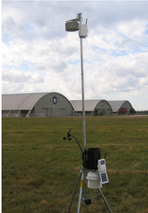
Figure 15. Davis Vantage Pro2 Plus weather station. Two levels of temperature and humidity, one level of pressure and wind are given. Two levels of wind are extrapolated as needed for the model by assuming a linear wind profile and that wind being zero at height zero.
