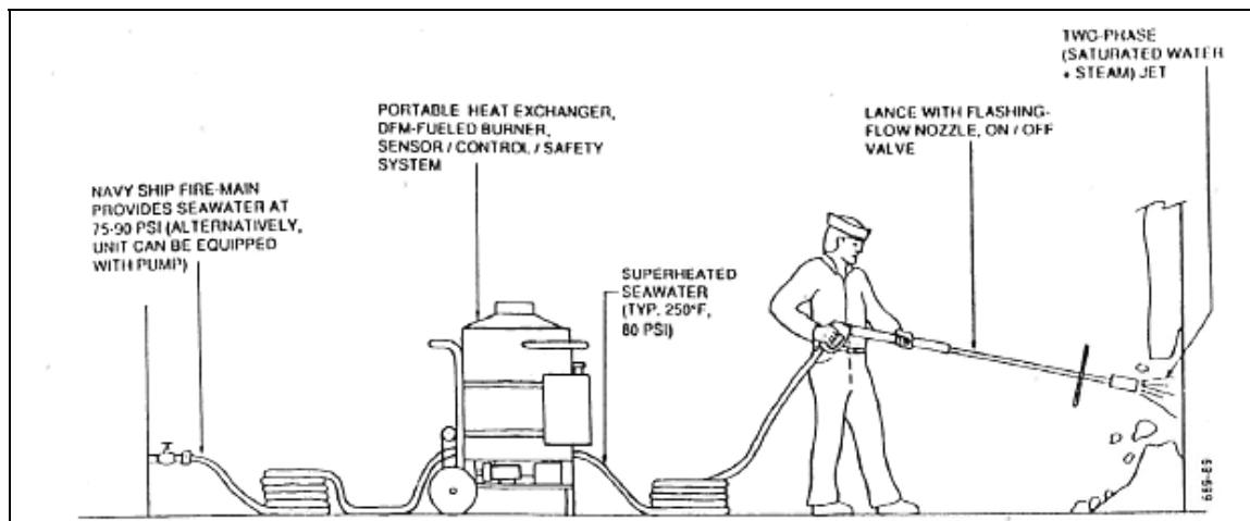
Figure 38. Flash flow portable deicing system for ships.
