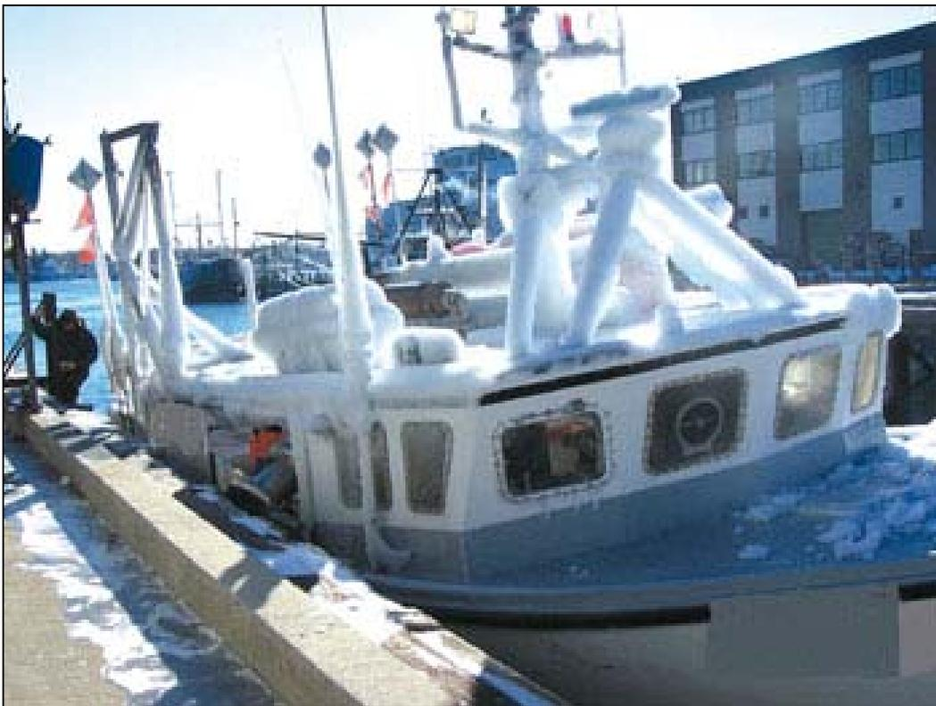
Figure 18. Superstructure ice covering life rafts, antennas, and windows of small trawler-size boat. (Photographs courtesy Kevin F. Plowman, USCG).
