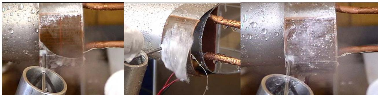
Figure 45. Ice being removed from surface coated with piezometric crystals, left to right.
