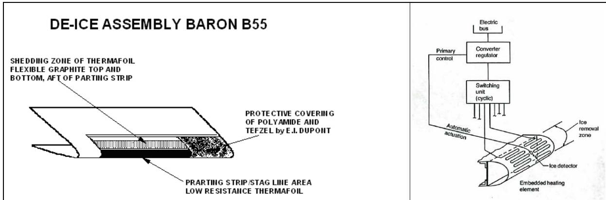
Figure 34. Graphite conductor electrothermal system by Northcoast technologies.
