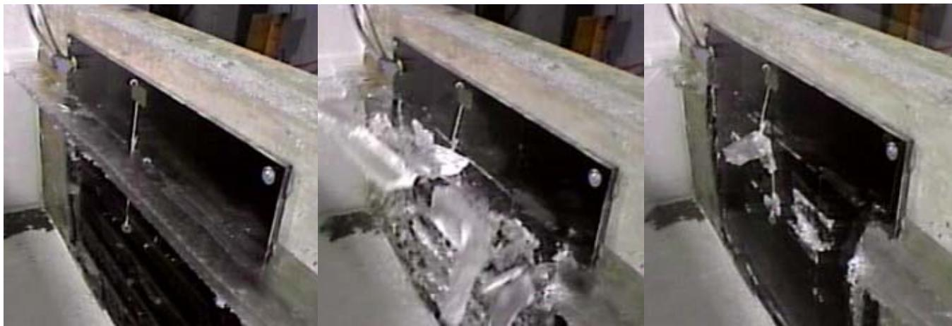
Figure 31. IMS EEDS used for removing ice from a simulated navigation lock wall.
