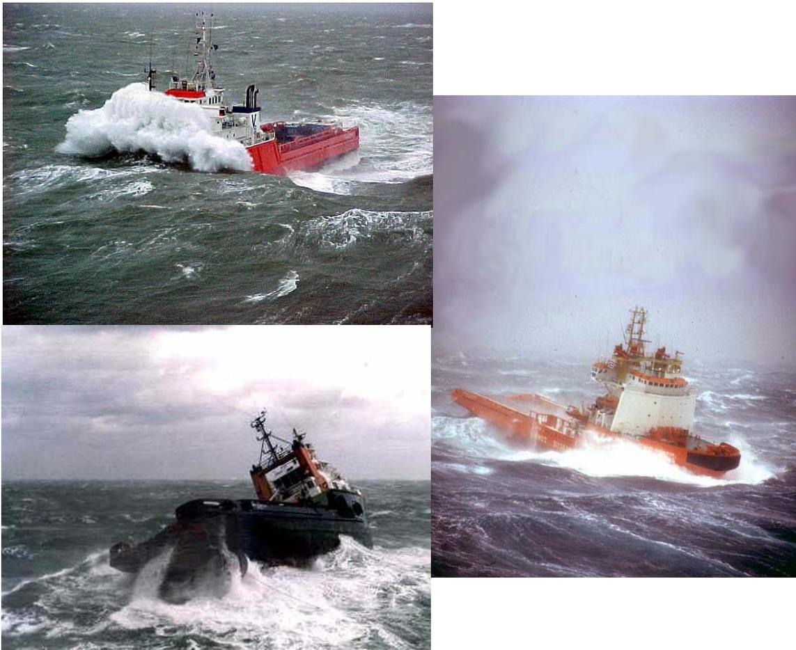
Figure 14. Oil platform supply boats interact actively with the sea, creating abundant spray for superstructure icing (<http://www.qsl.net/kc2jpo/index.html>).
