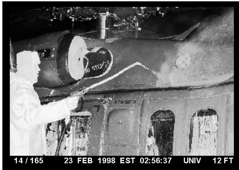
Figure 37. Hot water deicing of Black Hawk helicopter.
