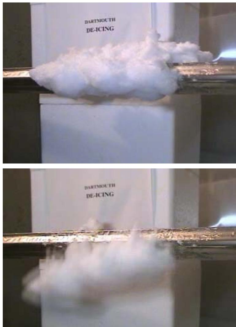
Figure 27. Ice being released from simulated cable by ice dielectric heating method.
