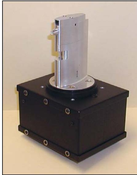
Figure 59. TAMDAR sensor head that senses a variety of atmospheric conditions. Ice sensing is accomplished by light beam interruption in the leading edge notch.
