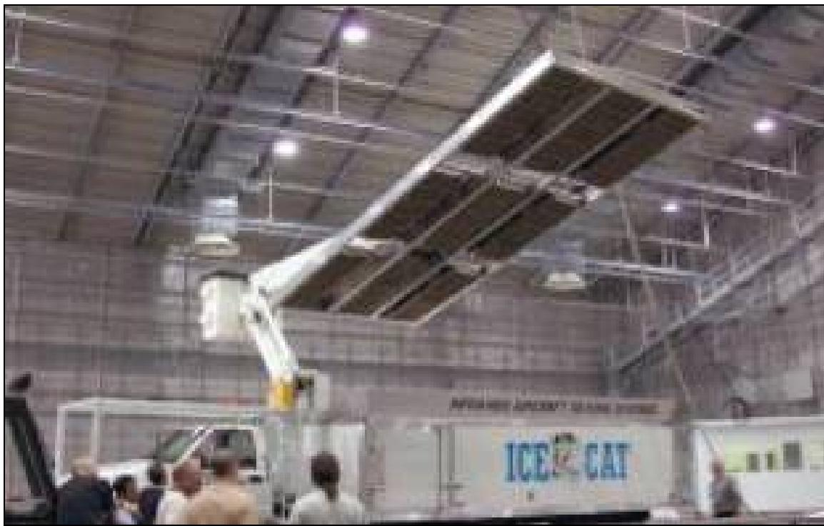
Figure 41. Ice-Cat during testing at Eglin AFB McKinley Climatic Chamber.
