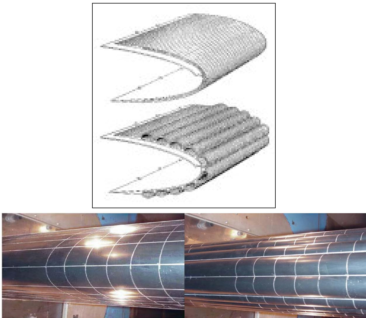
Figure 46. Diagrammatic view (top) of deflated (above) and inflated (below) deicing boot. Bottom: deflated (left) and inflated (right) boots on wing leading edge in wind tunnel.
