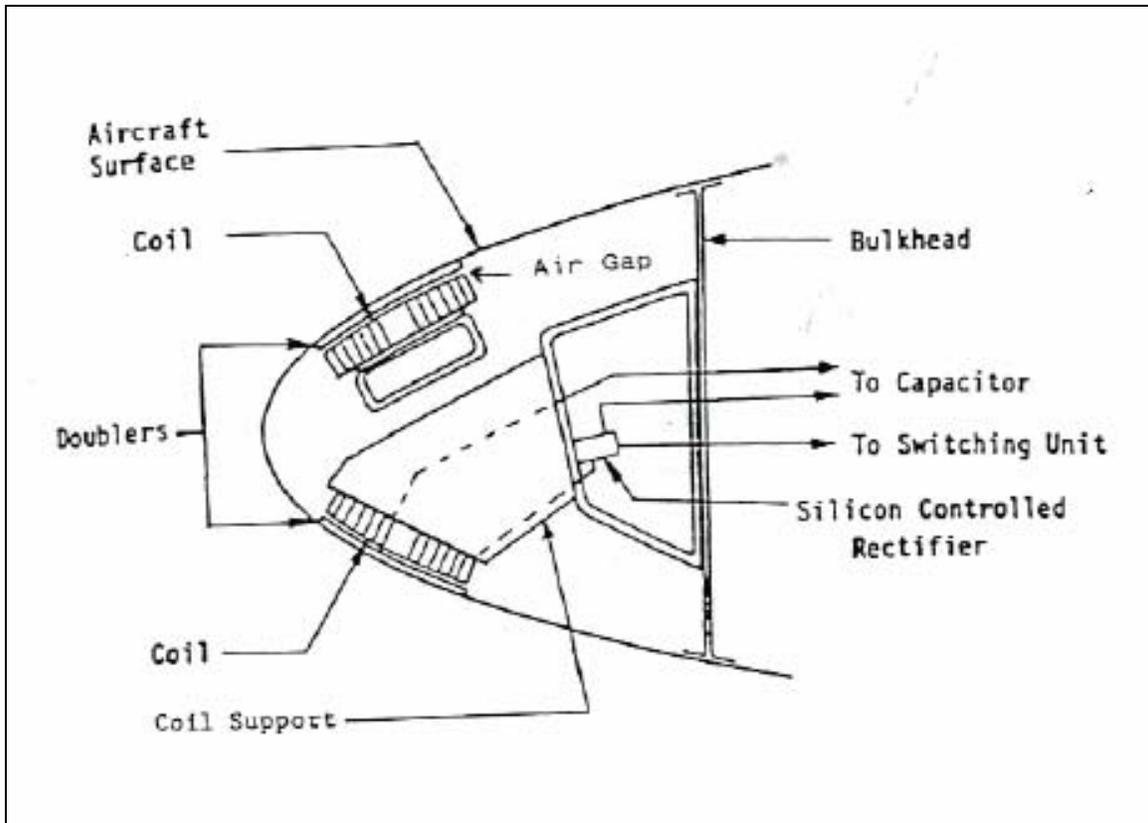
Figure 29. IDI EIDI applied to an airfoil.
