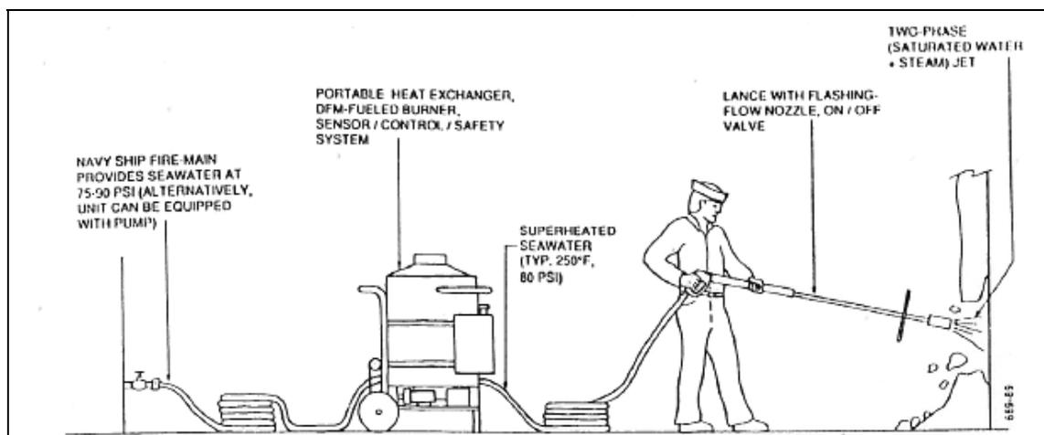
Figure 38. Flash flow portable deicing system for ships.
