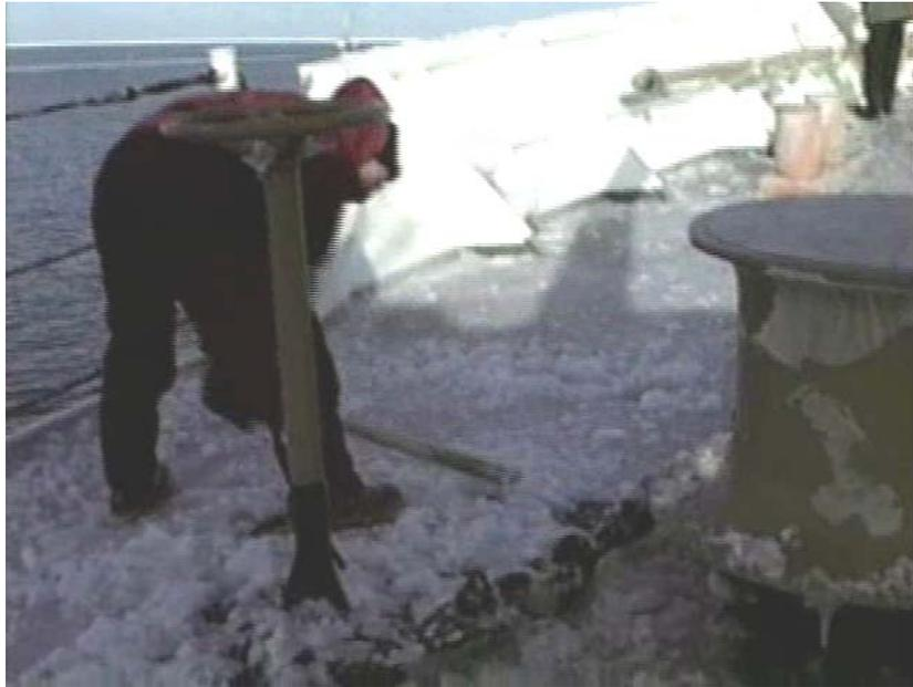
Figure 12. Ice being removed with baseball bat on CGC *Midgett* in Bering Sea.
