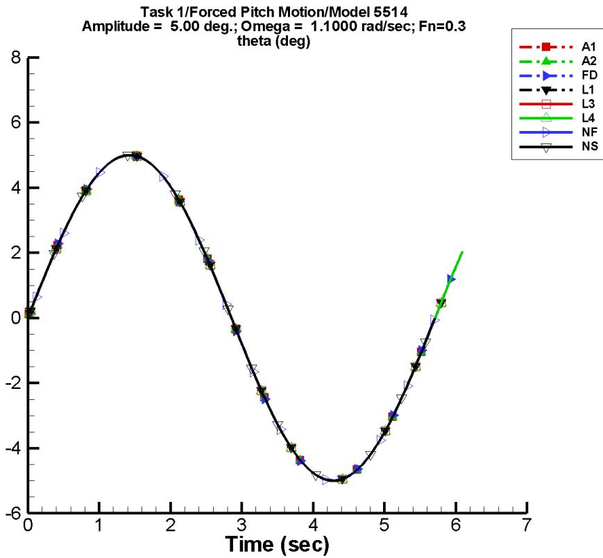
Figure F-30. Time history of  $\theta$  for one period at amplitude = 5.00 deg, frequency = 1.1000 rad/s, Fn = 0.3 in the case of prescribed pitch motion of Model 5514 scaled to L = 142 m.
