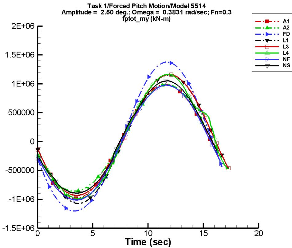
Figure F-113. Time history of  $M_y^{\text{tot}}$  for one period at amplitude = 2.50 deg, frequency = 0.3831 rad/s, Fn = 0.3 in the case of prescribed pitch motion of Model 5514 scaled to L = 142 m.
