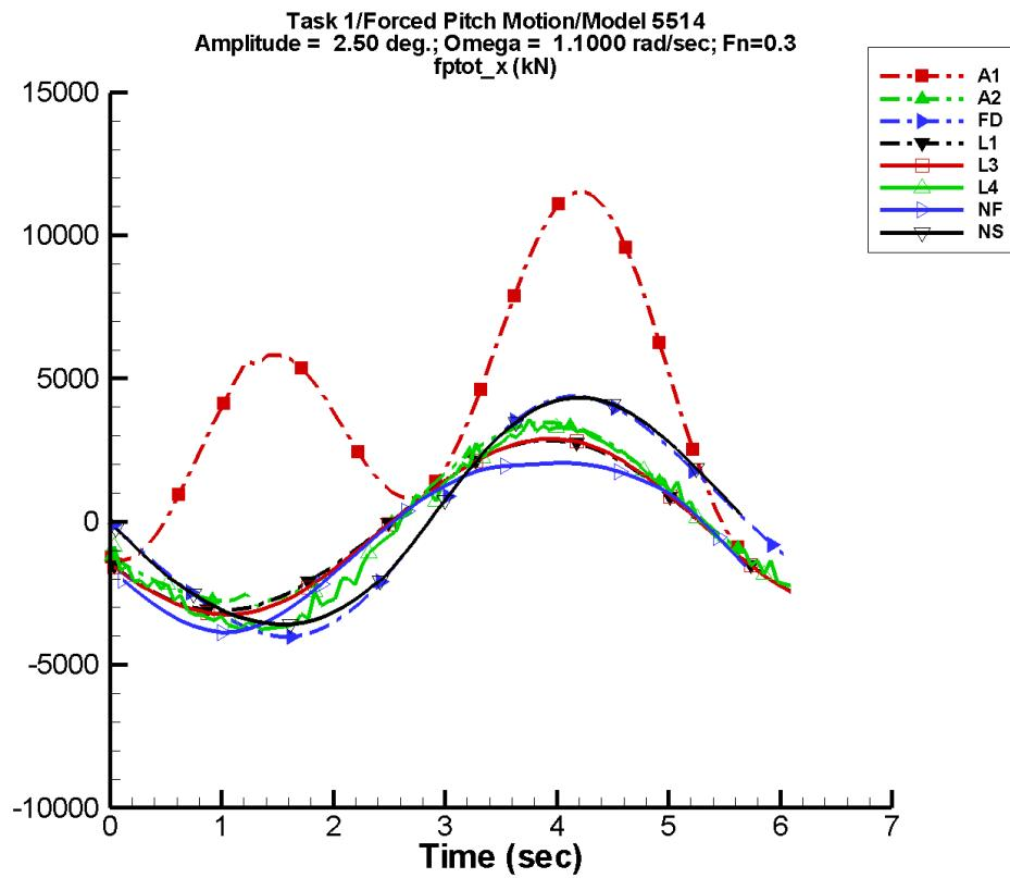
Figure F-58. Time history of  $F_x^{\text{tot}}$  for one period at amplitude = 2.50 deg, frequency = 1.1000 rad/s, Fn = 0.3 in the case of prescribed pitch motion of Model 5514 scaled to L = 142 m.
