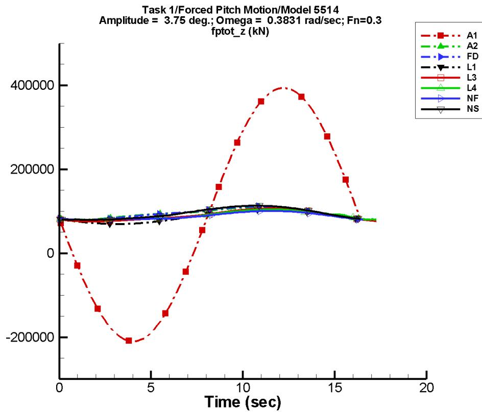
Figure F-84. Time history of  $F_z^{\text{tot}}$  for one period at amplitude = 3.75 deg, frequency = 0.3831 rad/s, Fn = 0.3 in the case of prescribed pitch motion of Model 5514 scaled to L = 142 m.
