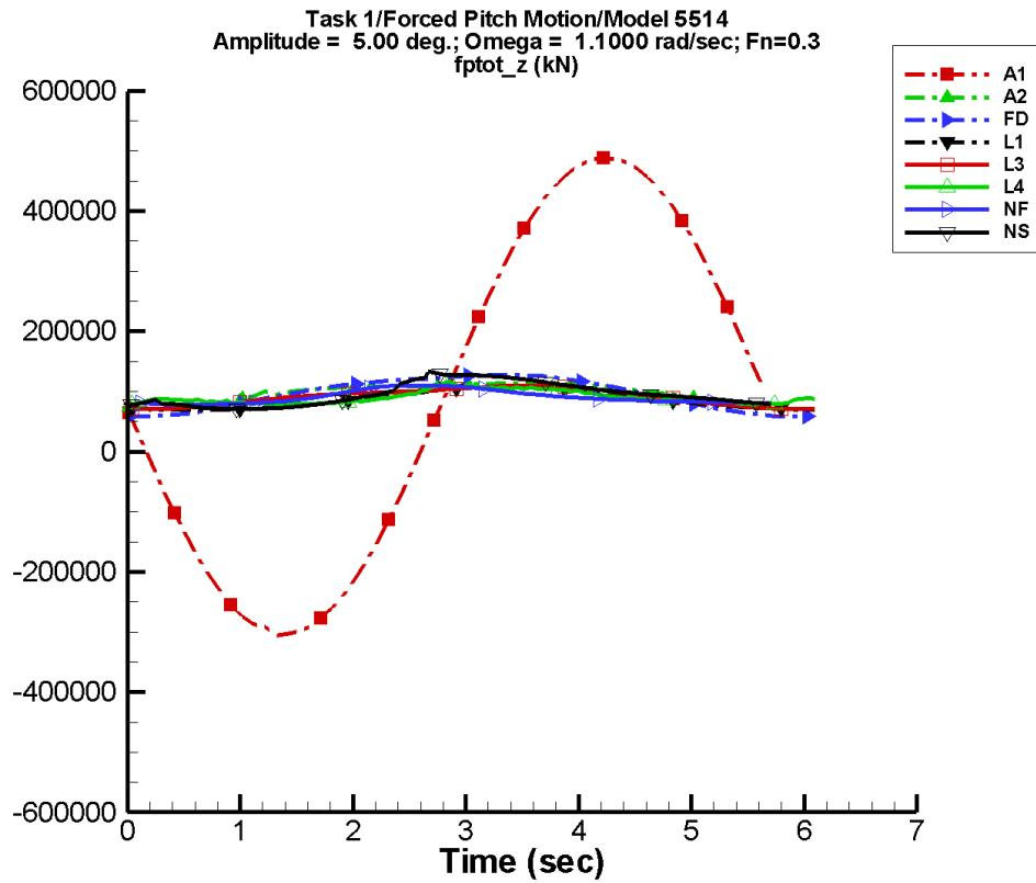
Figure F-90. Time history of  $F_z^{\text{tot}}$  for one period at amplitude = 5.00 deg, frequency = 1.1000 rad/s, Fn = 0.3 in the case of prescribed pitch motion of Model 5514 scaled to L = 142 m.
