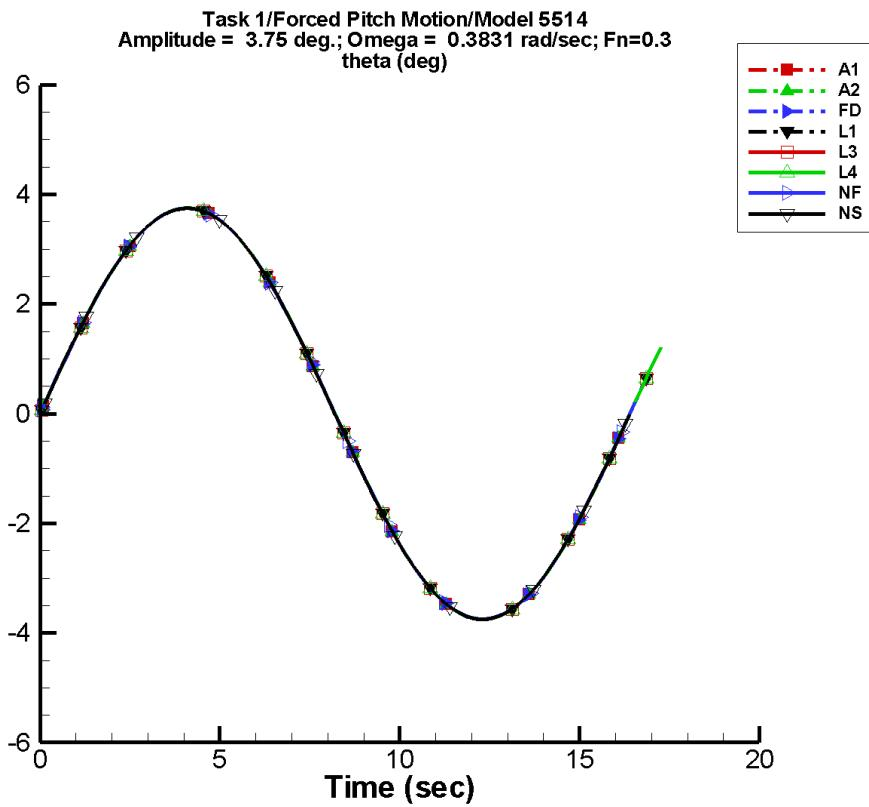
Figure F-24. Time history of  $\theta$  for one period at amplitude = 3.75 deg, frequency = 0.3831 rad/s, Fn = 0.3 in the case of prescribed pitch motion of Model 5514 scaled to L = 142 m.
