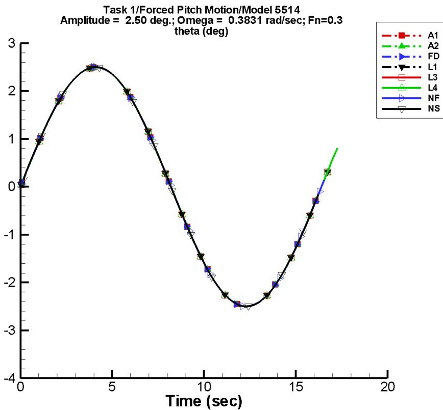
Figure F-23. Time history of  $\theta$  for one period at amplitude = 2.50 deg, frequency = 0.3831 rad/s, Fn = 0.3 in the case of prescribed pitch motion of Model 5514 scaled to L = 142 m.
