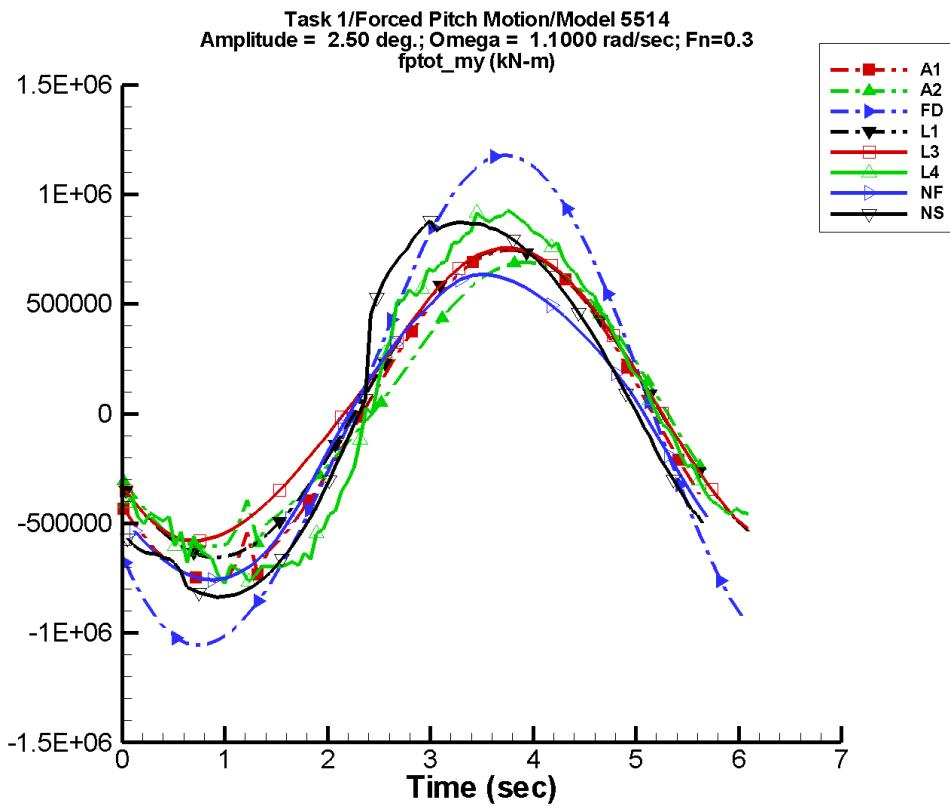
Figure F-118. Time history of  $M_y^{\text{tot}}$  for one period at amplitude = 2.50 deg, frequency = 1.1000 rad/s, Fn = 0.3 in the case of prescribed pitch motion of Model 5514 scaled to L = 142 m.
