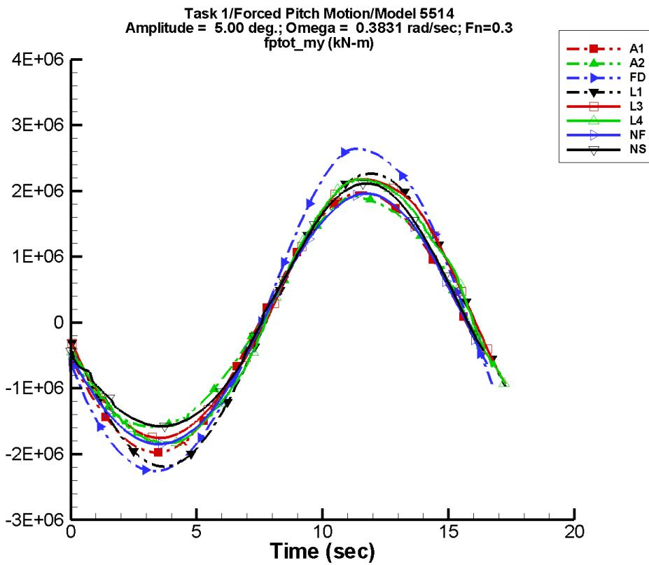
Figure F-115. Time history of  $M_y^{\text{tot}}$  for one period at amplitude = 5.00 deg, frequency = 0.3831 rad/s, Fn = 0.3 in the case of prescribed pitch motion of Model 5514 scaled to L = 142 m.
