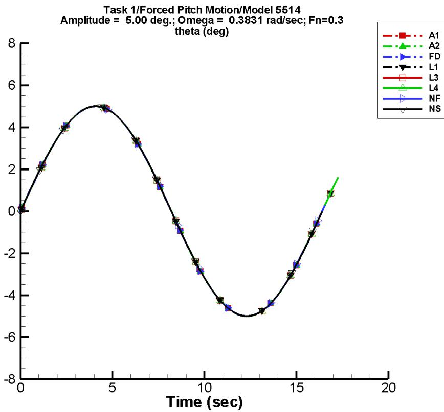
Figure F-25. Time history of  $\theta$  for one period at amplitude = 5.00 deg, frequency = 0.3831 rad/s, Fn = 0.3 in the case of prescribed pitch motion of Model 5514 scaled to L = 142 m.
