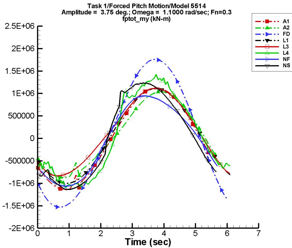
Figure F-119. Time history of  $M_y^{\text{tot}}$  for one period at amplitude = 3.75 deg, frequency = 1.1000 rad/s, Fn = 0.3 in the case of prescribed pitch motion of Model 5514 scaled to L = 142 m.
