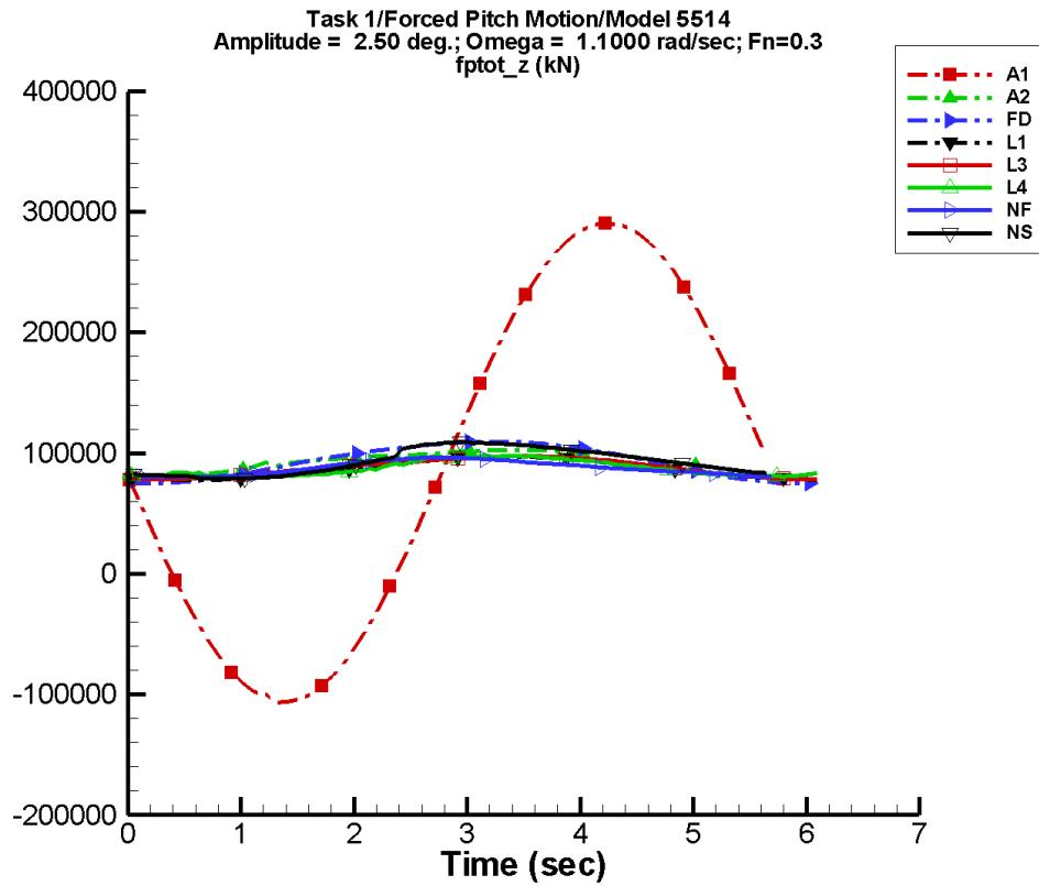
Figure F-88. Time history of  $F_z^{\text{tot}}$  for one period at amplitude = 2.50 deg, frequency = 1.1000 rad/s, Fn = 0.3 in the case of prescribed pitch motion of Model 5514 scaled to L = 142 m.
