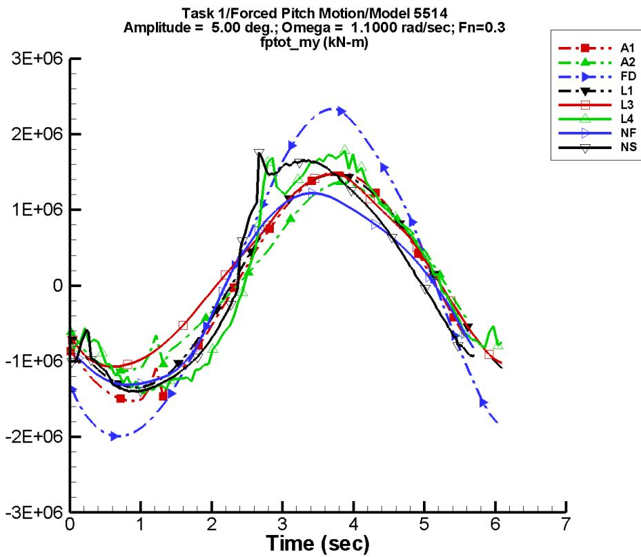
Figure F-120. Time history of  $M_y^{\text{tot}}$  for one period at amplitude = 5.00 deg, frequency = 1.1000 rad/s, Fn = 0.3 in the case of prescribed pitch motion of Model 5514 scaled to L = 142 m.
