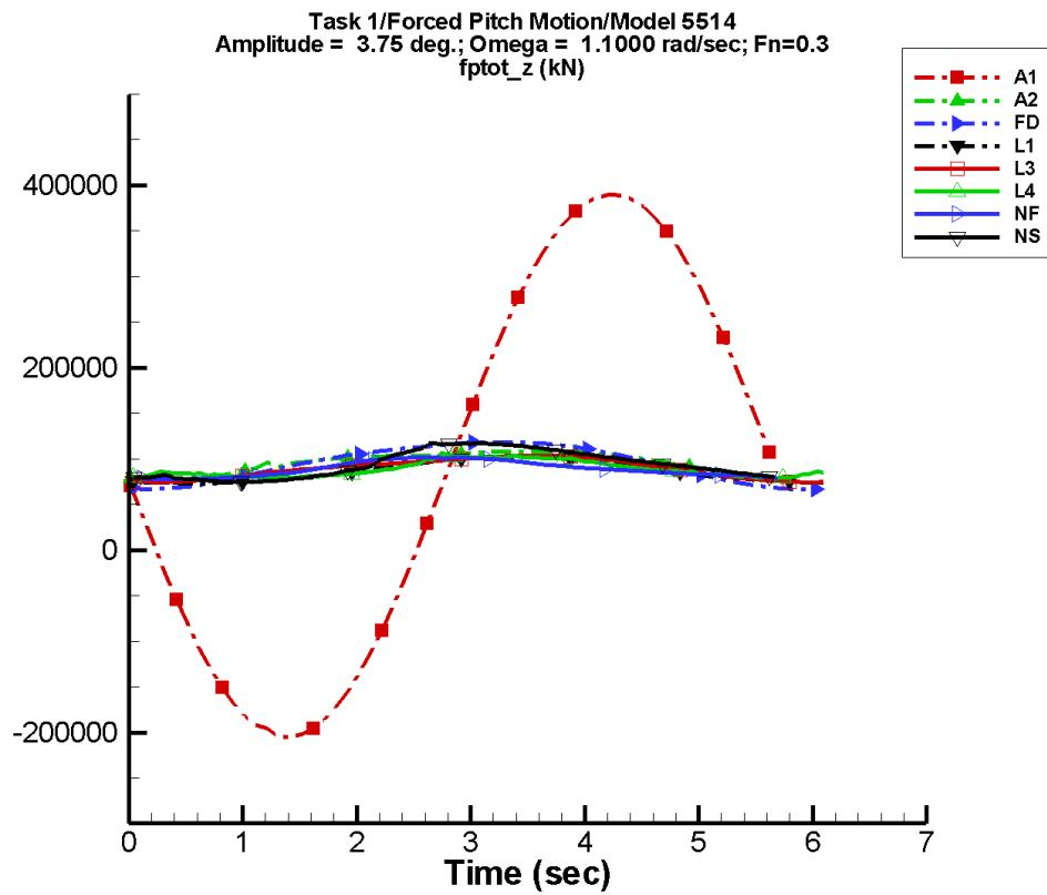
Figure F-89. Time history of  $F_z^{\text{tot}}$  for one period at amplitude = 3.75 deg, frequency = 1.1000 rad/s, Fn = 0.3 in the case of prescribed pitch motion of Model 5514 scaled to L = 142 m.
