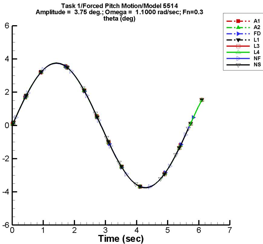
Figure F-29. Time history of  $\theta$  for one period at amplitude = 3.75 deg, frequency = 1.1000 rad/s, Fn = 0.3 in the case of prescribed pitch motion of Model 5514 scaled to L = 142 m.
