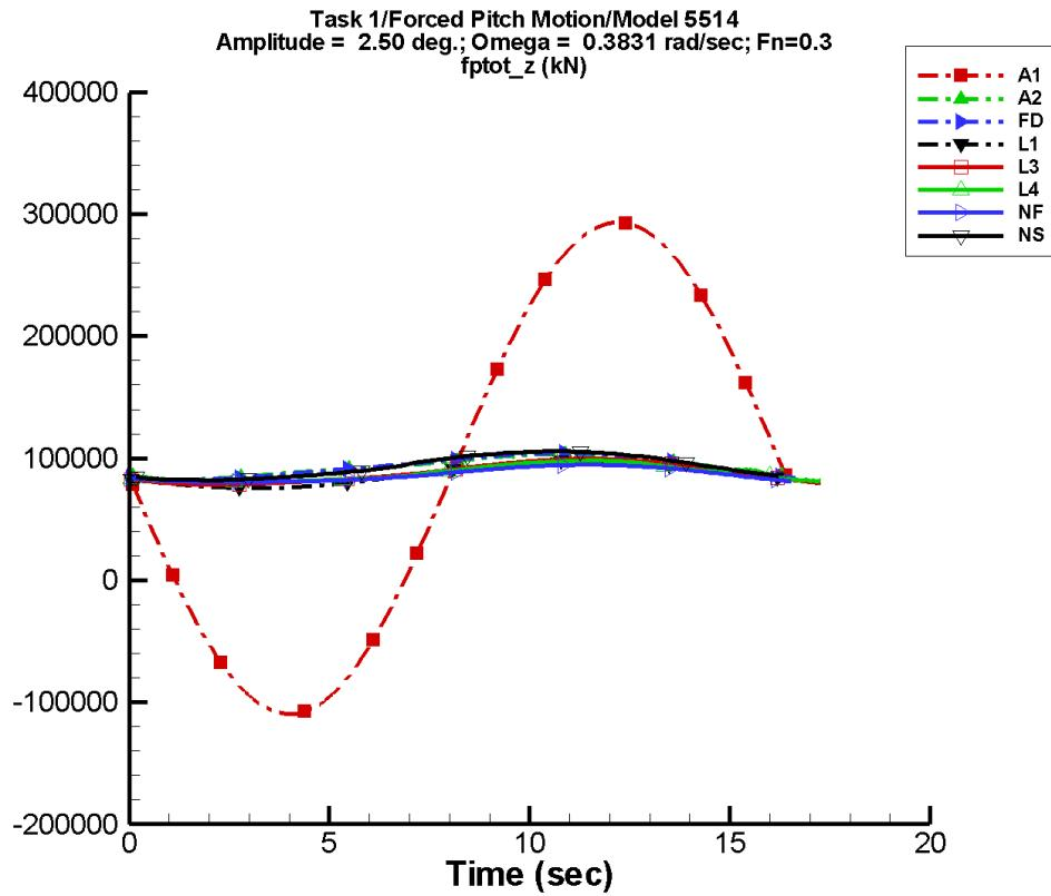
Figure F-83. Time history of  $F_z^{\text{tot}}$  for one period at amplitude = 2.50 deg, frequency = 0.3831 rad/s, Fn = 0.3 in the case of prescribed pitch motion of Model 5514 scaled to L = 142 m.
