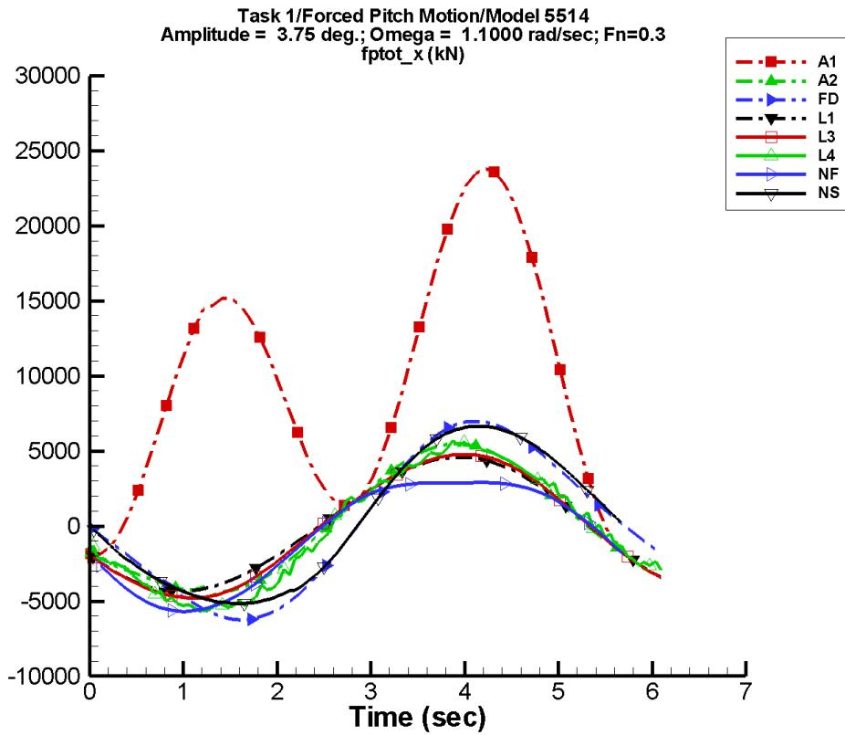
Figure F-59. Time history of  $F_x^{\text{tot}}$  for one period at amplitude = 3.75 deg, frequency = 1.1000 rad/s, Fn = 0.3 in the case of prescribed pitch motion of Model 5514 scaled to L = 142 m.
