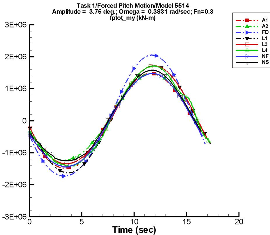
Figure F-114. Time history of  $M_y^{\text{tot}}$  for one period at amplitude = 3.75 deg, frequency = 0.3831 rad/s, Fn = 0.3 in the case of prescribed pitch motion of Model 5514 scaled to L = 142 m.
