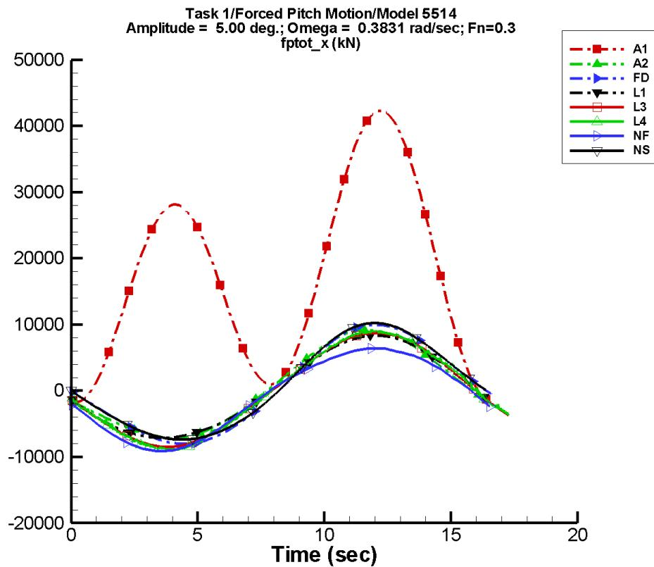
Figure F-55. Time history of  $F_x^{\text{tot}}$  for one period at amplitude = 5.00 deg, frequency = 0.3831 rad/s, Fn = 0.3 in the case of prescribed pitch motion of Model 5514 scaled to L = 142 m.
