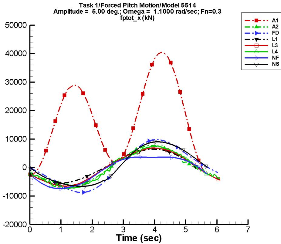
Figure F-60. Time history of  $F_x^{\text{tot}}$  for one period at amplitude = 5.00 deg, frequency = 1.1000 rad/s, Fn = 0.3 in the case of prescribed pitch motion of Model 5514 scaled to L = 142 m.
