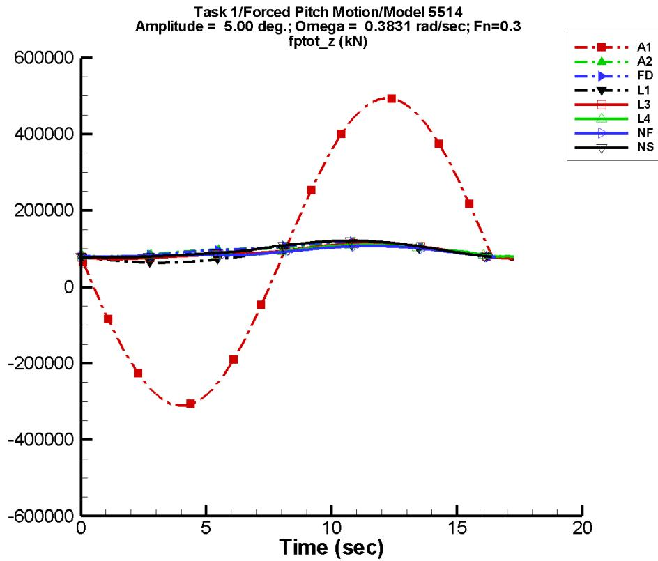
Figure F-85. Time history of  $F_z^{\text{tot}}$  for one period at amplitude = 5.00 deg, frequency = 0.3831 rad/s, Fn = 0.3 in the case of prescribed pitch motion of Model 5514 scaled to L = 142 m.
