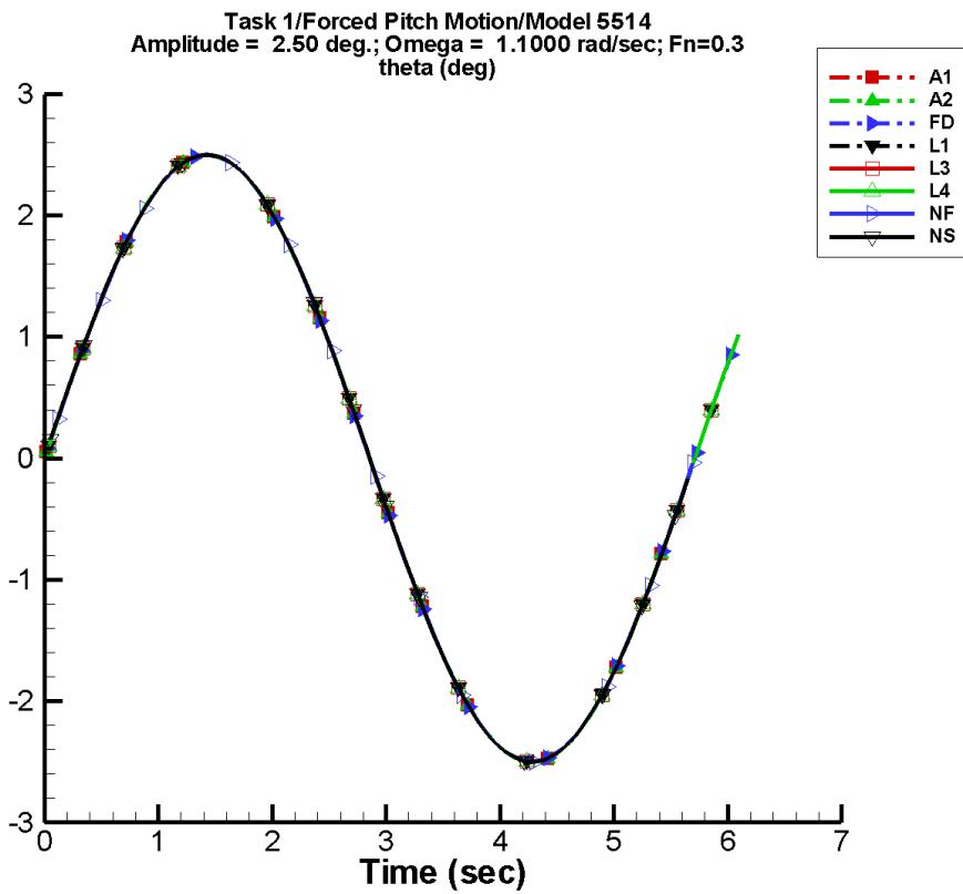
Figure F-28. Time history of  $\theta$  for one period at amplitude = 2.50 deg, frequency = 1.1000 rad/s, Fn = 0.3 in the case of prescribed pitch motion of Model 5514 scaled to L = 142 m.
