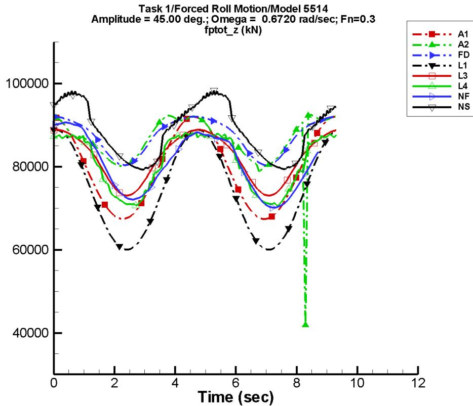
Figure D-119. Time history of  $F_z^{\text{tot}}$  for one period at amplitude = 45.00 deg, frequency = 0.6720 rad/s, Fn = 0.3 in the case of prescribed roll motion of Model 5514 scaled to L = 142 m.
