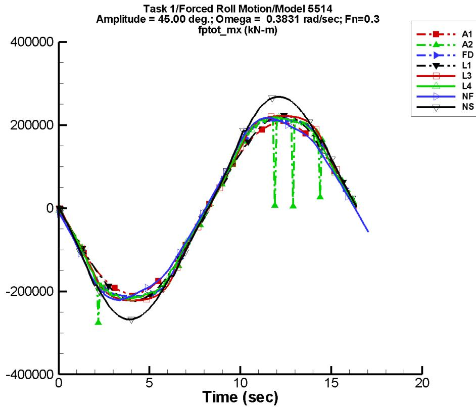
Figure D-144. Time history of  $M_x^{\text{tot}}$  for one period at amplitude = 45.00 deg, frequency = 0.3831 rad/s, Fn = 0.3 in the case of prescribed roll motion of Model 5514 scaled to L = 142 m.
