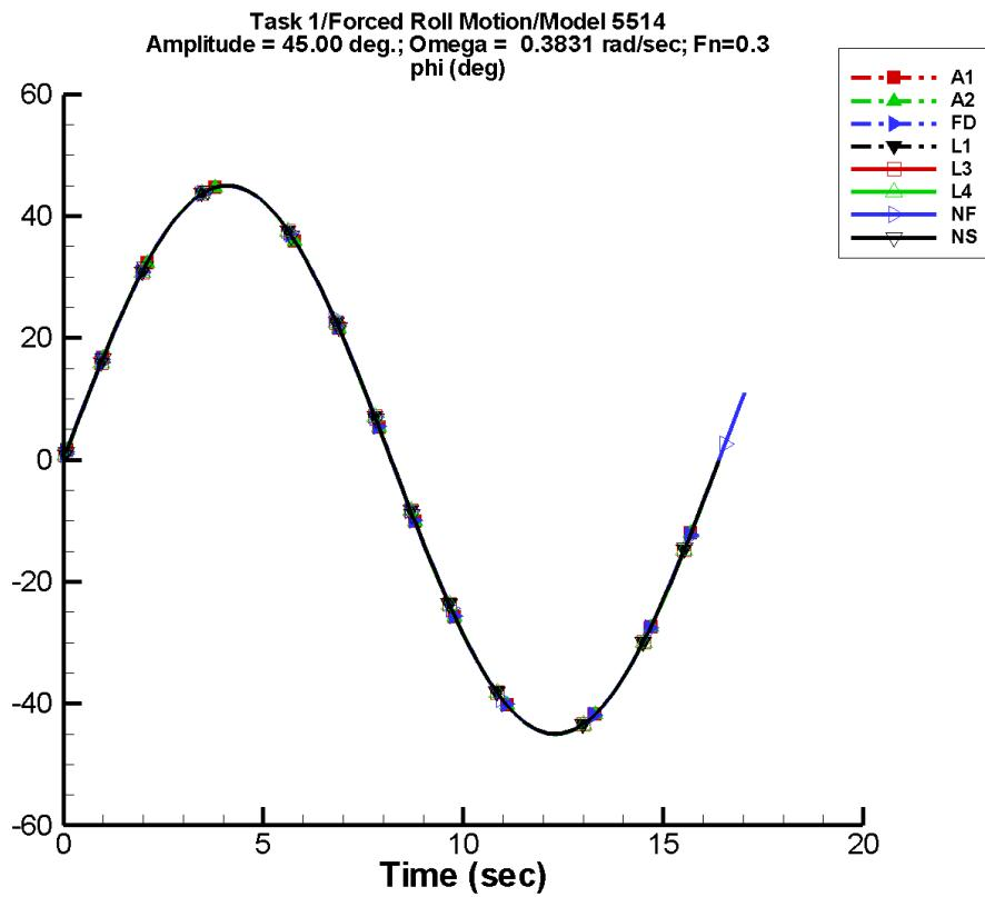
Figure D-24. Time history of  $\phi$  for one period at amplitude = 45.00 deg, frequency = 0.3831 rad/s, Fn = 0.3 in the case of prescribed roll motion of Model 5514 scaled to L = 142 m.
