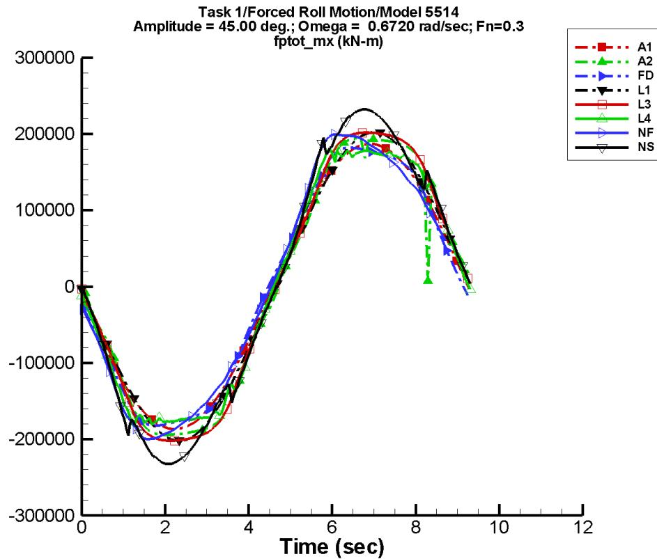
Figure D-149. Time history of  $M_x^{\text{tot}}$  for one period at amplitude = 45.00 deg, frequency = 0.6720 rad/s, Fn = 0.3 in the case of prescribed roll motion of Model 5514 scaled to L = 142 m.
