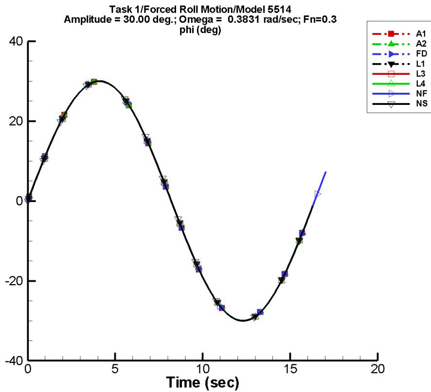
Figure D-23. Time history of  $\phi$  for one period at amplitude = 30.00 deg, frequency = 0.3831 rad/s, Fn = 0.3 in the case of prescribed roll motion of Model 5514 scaled to L = 142 m.
