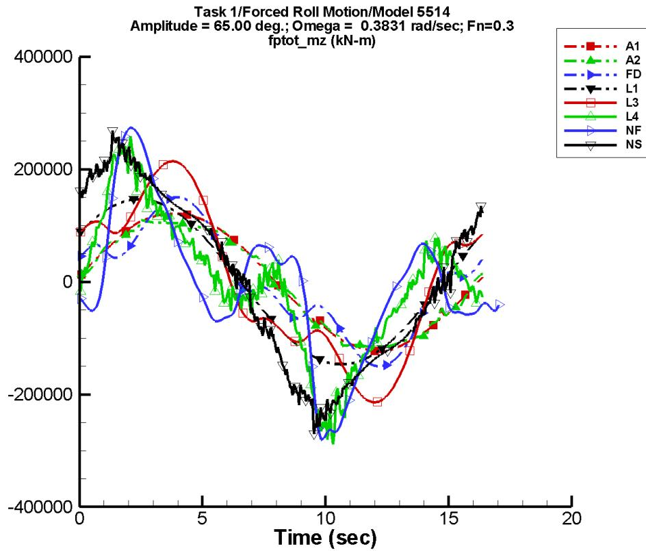
Figure D-205. Time history of  $M_z^{\text{tot}}$  for one period at amplitude = 65.00 deg, frequency = 0.3831 rad/s, Fn = 0.3 in the case of prescribed roll motion of Model 5514 scaled to L = 142 m.
