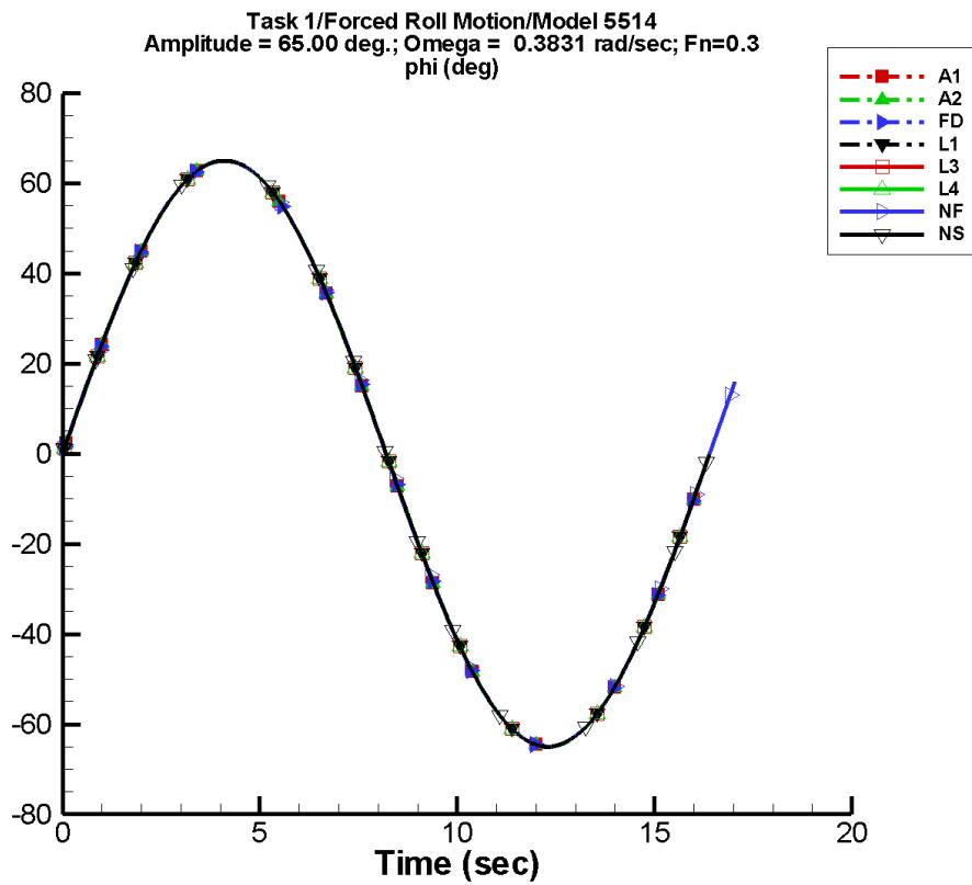
Figure D-25. Time history of  $\phi$  for one period at amplitude = 65.00 deg, frequency = 0.3831 rad/s, Fn = 0.3 in the case of prescribed roll motion of Model 5514 scaled to L = 142 m.
