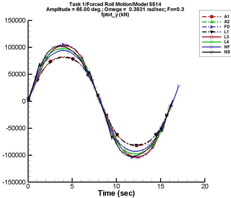
Figure D-85. Time history of  $F_y^{\text{tot}}$  for one period at amplitude = 65.00 deg, frequency = 0.3831 rad/s, Fn = 0.3 in the case of prescribed roll motion of Model 5514 scaled to L = 142 m.
