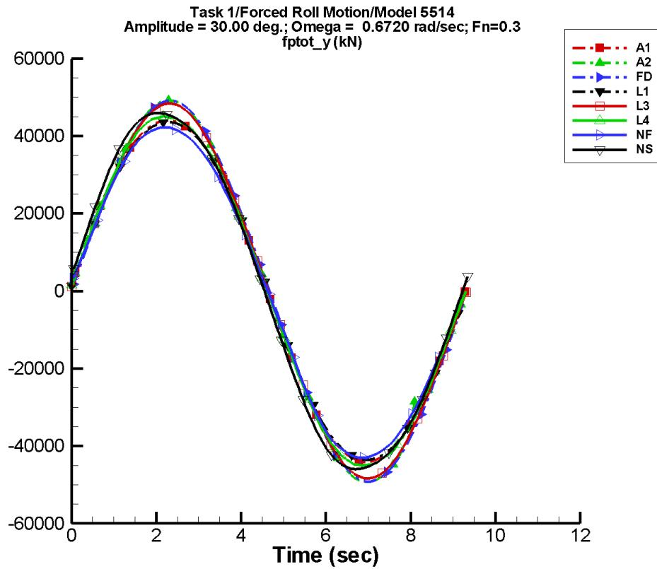
Figure D-88. Time history of  $F_y^{\text{tot}}$  for one period at amplitude = 30.00 deg, frequency = 0.6720 rad/s, Fn = 0.3 in the case of prescribed roll motion of Model 5514 scaled to L = 142 m.
