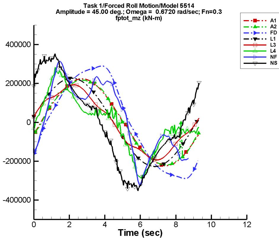
Figure D-209. Time history of  $M_z^{\text{tot}}$  for one period at amplitude = 45.00 deg, frequency = 0.6720 rad/s, Fn = 0.3 in the case of prescribed roll motion of Model 5514 scaled to L = 142 m.
