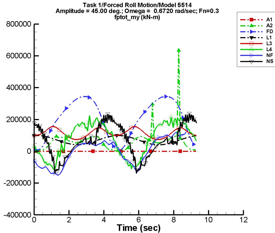
Figure D-179. Time history of  $M_y^{\text{tot}}$  for one period at amplitude = 45.00 deg, frequency = 0.6720 rad/s, Fn = 0.3 in the case of prescribed roll motion of Model 5514 scaled to L = 142 m.
