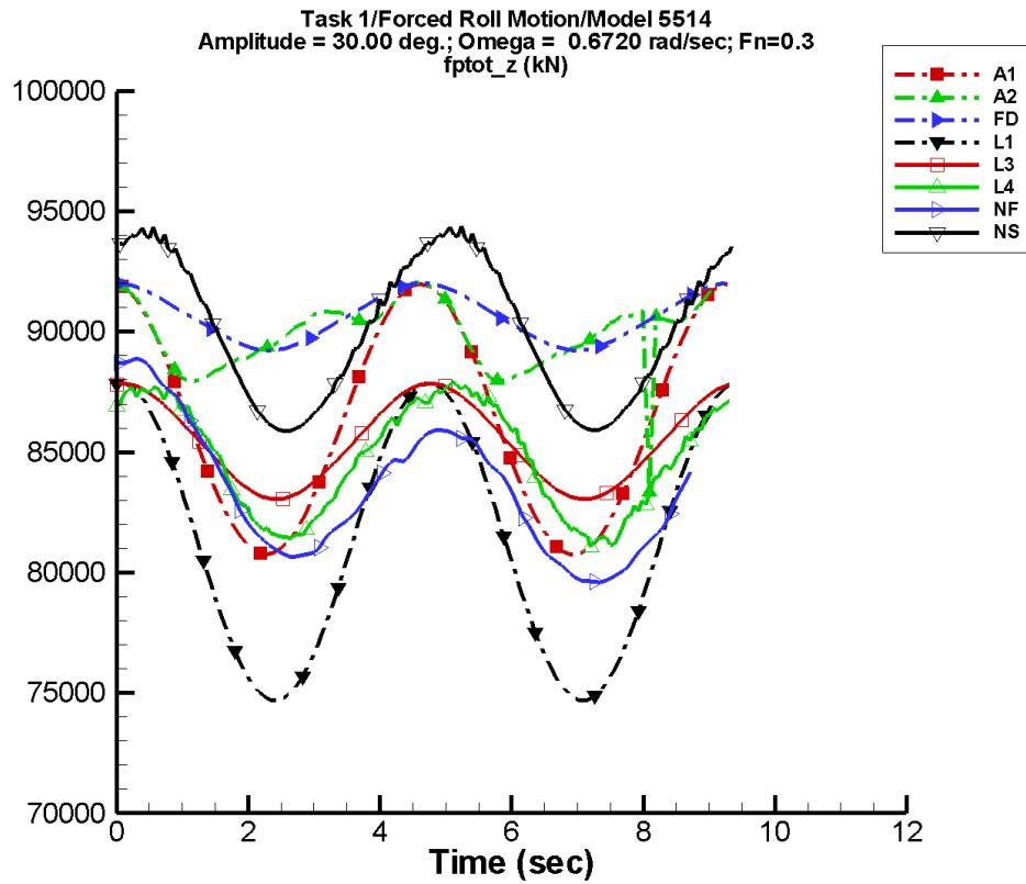
Figure D-118. Time history of  $F_z^{\text{tot}}$  for one period at amplitude = 30.00 deg, frequency = 0.6720 rad/s, Fn = 0.3 in the case of prescribed roll motion of Model 5514 scaled to L = 142 m.
