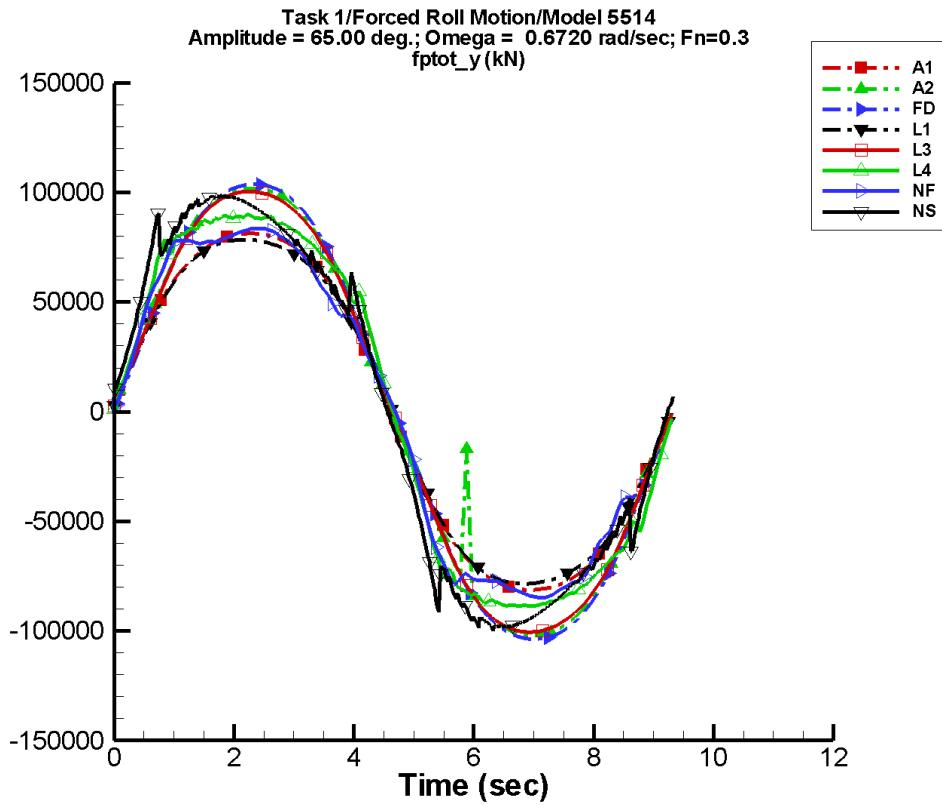
Figure D-90. Time history of  $F_y^{\text{tot}}$  for one period at amplitude = 65.00 deg, frequency = 0.6720 rad/s, Fn = 0.3 in the case of prescribed roll motion of Model 5514 scaled to L = 142 m.
