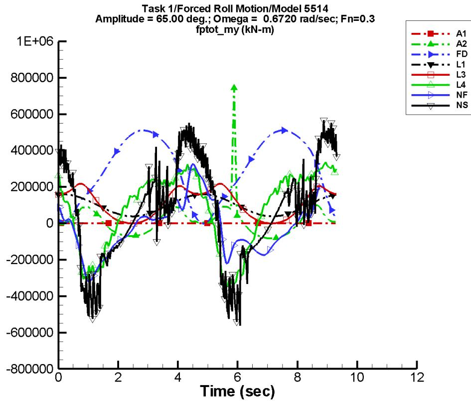
Figure D-180. Time history of  $M_y^{\text{tot}}$  for one period at amplitude = 65.00 deg, frequency = 0.6720 rad/s, Fn = 0.3 in the case of prescribed roll motion of Model 5514 scaled to L = 142 m.
