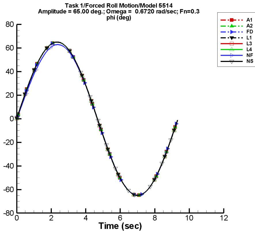
Figure D-30. Time history of  $\phi$  for one period at amplitude = 65.00 deg, frequency = 0.6720 rad/s, Fn = 0.3 in the case of prescribed roll motion of Model 5514 scaled to L = 142 m.
