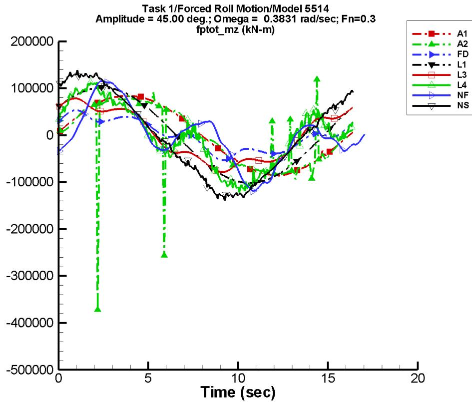
Figure D-204. Time history of  $M_z^{\text{tot}}$  for one period at amplitude = 45.00 deg, frequency = 0.3831 rad/s, Fn = 0.3 in the case of prescribed roll motion of Model 5514 scaled to L = 142 m.
