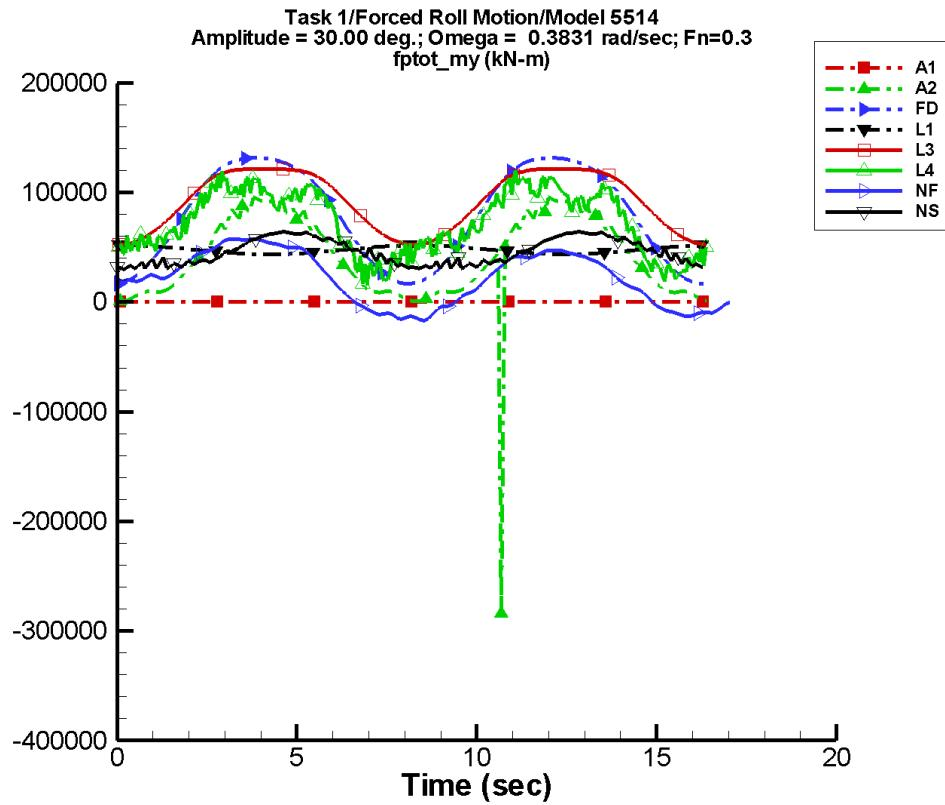
Figure D-173. Time history of  $M_y^{\text{tot}}$  for one period at amplitude = 30.00 deg, frequency = 0.3831 rad/s, Fn = 0.3 in the case of prescribed roll motion of Model 5514 scaled to L = 142 m.
