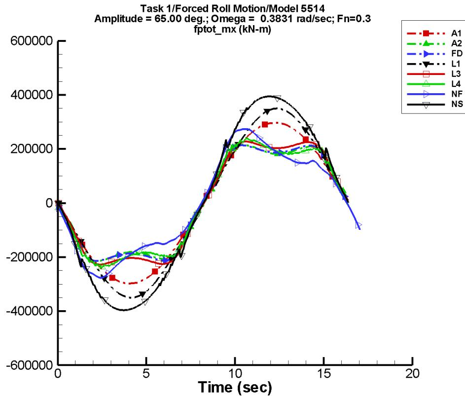
Figure D-145. Time history of  $M_x^{\text{tot}}$  for one period at amplitude = 65.00 deg, frequency = 0.3831 rad/s, Fn = 0.3 in the case of prescribed roll motion of Model 5514 scaled to L = 142 m.
