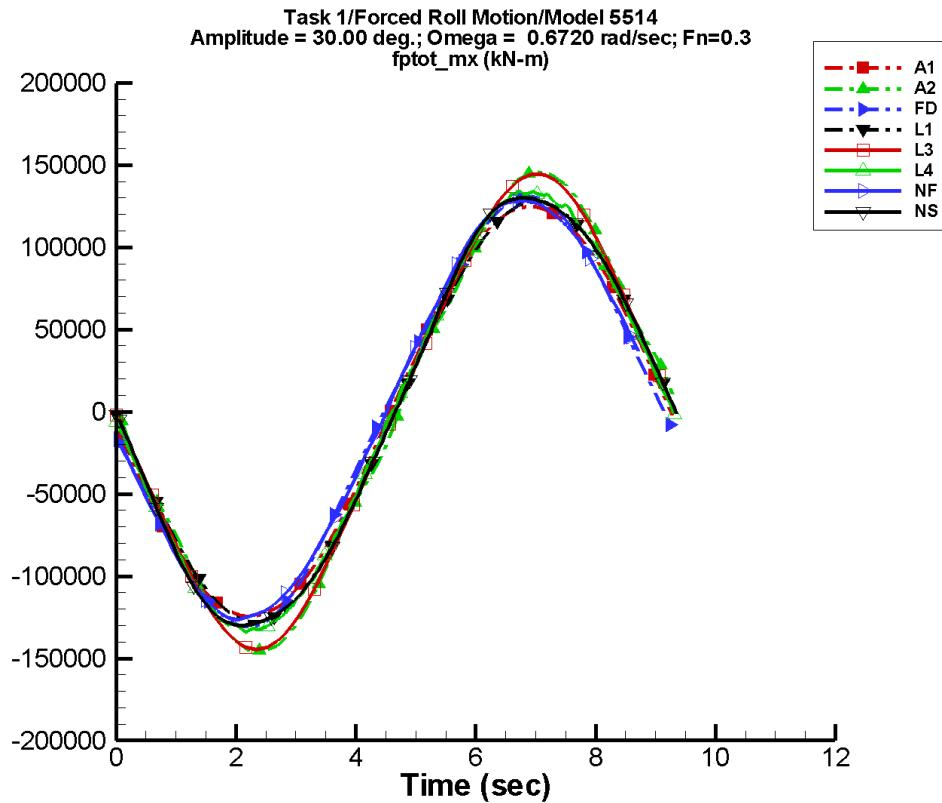
Figure D-148. Time history of  $M_x^{\text{tot}}$  for one period at amplitude = 30.00 deg, frequency = 0.6720 rad/s, Fn = 0.3 in the case of prescribed roll motion of Model 5514 scaled to L = 142 m.
