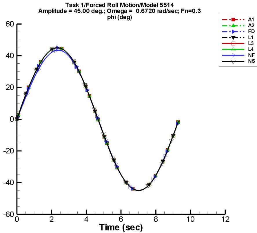
Figure D-29. Time history of  $\phi$  for one period at amplitude = 45.00 deg, frequency = 0.6720 rad/s, Fn = 0.3 in the case of prescribed roll motion of Model 5514 scaled to L = 142 m.
