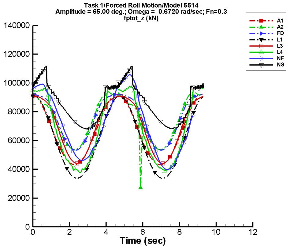
Figure D-120. Time history of  $F_z^{\text{tot}}$  for one period at amplitude = 65.00 deg, frequency = 0.6720 rad/s, Fn = 0.3 in the case of prescribed roll motion of Model 5514 scaled to L = 142 m.
