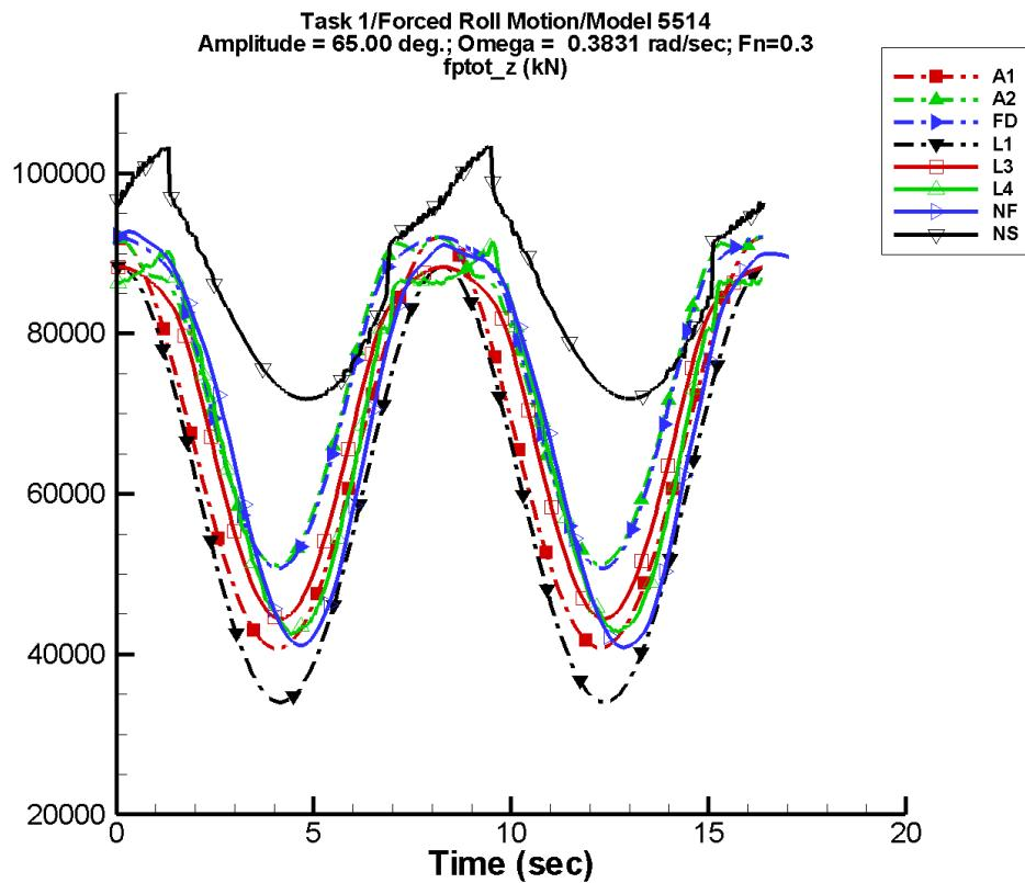
Figure D-115. Time history of  $F_z^{\text{tot}}$  for one period at amplitude = 65.00 deg, frequency = 0.3831 rad/s, Fn = 0.3 in the case of prescribed roll motion of Model 5514 scaled to L = 142 m.
