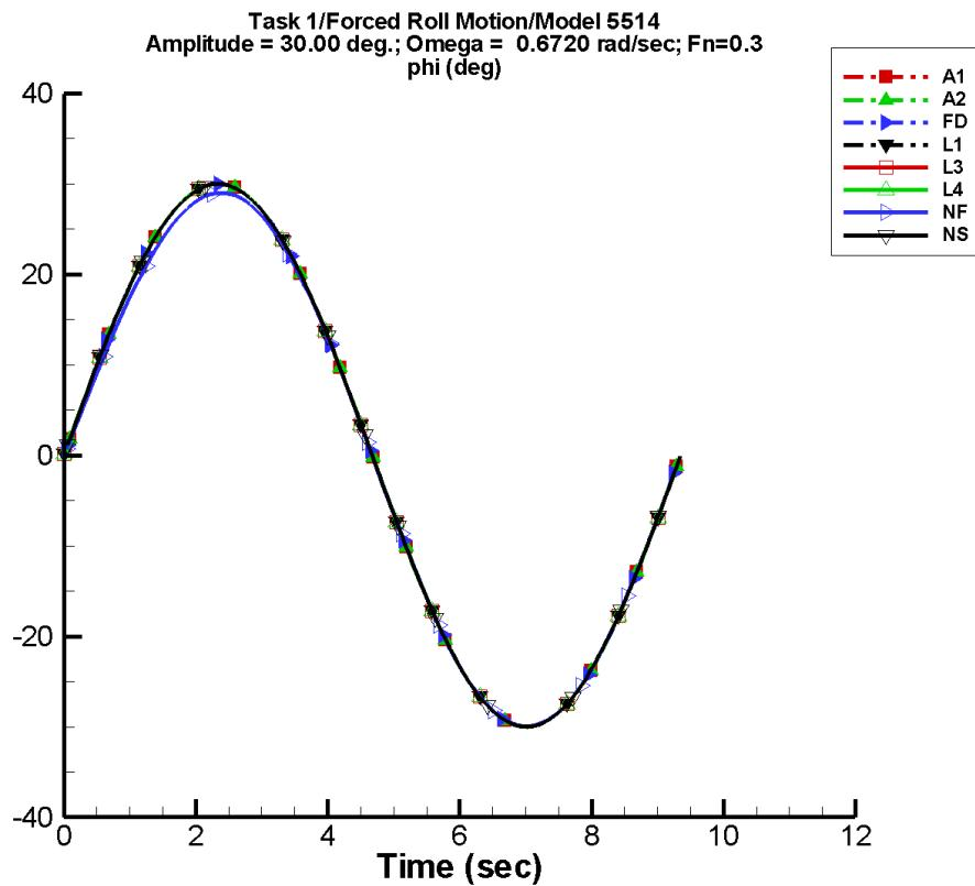
Figure D-28. Time history of  $\phi$  for one period at amplitude = 30.00 deg, frequency = 0.6720 rad/s, Fn = 0.3 in the case of prescribed roll motion of Model 5514 scaled to L = 142 m.
