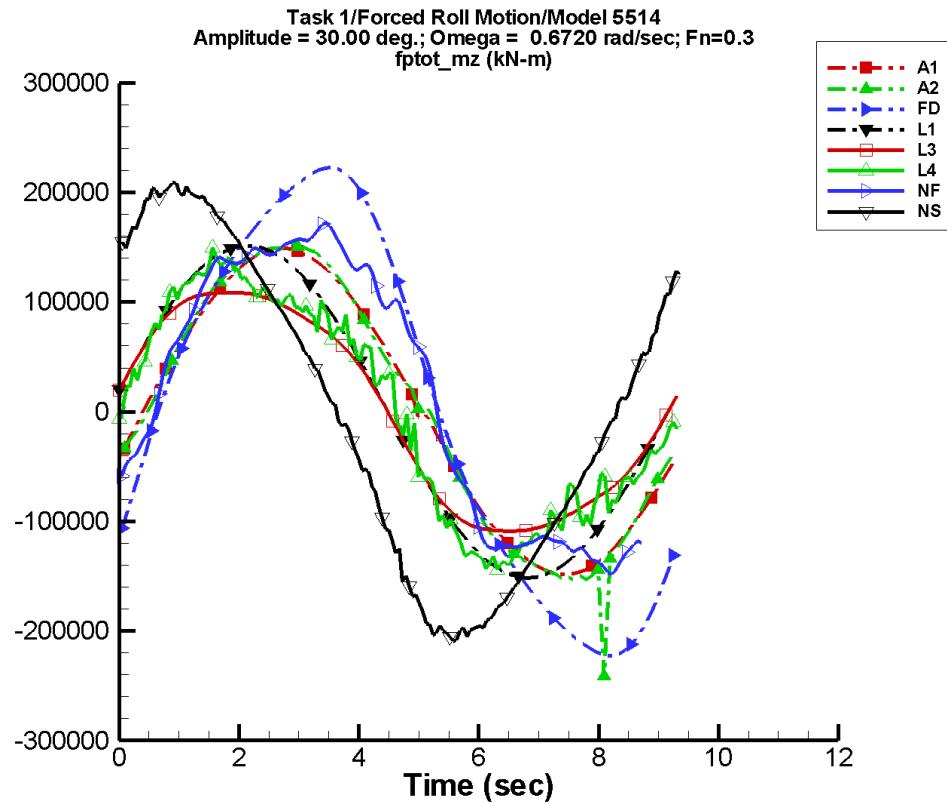
Figure D-208. Time history of  $M_z^{\text{tot}}$  for one period at amplitude = 30.00 deg, frequency = 0.6720 rad/s, Fn = 0.3 in the case of prescribed roll motion of Model 5514 scaled to L = 142 m.
