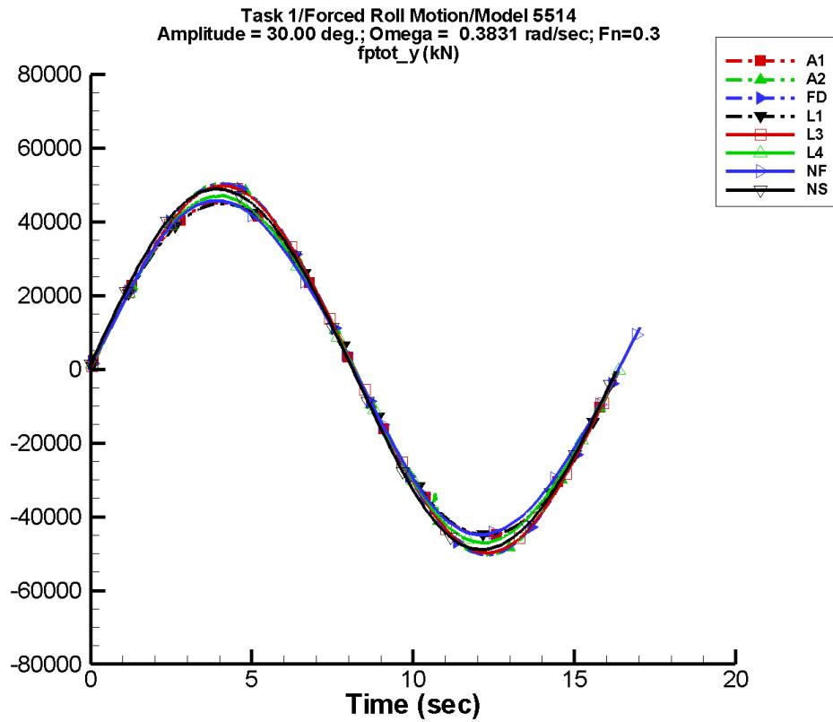
Figure D-83. Time history of  $F_y^{\text{tot}}$  for one period at amplitude = 30.00 deg, frequency = 0.3831 rad/s, Fn = 0.3 in the case of prescribed roll motion of Model 5514 scaled to L = 142 m.
