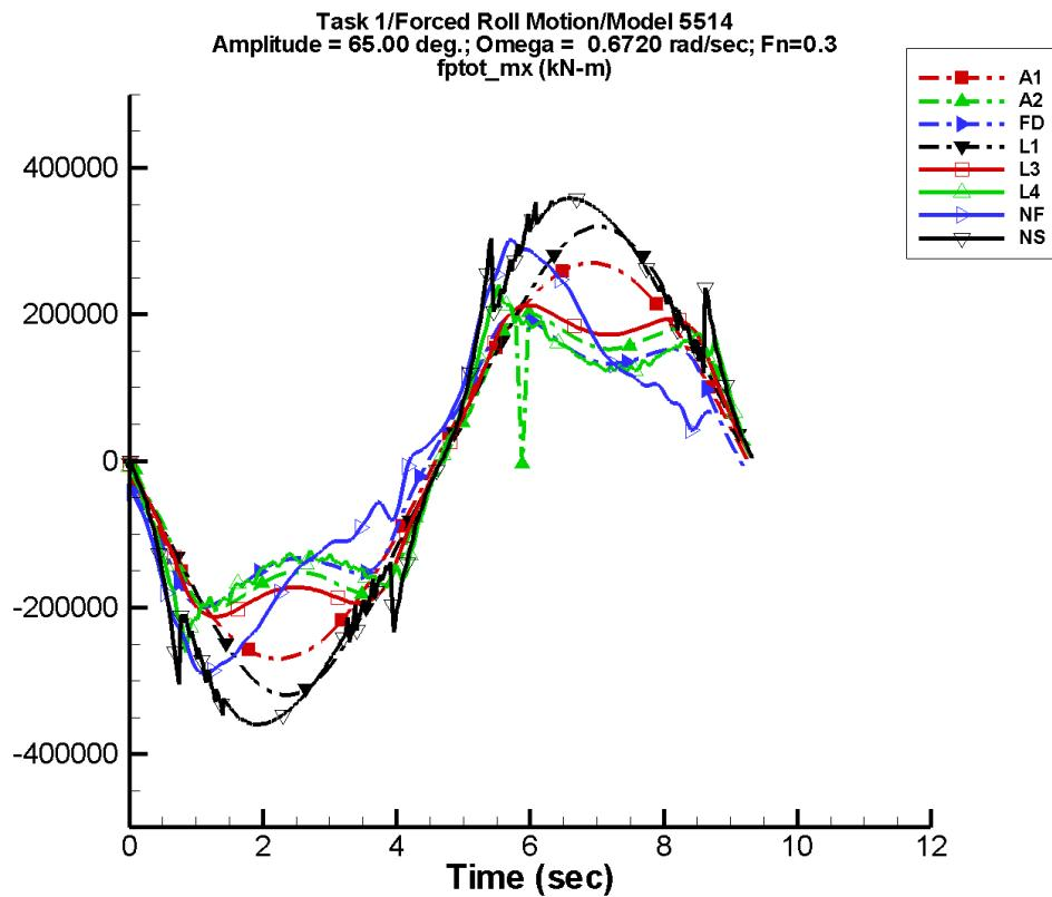
Figure D-150. Time history of  $M_x^{\text{ptot}}$  for one period at amplitude = 65.00 deg, frequency = 0.6720 rad/s, Fn = 0.3 in the case of prescribed roll motion of Model 5514 scaled to L = 142 m.
