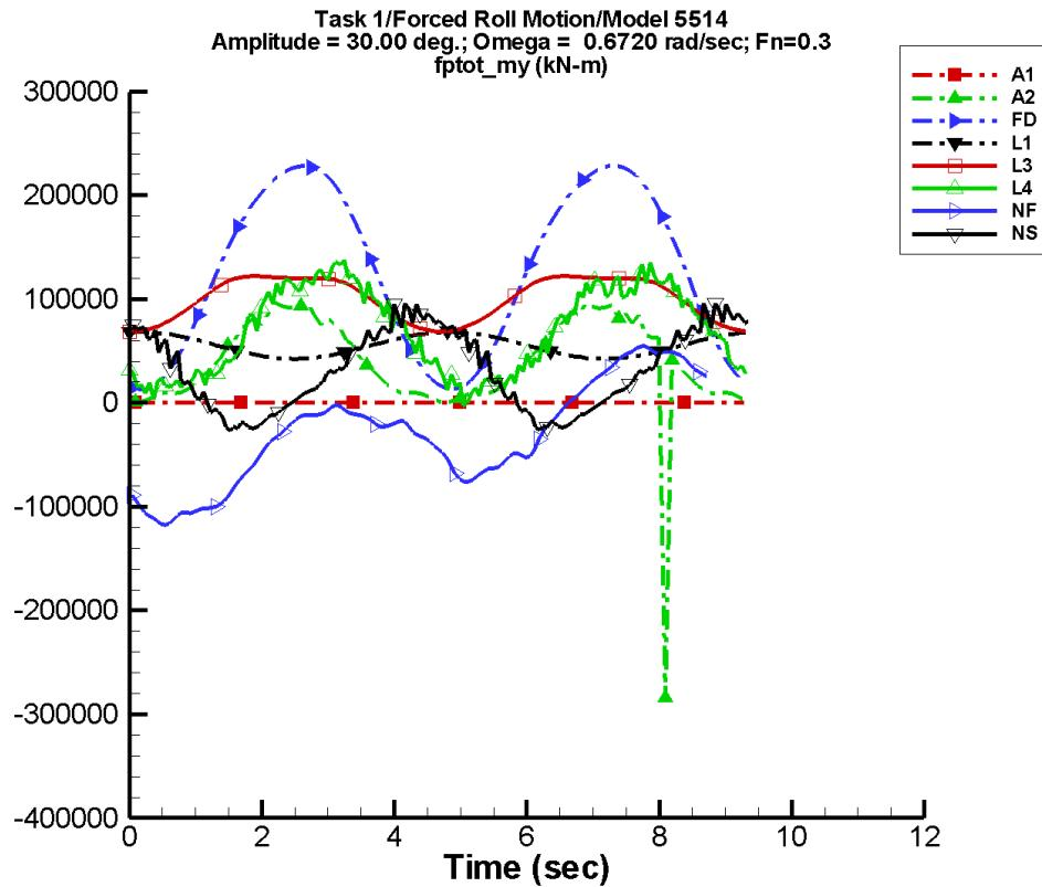
Figure D-178. Time history of  $M_y^{\text{tot}}$  for one period at amplitude = 30.00 deg, frequency = 0.6720 rad/s, Fn = 0.3 in the case of prescribed roll motion of Model 5514 scaled to L = 142 m.
