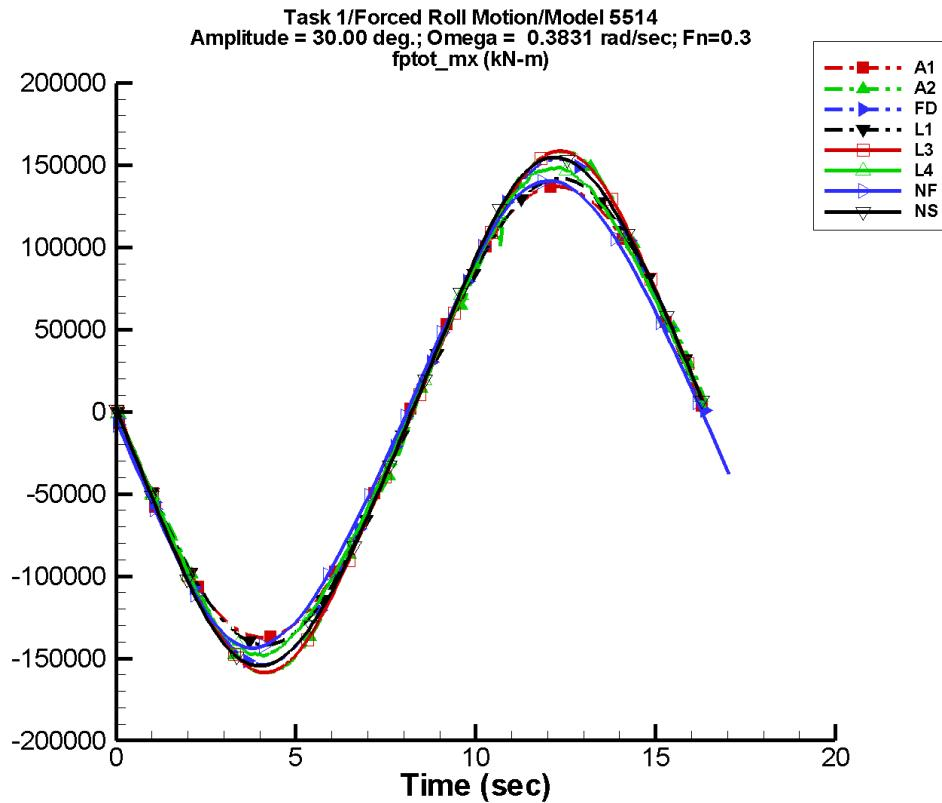
Figure D-143. Time history of  $M_x^{\text{tot}}$  for one period at amplitude = 30.00 deg, frequency = 0.3831 rad/s, Fn = 0.3 in the case of prescribed roll motion of Model 5514 scaled to L = 142 m.
