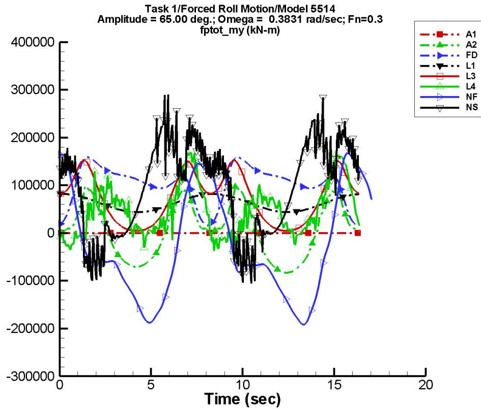
Figure D-175. Time history of  $M_y^{\text{tot}}$  for one period at amplitude = 65.00 deg, frequency = 0.3831 rad/s, Fn = 0.3 in the case of prescribed roll motion of Model 5514 scaled to L = 142 m.
