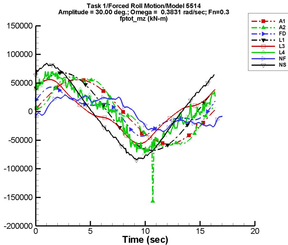
Figure D-203. Time history of  $M_z^{\text{tot}}$  for one period at amplitude = 30.00 deg, frequency = 0.3831 rad/s, Fn = 0.3 in the case of prescribed roll motion of Model 5514 scaled to L = 142 m.
