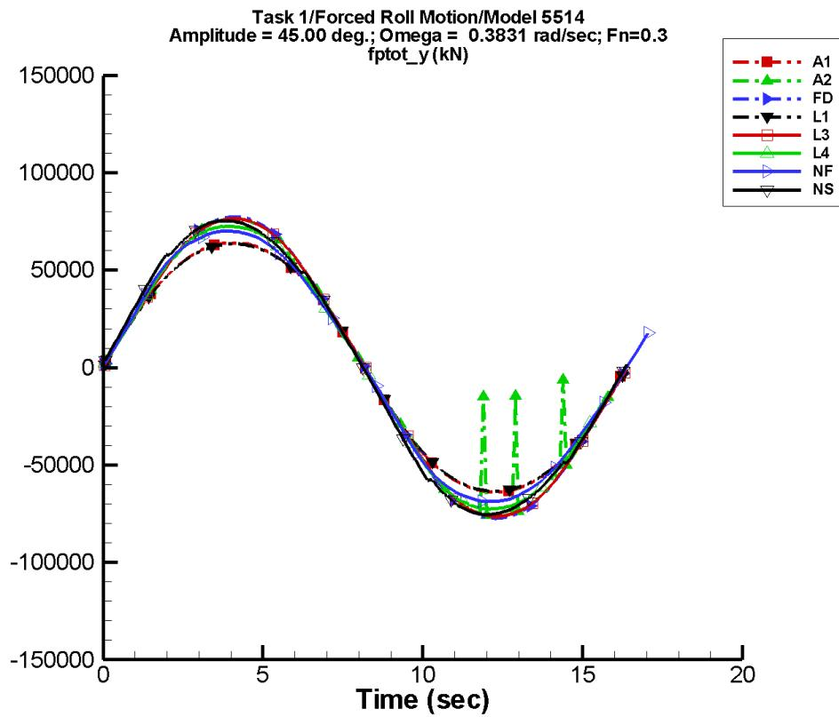
Figure D-84. Time history of  $F_y^{\text{tot}}$  for one period at amplitude = 45.00 deg, frequency = 0.3831 rad/s, Fn = 0.3 in the case of prescribed roll motion of Model 5514 scaled to L = 142 m.
