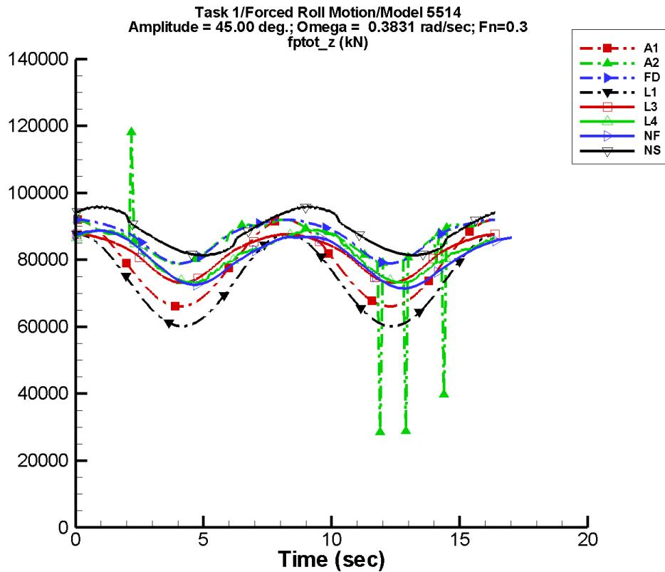
Figure D-114. Time history of  $F_z^{\text{tot}}$  for one period at amplitude = 45.00 deg, frequency = 0.3831 rad/s, Fn = 0.3 in the case of prescribed roll motion of Model 5514 scaled to L = 142 m.
