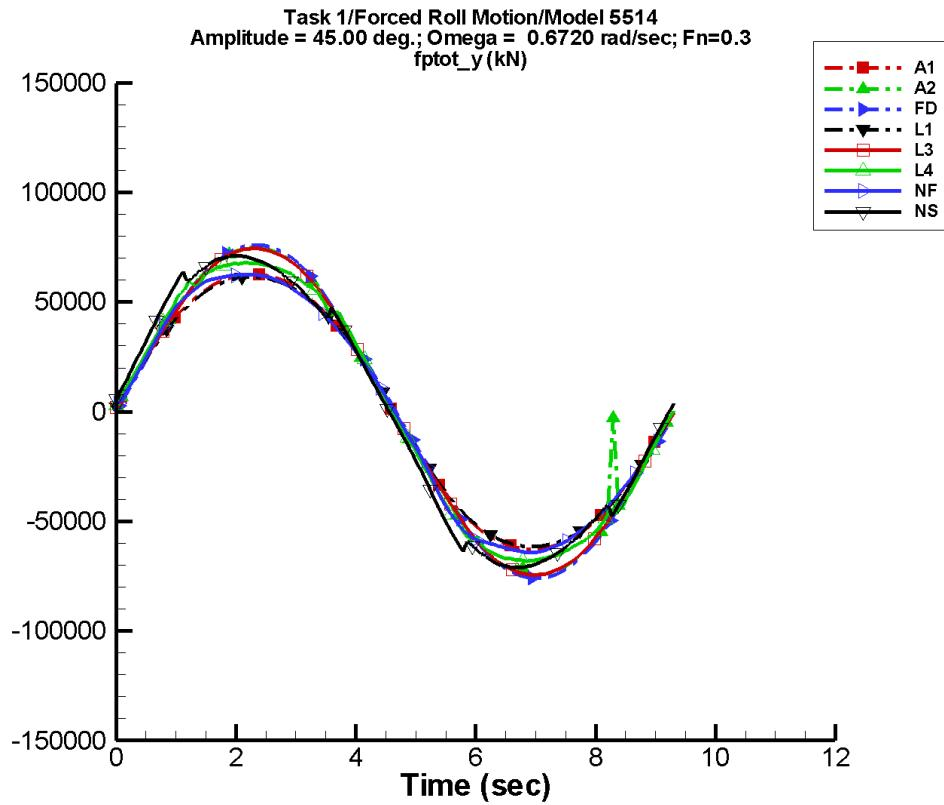
Figure D-89. Time history of  $F_y^{\text{tot}}$  for one period at amplitude = 45.00 deg, frequency = 0.6720 rad/s, Fn = 0.3 in the case of prescribed roll motion of Model 5514 scaled to L = 142 m.
