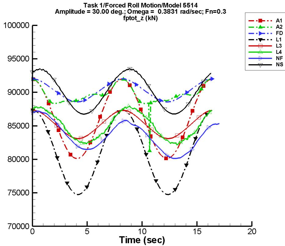
Figure D-113. Time history of  $F_z^{\text{tot}}$  for one period at amplitude = 30.00 deg, frequency = 0.3831 rad/s, Fn = 0.3 in the case of prescribed roll motion of Model 5514 scaled to L = 142 m.
