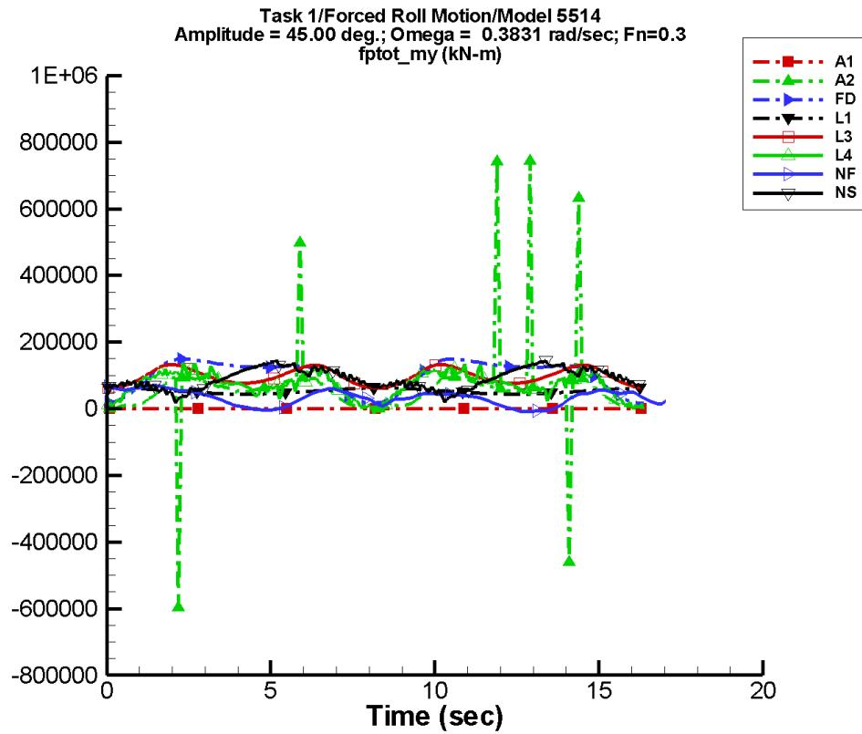
Figure D-174. Time history of  $M_y^{\text{tot}}$  for one period at amplitude = 45.00 deg, frequency = 0.3831 rad/s, Fn = 0.3 in the case of prescribed roll motion of Model 5514 scaled to L = 142 m.
