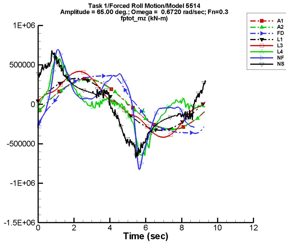
Figure D-210. Time history of  $M_z^{\text{tot}}$  for one period at amplitude = 65.00 deg, frequency = 0.6720 rad/s, Fn = 0.3 in the case of prescribed roll motion of Model 5514 scaled to L = 142 m.
