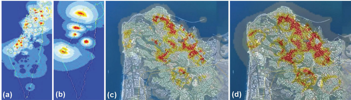
Figure 1. Examples of threat forecasts are shown, with threat likelihood coded by color, ranging from blue for lowest threat to red for highest threat. (a) Several high-level threats appear in this example. (b) Feature reduction of (a), achieved by aggregating geospatial information layers, provides a more manageable forecast for security resource allocation. (c) Map overlay of subregion hot spots. (d) Threat levels are more widely distributed when historical-event position uncertainties are incorporated in (c).
