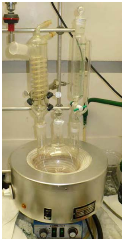
Figure 7. The setup for the synthesis of the citrate-capped AuNP solution. The heating mantle is placed on top of a magnetic stirrer, and a 1L flask is fitted with a distillation column and filter.
