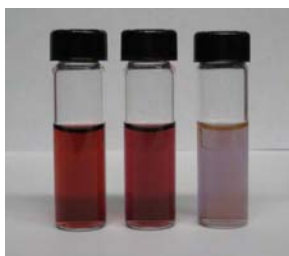
Figure 14. Colloidal AuNP synthesized using molar ratios of 4:1 (left), 3:1 (center) and 1:1 (right)
