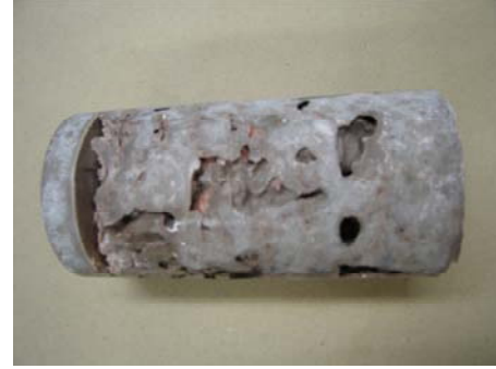
(b) Cylinder with honeycomb (Mix C-I-m4.5-SL4")
