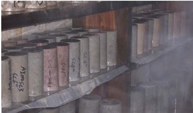
Figure 13. Concrete samples curing
