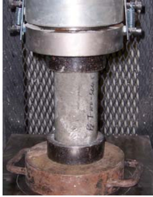
(a) Sample under compression
