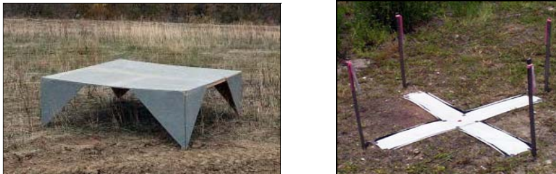
Figure 8-1. Example of fiducial targets used to verify performance of orthophotography and LiDAR systems.
