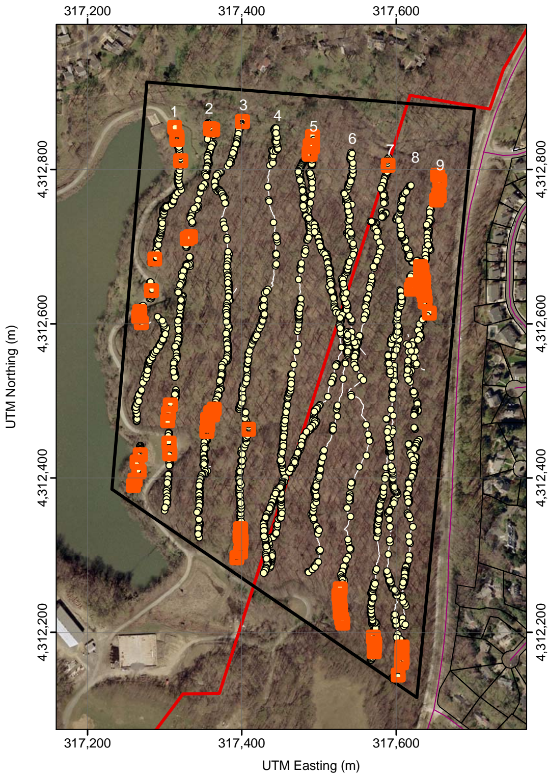
Figure D-26. Areas marked by the analysis module of VSP as exceeding a critical anomaly density of 1,800 anomalies per acre.
