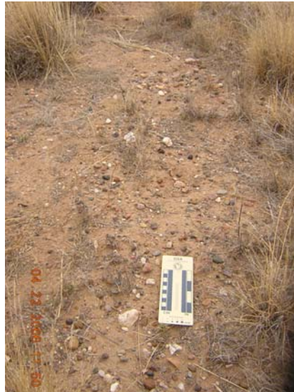
Figure 5-37. The ground reconnaissance team investigated KBPR-AOI-11. The team located a concentration of alluvial pebbles that caused responses from the hand-held magnetometer.
