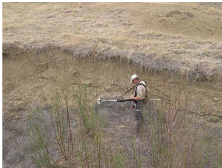
Figure 4-14. Areas in the suspected 75-mm range that were inaccessible due to the vegetation or terrain were investigated on foot. A visual inspection was conducted, supplemented with a hand-held magnetometer, and no evidence of a 75-mm target was found.
