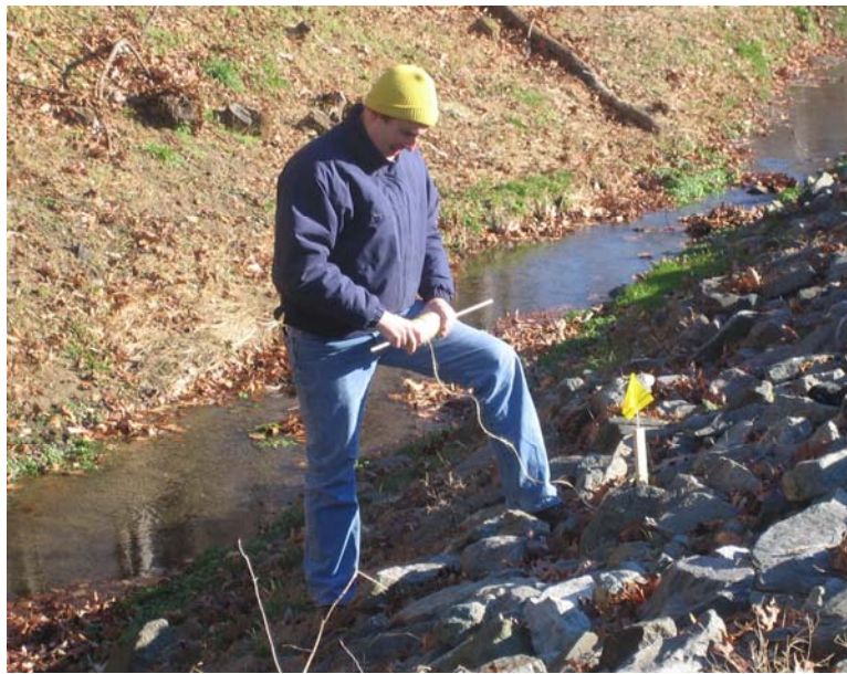
Figure D-15. The transect path is marked by running light string from the two surveyed ends of the transects.
