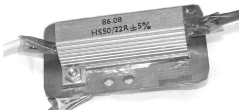
Fig. 2. High wattage resistor attached to cathode plate to apply heat.
