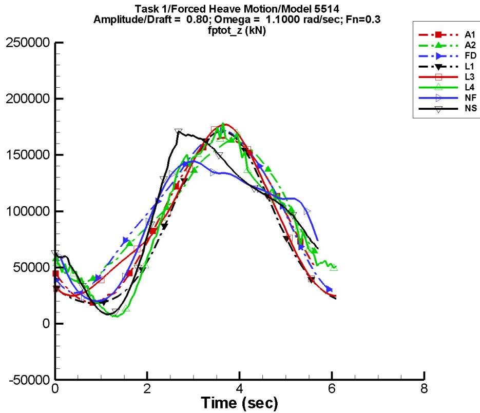
Figure B-90. Time history of  $F_z^{\text{tot}}$  for one period at amplitude/draft = 0.80, frequency = 1.1000 rad/s, Fn = 0.3 in the case of prescribed heave motion of Model 5514 scaled to L = 142 m.
