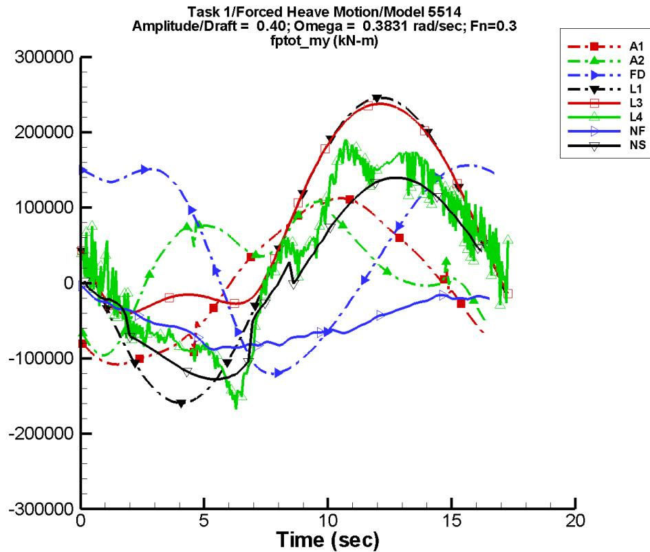
Figure B-114. Time history of  $M_y^{\text{tot}}$  for one period at amplitude/draft = 0.40, frequency = 0.3831 rad/s, Fn = 0.3 in the case of prescribed heave motion of Model 5514 scaled to L = 142 m.
