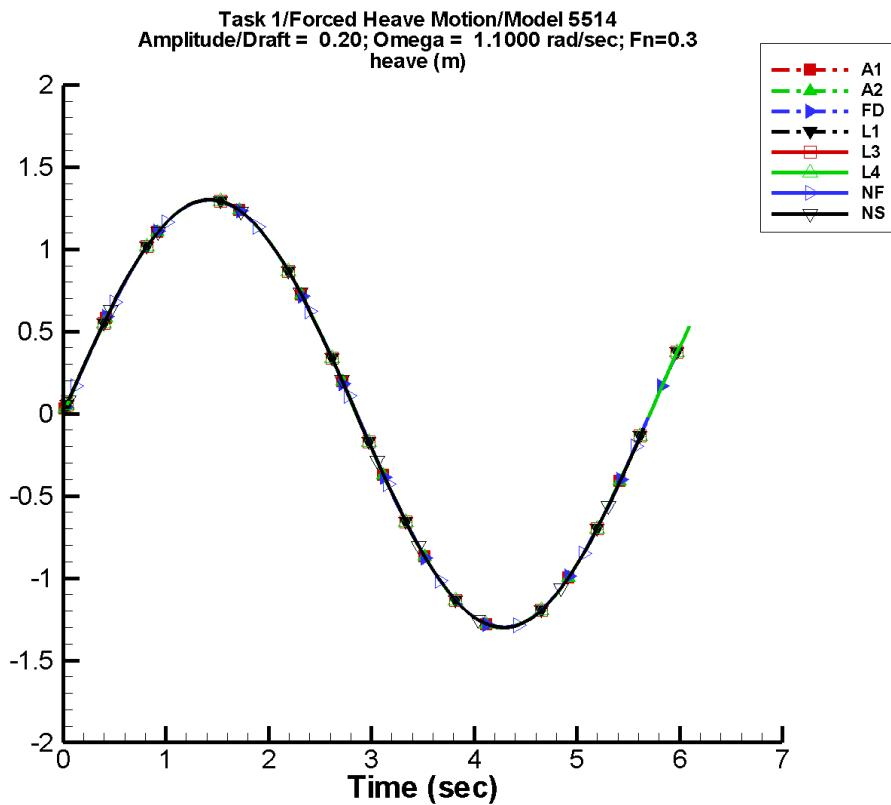
Figure B-28. Time history of  $z_e$  for one period at amplitude/draft = 0.20, frequency = 1.1000 rad/s, Fn = 0.3 in the case of prescribed heave motion of Model 5514 scaled to L = 142 m.
