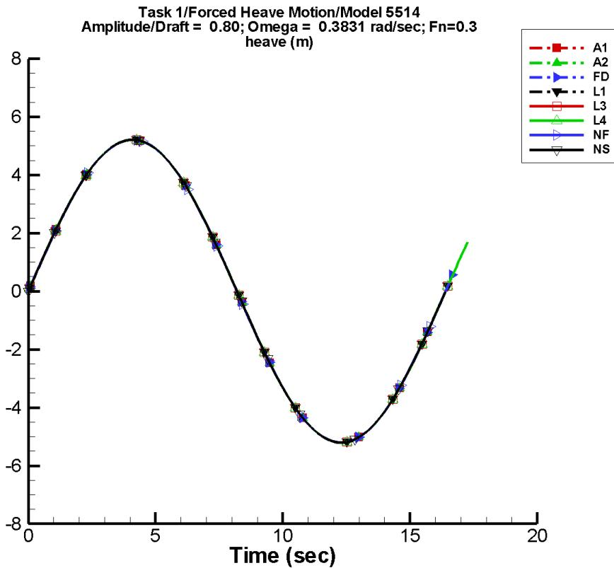
Figure B-25. Time history of  $z_e$  for one period at amplitude/draft = 0.80, frequency = 0.3831 rad/s, Fn = 0.3 in the case of prescribed heave motion of Model 5514 scaled to L = 142 m.
