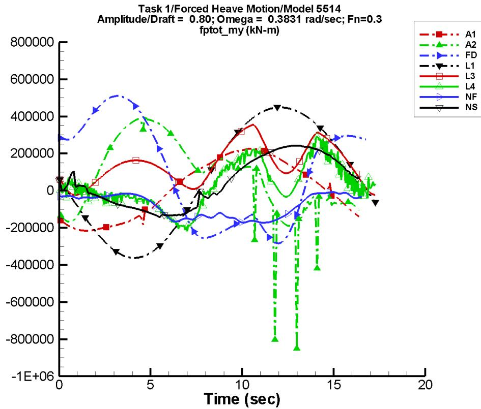
Figure B-115. Time history of  $M_y^{\text{tot}}$  for one period at amplitude/draft = 0.80, frequency = 0.3831 rad/s, Fn = 0.3 in the case of prescribed heave motion of Model 5514 scaled to L = 142 m.
