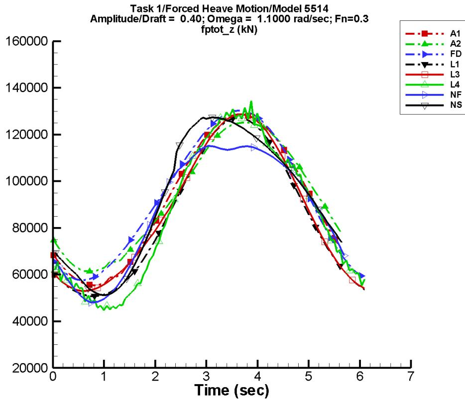
Figure B-89. Time history of  $F_z^{\text{tot}}$  for one period at amplitude/draft = 0.40, frequency = 1.1000 rad/s, Fn = 0.3 in the case of prescribed heave motion of Model 5514 scaled to L = 142 m.
