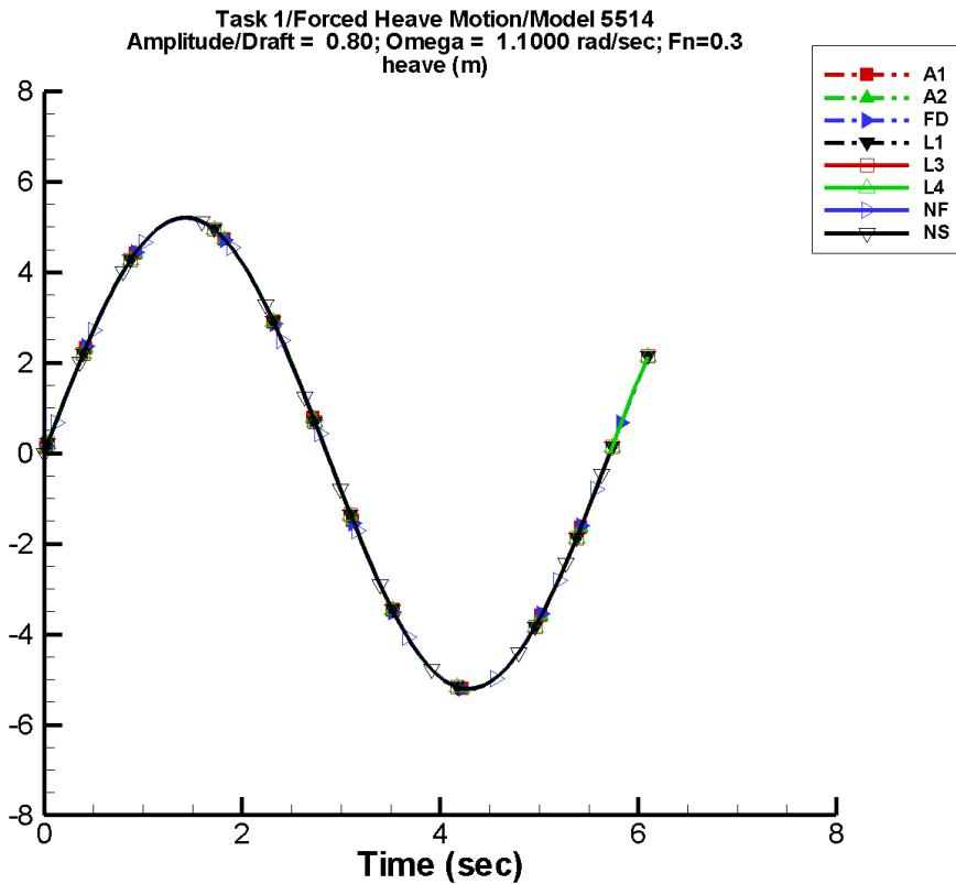
Figure B–30. Time history of  $z_e$  for one period at amplitude/draft = 0.80, frequency = 1.1000 rad/s, Fn = 0.3 in the case of prescribed heave motion of Model 5514 scaled to L = 142 m.
