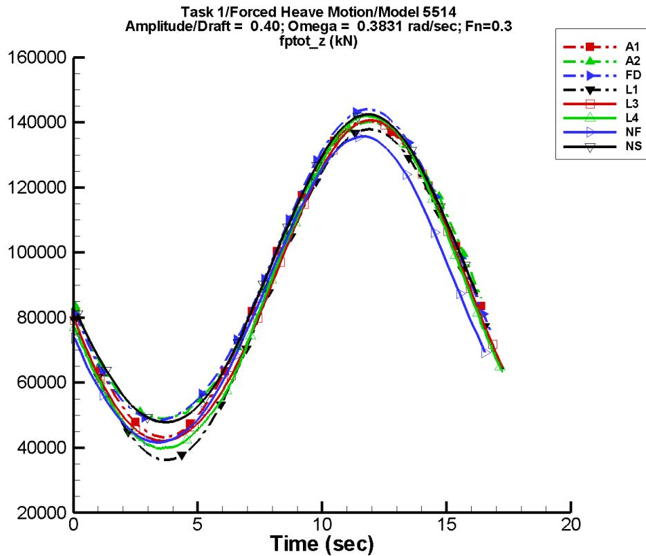
Figure B-84. Time history of  $F_z^{\text{tot}}$  for one period at amplitude/draft = 0.40, frequency = 0.3831 rad/s, Fn = 0.3 in the case of prescribed heave motion of Model 5514 scaled to L = 142 m.
