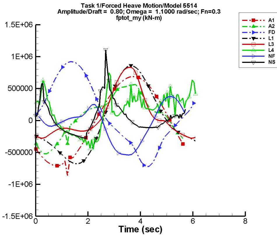
Figure B-120. Time history of  $M_y^{\text{tot}}$  for one period at amplitude/draft = 0.80, frequency = 1.1000 rad/s, Fn = 0.3 in the case of prescribed heave motion of Model 5514 scaled to L = 142 m.
