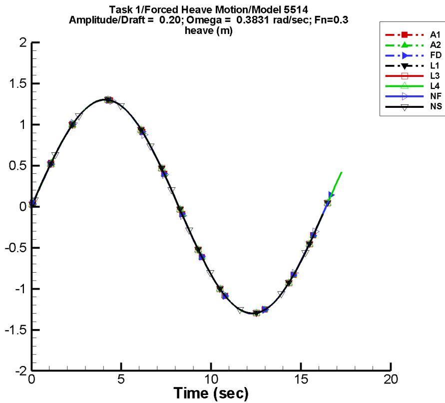
Figure B-23. Time history of  $z_e$  for one period at amplitude/draft = 0.20, frequency = 0.3831 rad/s, Fn = 0.3 in the case of prescribed heave motion of Model 5514 scaled to L = 142 m.
