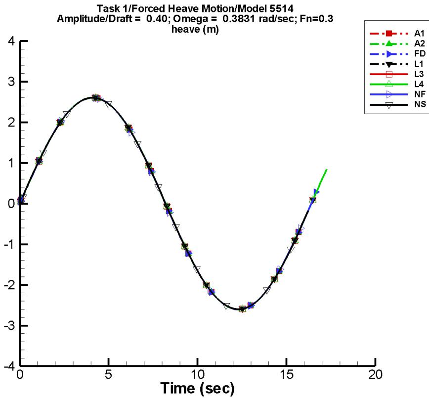
Figure B-24. Time history of  $z_e$  for one period at amplitude/draft = 0.40, frequency = 0.3831 rad/s, Fn = 0.3 in the case of prescribed heave motion of Model 5514 scaled to L = 142 m.
