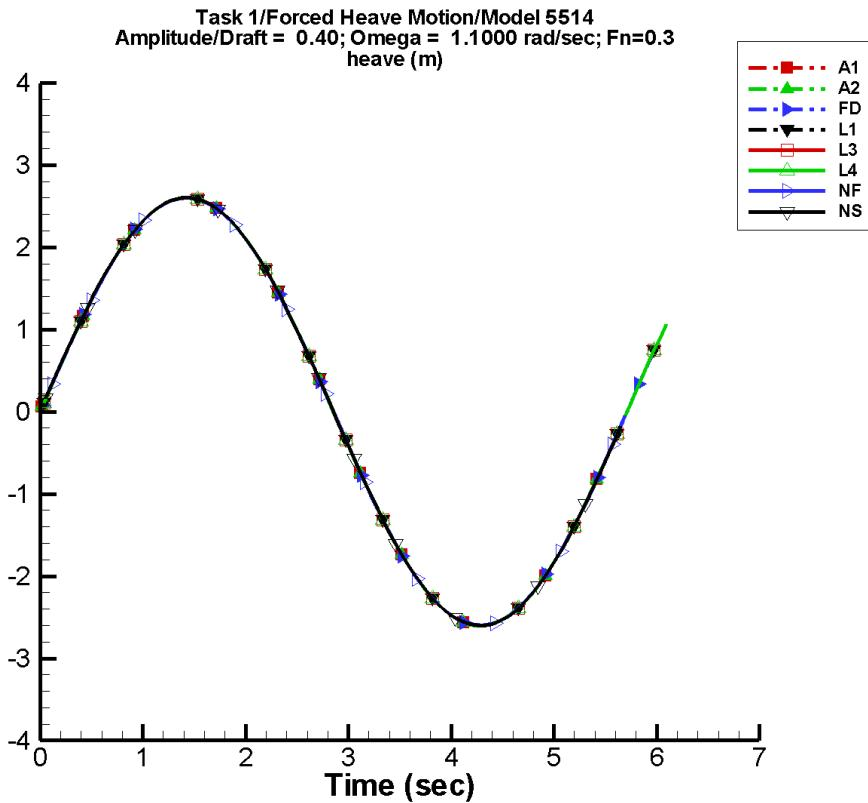
Figure B-29. Time history of  $z_e$  for one period at amplitude/draft = 0.40, frequency = 1.1000 rad/s, Fn = 0.3 in the case of prescribed heave motion of Model 5514 scaled to L = 142 m.
