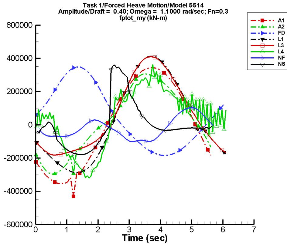
Figure B-119. Time history of  $M_y^{\text{tot}}$  for one period at amplitude/draft = 0.40, frequency = 1.1000 rad/s, Fn = 0.3 in the case of prescribed heave motion of Model 5514 scaled to L = 142 m.
