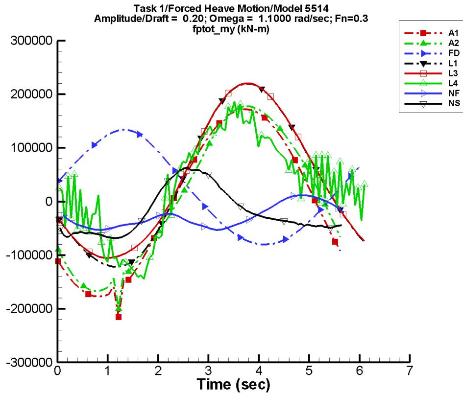
Figure B-118. Time history of  $M_y^{\text{tot}}$  for one period at amplitude/draft = 0.20, frequency = 1.1000 rad/s, Fn = 0.3 in the case of prescribed heave motion of Model 5514 scaled to L = 142 m.
