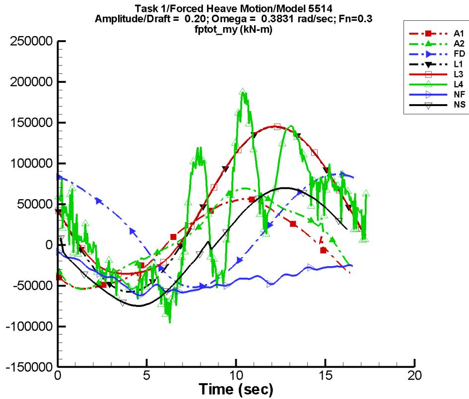
Figure B-113. Time history of  $M_y^{\text{tot}}$  for one period at amplitude/draft = 0.20, frequency = 0.3831 rad/s, Fn = 0.3 in the case of prescribed heave motion of Model 5514 scaled to L = 142 m.
