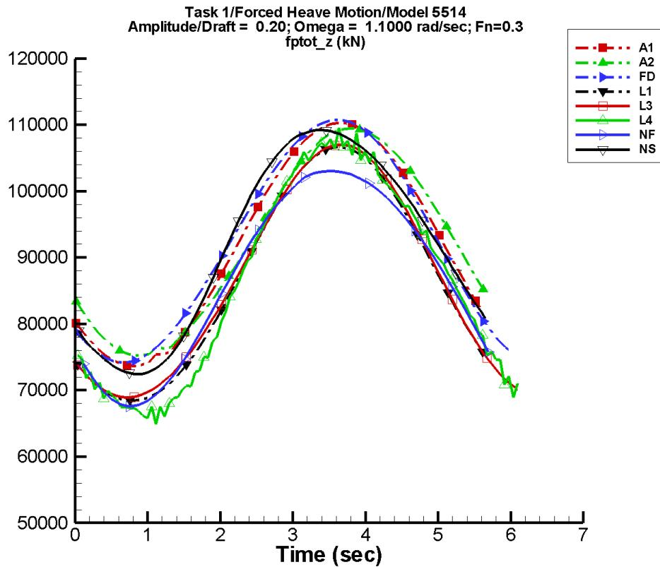
Figure B-88. Time history of  $F_z^{\text{ptot}}$  for one period at amplitude/draft = 0.20, frequency = 1.1000 rad/s, Fn = 0.3 in the case of prescribed heave motion of Model 5514 scaled to L = 142 m.
