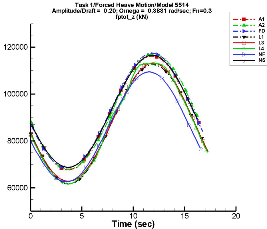
Figure B-83. Time history of  $F_z^{\text{tot}}$  for one period at amplitude/draft = 0.20, frequency = 0.3831 rad/s, Fn = 0.3 in the case of prescribed heave motion of Model 5514 scaled to L = 142 m.
