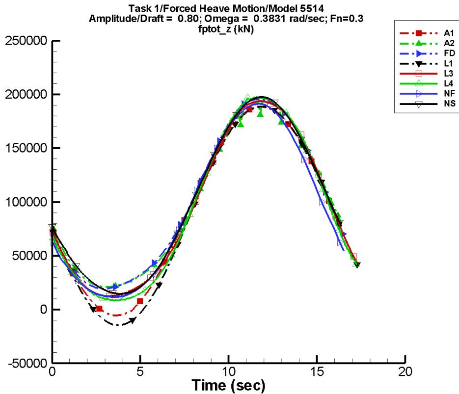
Figure B-85. Time history of  $F_z^{\text{ptot}}$  for one period at amplitude/draft = 0.80, frequency = 0.3831 rad/s, Fn = 0.3 in the case of prescribed heave motion of Model 5514 scaled to L = 142 m.
