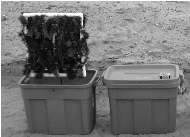
Figure 3. Field instrumentation: Top - Field measurement of deposition velocity of vehicle-generated dust near an unpaved road. Middle - Detail of directional flat substrates prior to removal of the covers for collection. Bottom - Detail of the plastic
