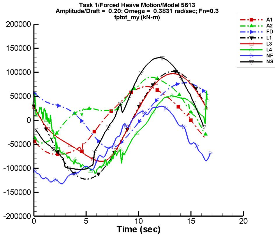
Figure A-113. Time history of  $M_y^{\text{tot}}$  for one period at amplitude/draft = 0.20, frequency = 0.3831 rad/s, Fn = 0.3 in the case of prescribed heave motion of Model 5613 scaled to L = 154 m.
