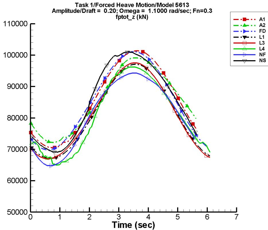
Figure A-88. Time history of  $F_z^{\text{tot}}$  for one period at amplitude/draft = 0.20, frequency = 1.1000 rad/s, Fn = 0.3 in the case of prescribed heave motion of Model 5613 scaled to L = 154 m.
