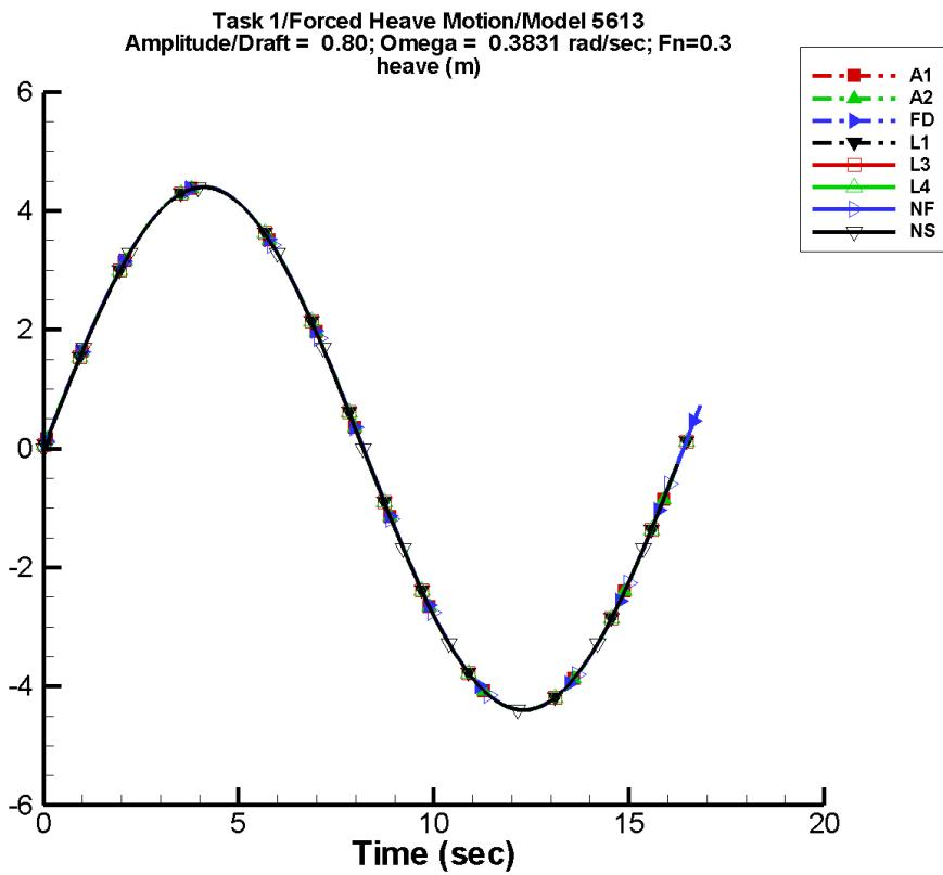
Figure A-25. Time history of  $z_e$  for one period at amplitude/draft = 0.80, frequency = 0.3831 rad/s, Fn = 0.3 in the case of prescribed heave motion of Model 5613 scaled to L = 154 m.
