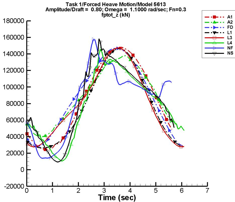
Figure A-90. Time history of  $F_z^{tot}$  for one period at amplitude/draft = 0.80, frequency = 1.1000 rad/s, Fn = 0.3 in the case of prescribed heave motion of Model 5613 scaled to L = 154 m.
