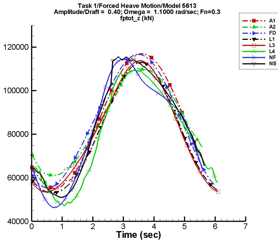
Figure A-89. Time history of  $F_z^{\text{tot}}$  for one period at amplitude/draft = 0.40, frequency = 1.1000 rad/s, Fn = 0.3 in the case of prescribed heave motion of Model 5613 scaled to L = 154 m.
