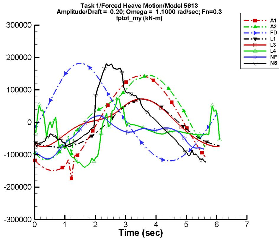
Figure A-118. Time history of  $M_y^{\text{tot}}$  for one period at amplitude/draft = 0.20, frequency = 1.1000 rad/s, Fn = 0.3 in the case of prescribed heave motion of Model 5613 scaled to L = 154 m.
