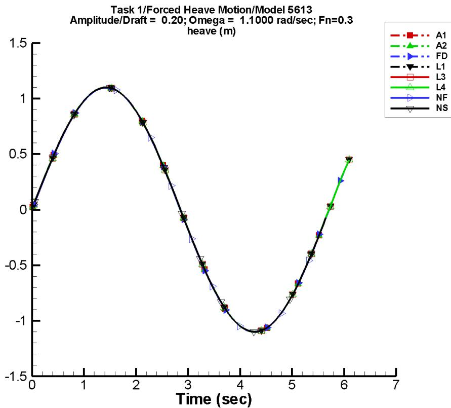
Figure A-28. Time history of  $z_e$  for one period at amplitude/draft = 0.20, frequency = 1.1000 rad/s, Fn = 0.3 in the case of prescribed heave motion of Model 5613 scaled to L = 154 m.
