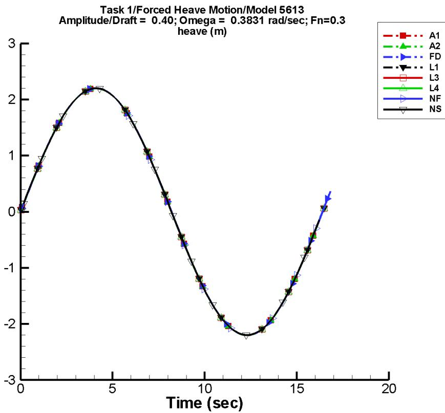
Figure A-24. Time history of  $z_e$  for one period at amplitude/draft = 0.40, frequency = 0.3831 rad/s, Fn = 0.3 in the case of prescribed heave motion of Model 5613 scaled to L = 154 m.
