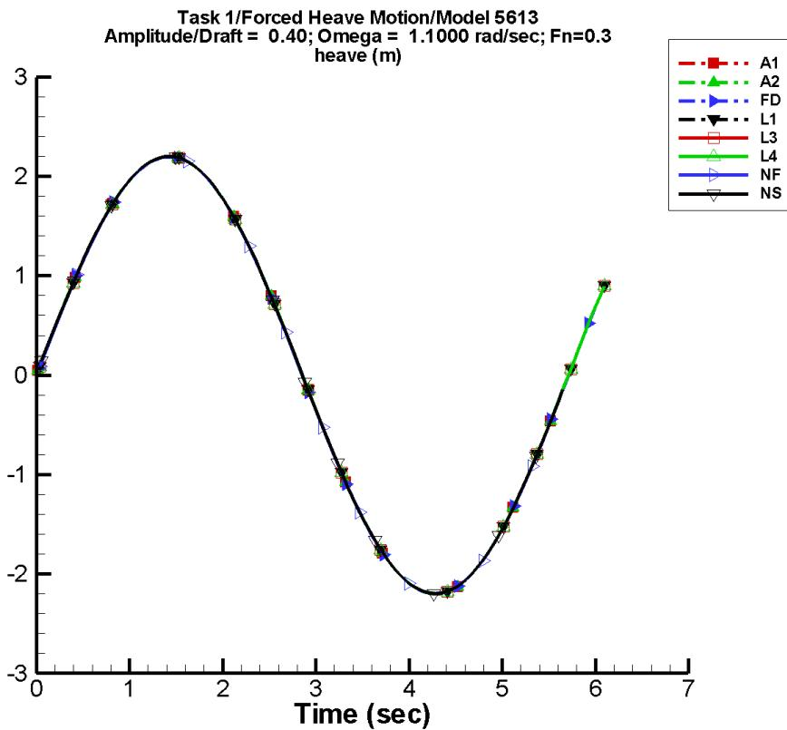
Figure A-29. Time history of  $z_e$  for one period at amplitude/draft = 0.40, frequency = 1.1000 rad/s, Fn = 0.3 in the case of prescribed heave motion of Model 5613 scaled to L = 154 m.
