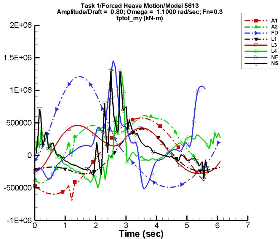
Figure A-120. Time history of  $M_y^{\text{tot}}$  for one period at amplitude/draft = 0.80, frequency = 1.1000 rad/s, Fn = 0.3 in the case of prescribed heave motion of Model 5613 scaled to L = 154 m.
