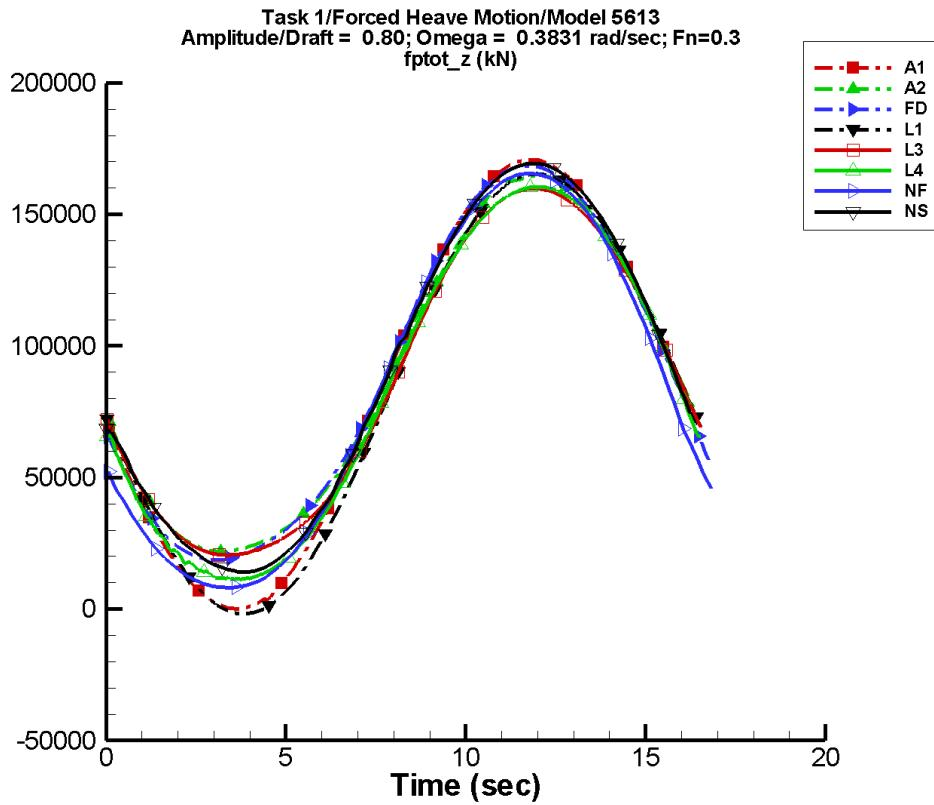
Figure A-85. Time history of  $F_z^{\text{tot}}$  for one period at amplitude/draft = 0.80, frequency = 0.3831 rad/s, Fn = 0.3 in the case of prescribed heave motion of Model 5613 scaled to L = 154 m.
