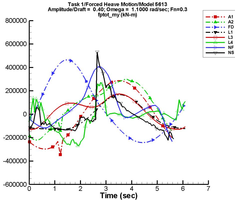
Figure A-119. Time history of  $M_y^{\text{tot}}$  for one period at amplitude/draft = 0.40, frequency = 1.1000 rad/s, Fn = 0.3 in the case of prescribed heave motion of Model 5613 scaled to L = 154 m.
