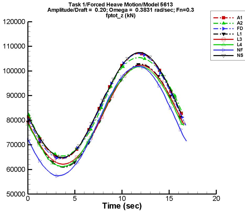
Figure A-83. Time history of  $F_z^{\text{tot}}$  for one period at amplitude/draft = 0.20, frequency = 0.3831 rad/s, Fn = 0.3 in the case of prescribed heave motion of Model 5613 scaled to L = 154 m.
