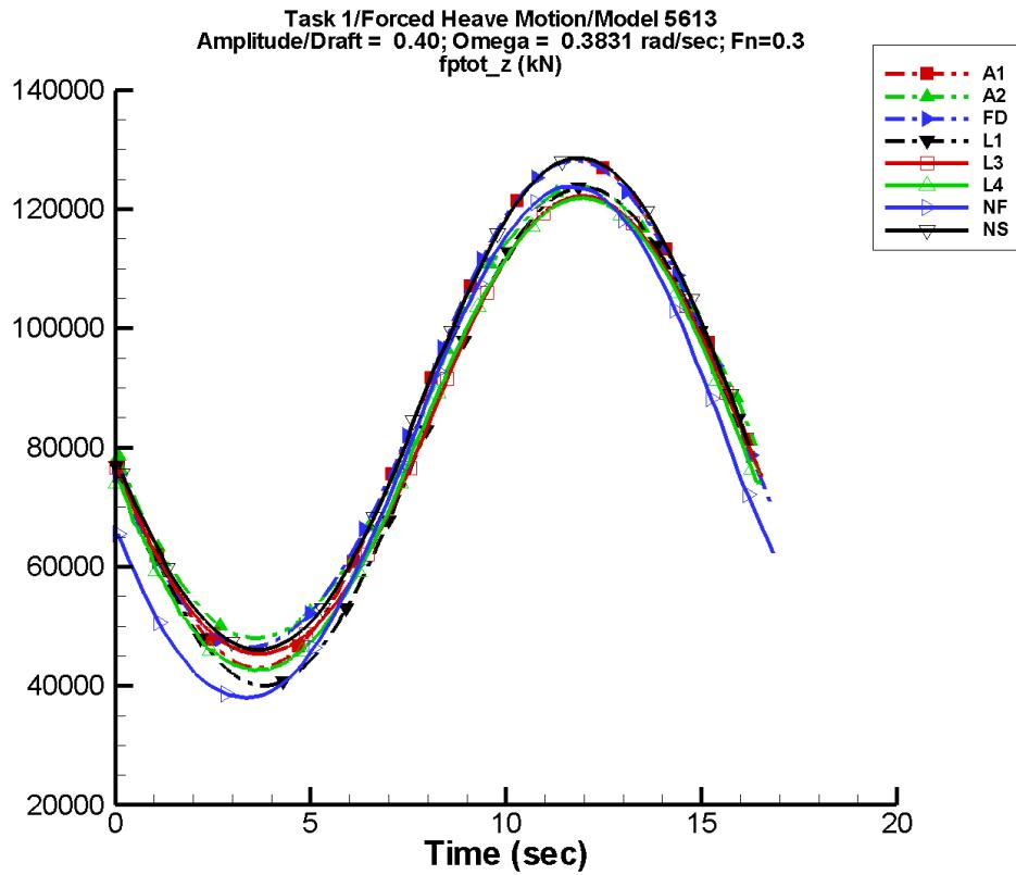
Figure A-84. Time history of  $F_z^{\text{tot}}$  for one period at amplitude/draft = 0.40, frequency = 0.3831 rad/s, Fn = 0.3 in the case of prescribed heave motion of Model 5613 scaled to L = 154 m.
