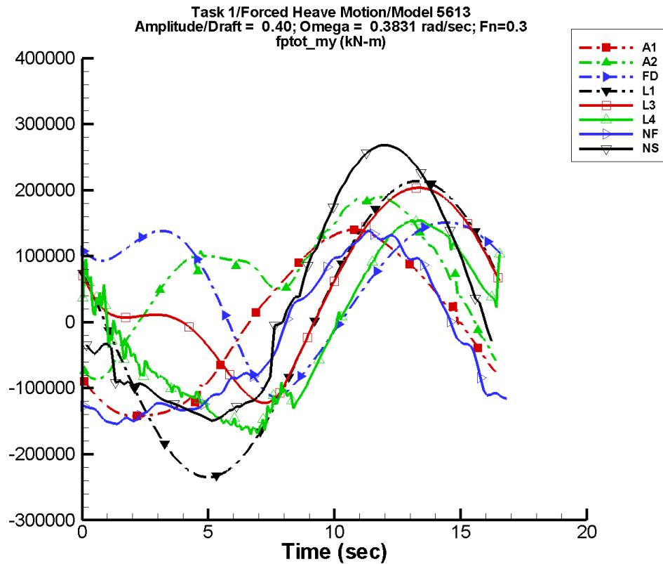
Figure A-114. Time history of  $M_y^{\text{tot}}$  for one period at amplitude/draft = 0.40, frequency = 0.3831 rad/s, Fn = 0.3 in the case of prescribed heave motion of Model 5613 scaled to L = 154 m.
