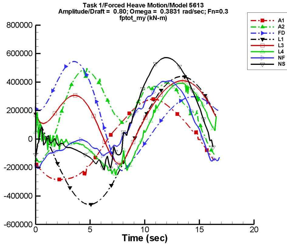
Figure A-115. Time history of  $M_y^{\text{tot}}$  for one period at amplitude/draft = 0.80, frequency = 0.3831 rad/s, Fn = 0.3 in the case of prescribed heave motion of Model 5613 scaled to L = 154 m.
