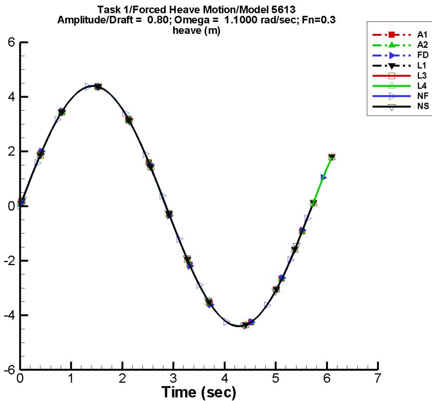
Figure A-30. Time history of  $z_e$  for one period at amplitude/draft = 0.80, frequency = 1.1000 rad/s, Fn = 0.3 in the case of prescribed heave motion of Model 5613 scaled to L = 154 m.
