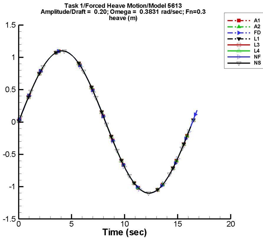
Figure A-23. Time history of  $z_e$  for one period at amplitude/draft = 0.20, frequency = 0.3831 rad/s, Fn = 0.3 in the case of prescribed heave motion of Model 5613 scaled to L = 154 m.
