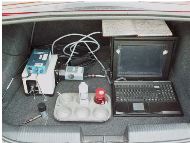
Figure 2. Photograph of the Portable Raman Instrument in the Trunk of a Rental Car at the ALAAP. (The laser (blue) is sitting on top of the spectrograph (white) with a multichannel CCD detector (light blue) attached. In the foreground is the fiber optic Raman probe inserted in the sample chamber. Reagents for the SERS method are in the muffin tin.)
