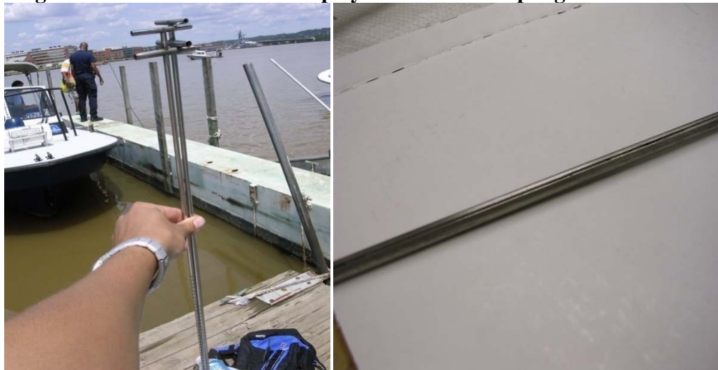
Figure 8: Picture of Field Deployable SPME Sampling Device.
