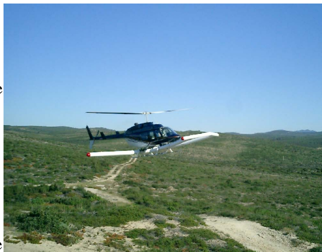
Figure 16: ORNL Arrowhead system in operation at Fort Ord. Notice the ridge and trough topography, which is apparently correlated with the anisotropic magnetic background.
