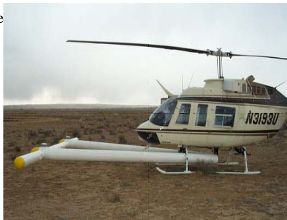
Figure 22: The MTADS airborne system deployed at Pueblo of Isleta, NM. The flat terrain and minimal vegetation made it possible to survey this site with average flight heights below 2 m (Nelson et al., 2003).
