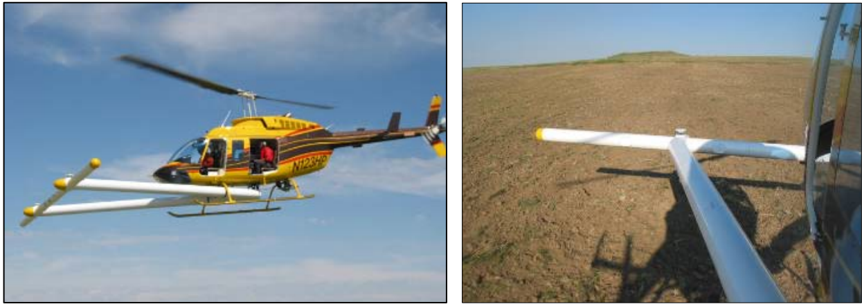
Figure 1. Helicopter MTADS technology as deployed on Bell Long Ranger helicopter.
