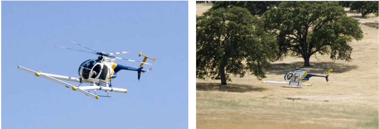
Figure 2. Helicopter and magnetometer boom assembly. Seven magnetometers are contained in the composite-material boom and positioned with the GPS antenna and laser/acoustics altimeters.
