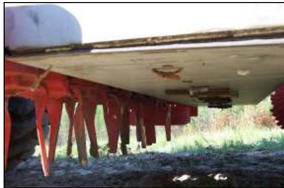
Figure 33: Metal Attracted to Magnet
