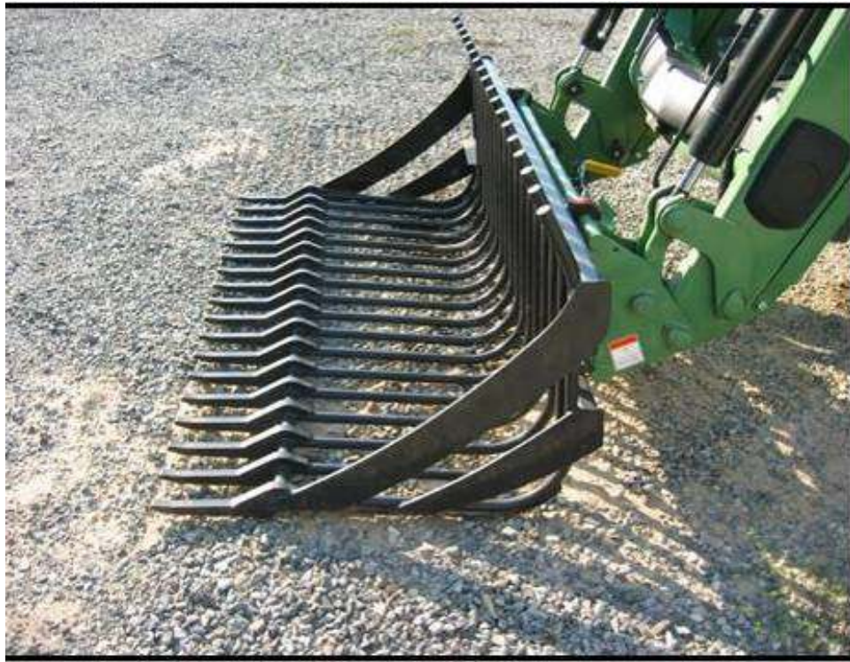
Figure 10: Quicke Rock Bucket (Stone Fork, Model 180)
