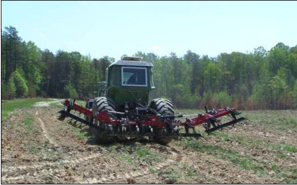
Figure 5: Unverferth Spring Cultivator Being Extended
