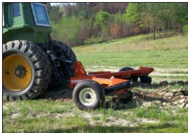
Figure 20: Operating Position, Miskin Parabolic Subsoiler
