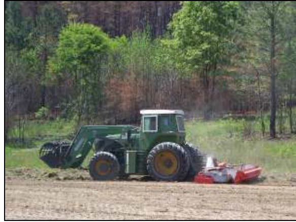
Figure 32: Power Harrow with Magnet Operations
