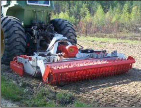
Figure 31: Power Harrow with Magnet Operations
