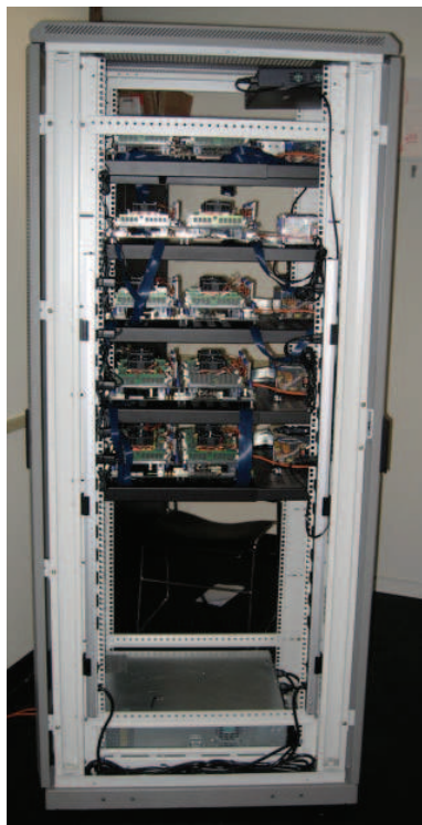
Figure 9: TRIPS Rack-based System with 5 Motherboards, 20 TRIPS Chips, and 40 TRIPS Processors
