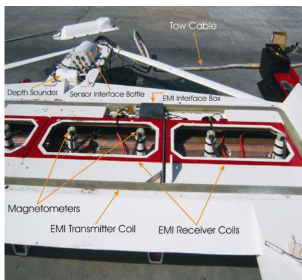
Figure 6. The marine sensor platform is shown with the hatch covers removed. Many of the system components are identified.
