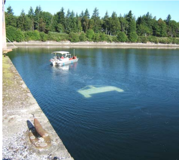
Figure 1. The 30 ft pontoon boat is shown towing the sensor platform during a survey on Ostrich Bay. The sensor platform is submerged about 7 ft below the surface.
