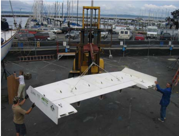
Figure 12. A larger hoist is used to unload the sensor platform and later load it back onto the MTA vessel boat trailer. It cannot be lifted from below with a fork lift.
