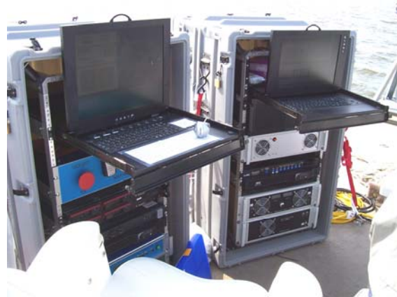
Figure 3. All sensor data are recorded by the computers in these data racks mounted across from the drive console, near the port rail.
