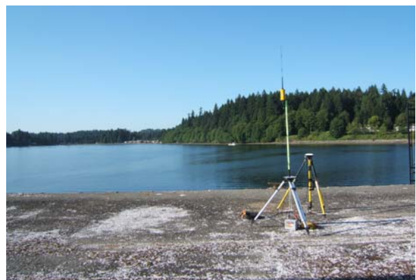
Figure 17. The GPS base station is shown set up on the Primary Control Point, which was established during earlier operations.
