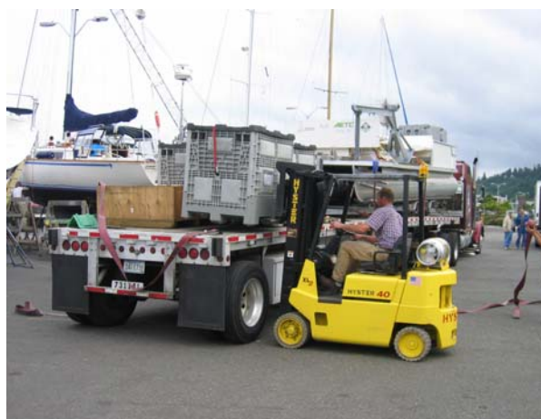
Figure 11. A small fork lift is used to unload the crated equipment from the shipping trailer into a rented box truck.
