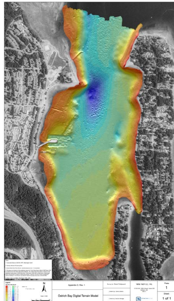
Figure 19. False color bathymetric image of Ostrich Bay overlaid on a recent aerial photograph of the area.
