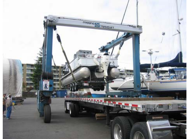
Figure 13. A large marine hoist is used to unload the MTA vessel and the trailer together. It is difficult to lift the vessel alone without damaging the pontoons.
