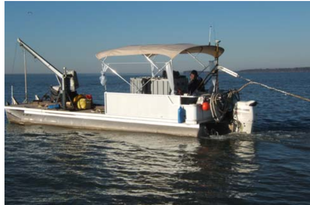
Figure 2. The tow point fixture is located at the rear of the boat. The master GPS antenna is located on the mast above this point. The digital angular encoder measures the angle of the tow cable relative to the boat heading. The weak link cable is located between the shackles at the end of the tow arm.
