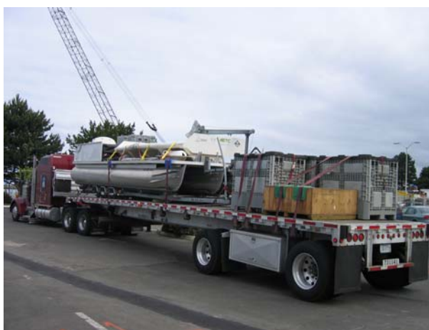
Figure 10. The entire MTA system is shipped on the deck of a 45 ft trailer.
