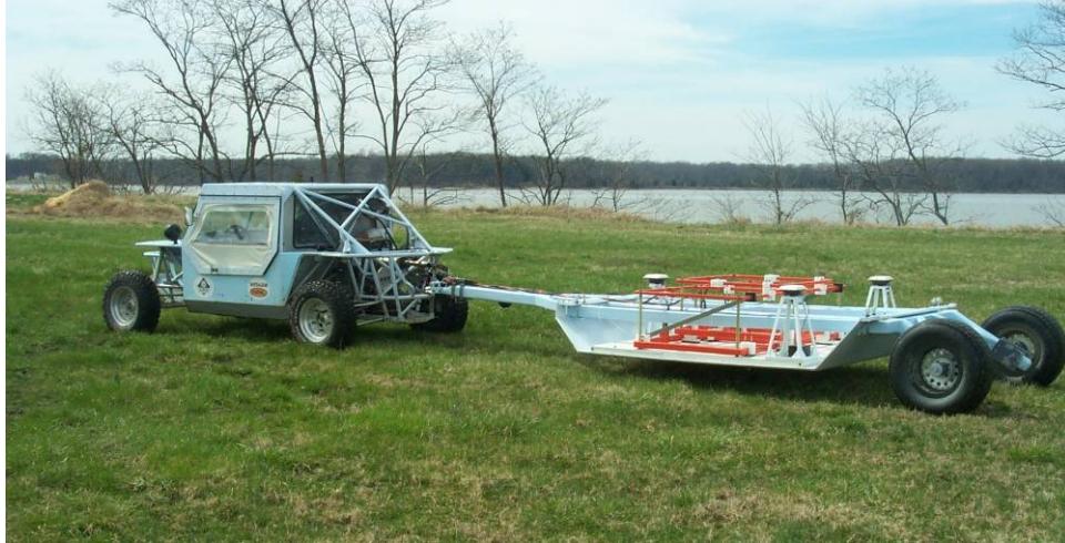
Figure 2-4. Photograph of NRL's Multi-Sensor Towed Array Detection Systems (MTADS).
