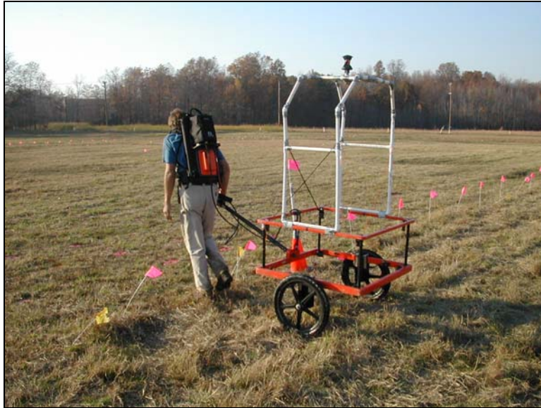
Figure 2-2. Photograph of TTFW's EM61 MK2 sensor system during data acquisition at the open field area of APG.
