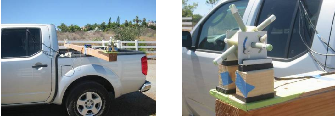
Figure 9. Photos of vehicle tests. Left: Boom with 3-axis sensor mounted on driver's side and reference sensor mounted on passenger side. Right: Close-up of 3-axis sensor mounted on boom and aligned to Earth's field.
