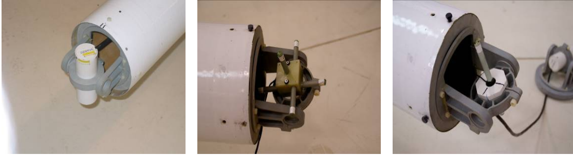
Figure 5. Left: Photo of Sky Research sensor mounting gimbal, holding a Cs-Vapor magnetometer. Middle and Right: Sky research gimbal holding the QFS 3-axis induction sensor and single axis reference sensor.
