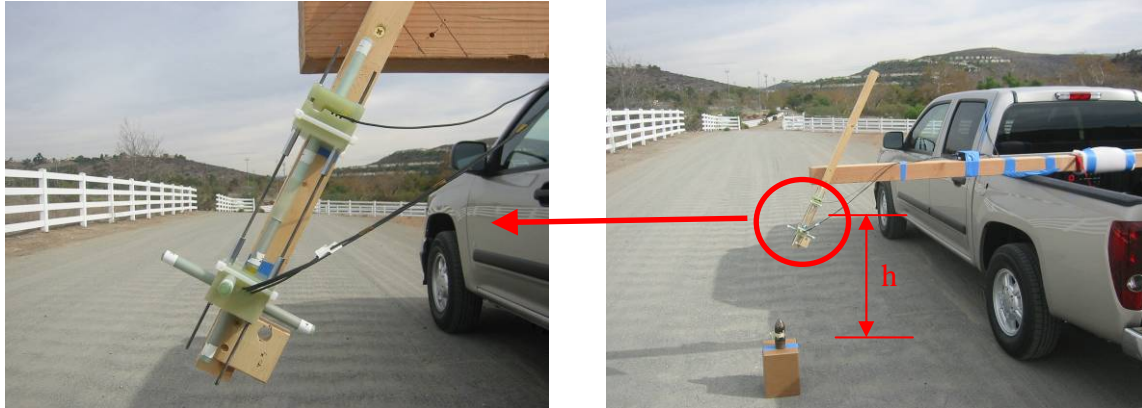
Figure 17. Left: Gradiometer configuration with reference sensor mounted rigidly above 3-axis main sensor. Right: Repeat of vehicle tests with gradiometer, using 57 mm shell target.
