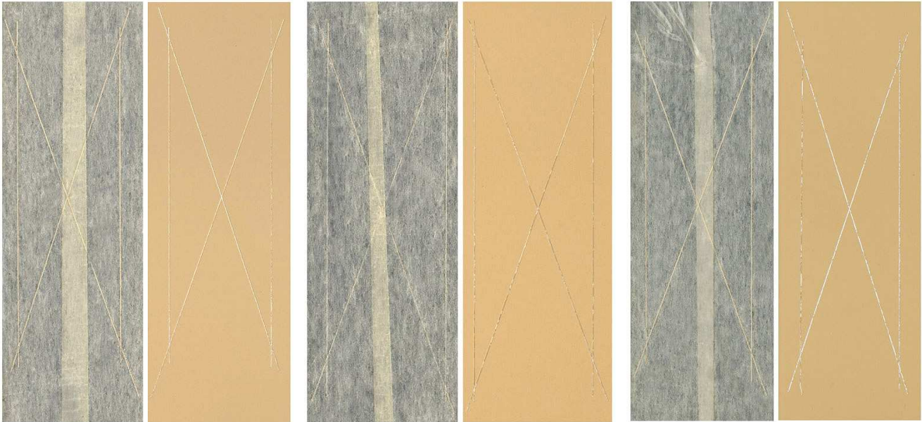
(a) (b) (c) Figure 6: 1 Week 150°F Immersed Wet Adhesion Panels Representative Scans Showing Coating Surface Incisions and Corresponding Test Tape Back Sides, All Rated at 5A per ASTM D 3359A (a) NCP, (b) TCP, (c) Grit Blast
