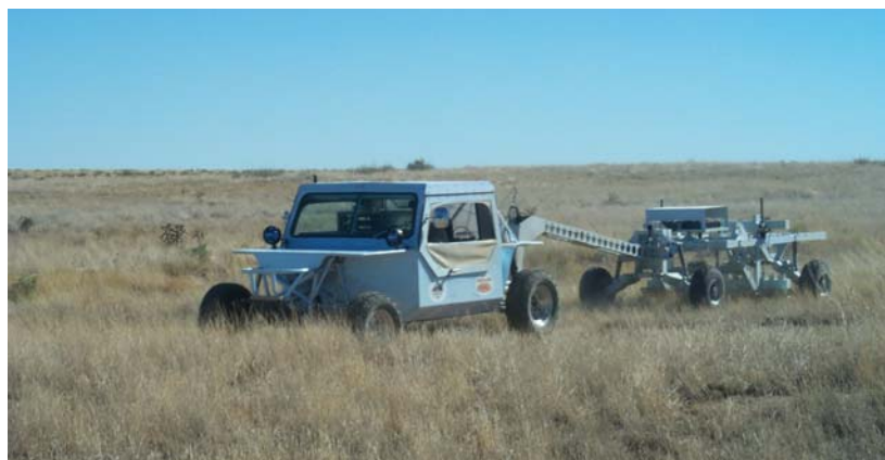
Figure 1. MTADS Vehicle Towing the Magnetometer Array.
