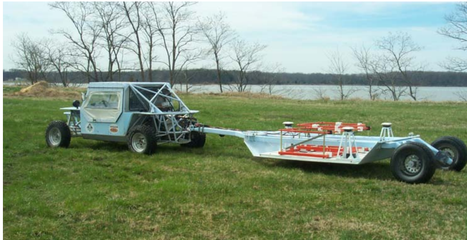
Figure 2. MTADS EM61 Array Pulled by the MTADS Tow Vehicle.
