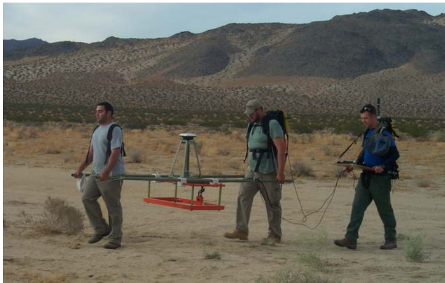
Figure 4. MP, Litter-Carried EM61 MkII Sensor System.
