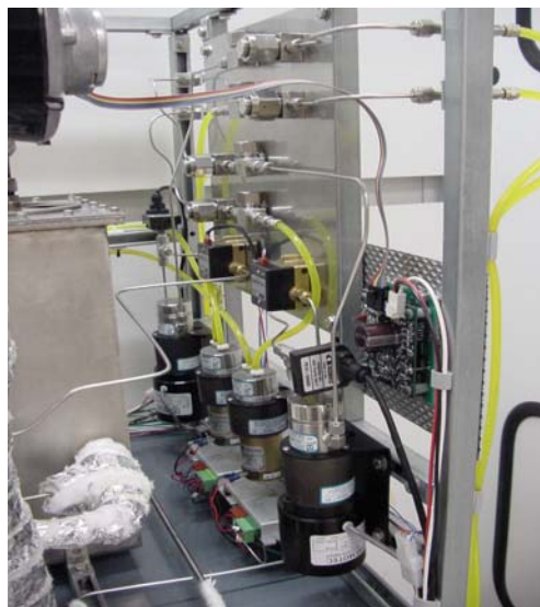
Figure 7: Balance of Plant – Reformer Burner Fuel Pump, Steam Generator Burner Fuel Pump, Process JP-8 Pump, and Process Water Pump
