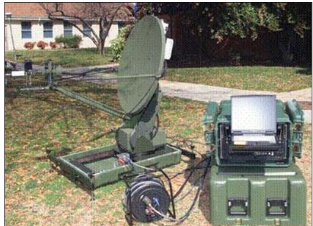
(Right) Figure 4. CSS Very Small Aperture Terminal System
