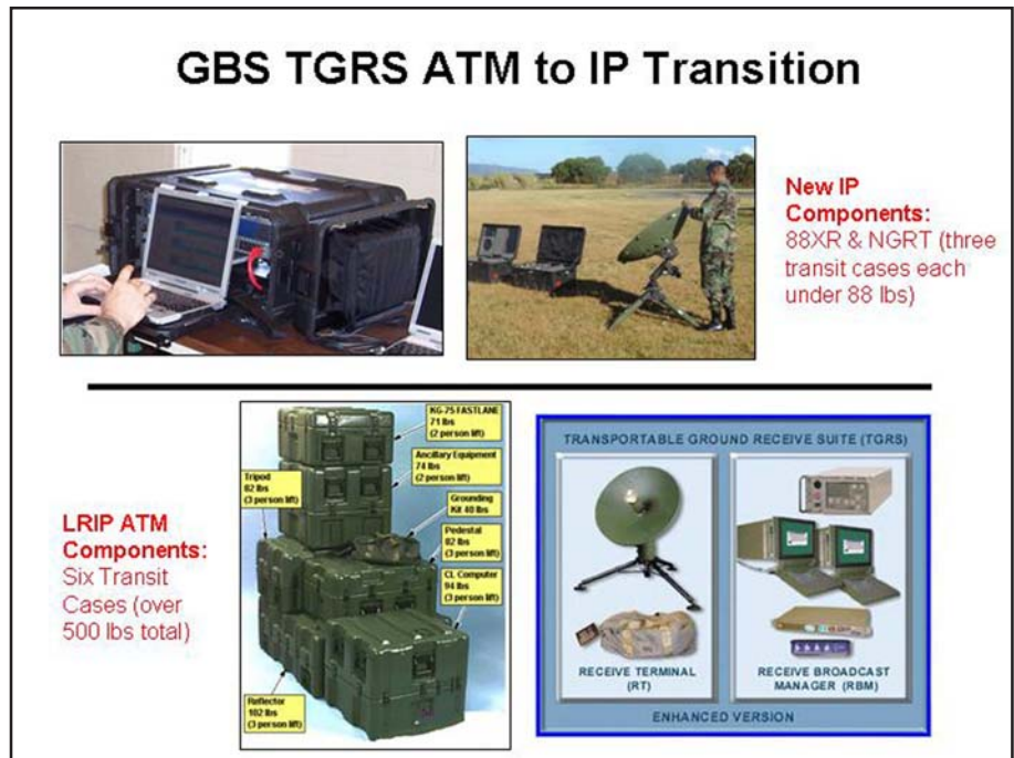
(Above) Figure 3. GBS Portable Ground Receive Suite (AN/TRC-4) and IP Transition
