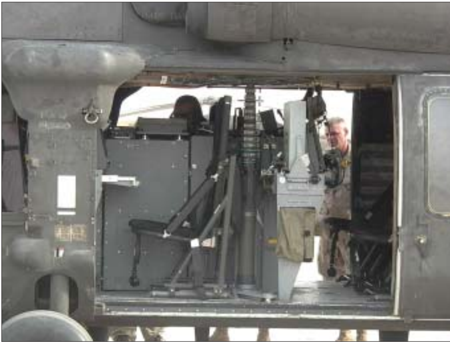
Product Manager for Blue Force Tracking, LTC John Bullington, checks out the first full-production model of the Army Airborne Command and Control System. A2C2S is a suite of five computer displays built in a UH-60 Blackhawk helicopter where a command staff can control a battle even during flight.
