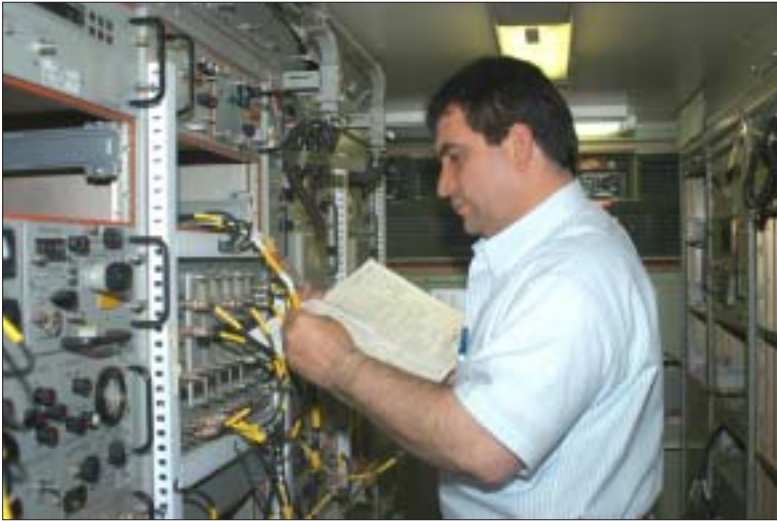
John Morelli, electronics mechanic leader, Satellite Communications Systems Directorate, checks new cabling in a prototype AN/TSC-85D Ground Mobile Forces Tactical Satellite communications terminal. Tobyhanna is upgrading the TSC-85 and the AN/TSC-93 to the D model to extend their service through 2012.
