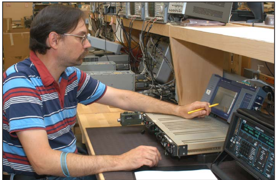
Stephen Bucklaw tests a KIV-19 Trunk Encryption Device at Tobyhanna Army Depot. He developed a procedure to screen and make minor repairs to KIV-19s, saving time and money. Bucklaw is an electronics mechanic leader in the depot's Communications Security and Tactical Missile Systems Directorate.
