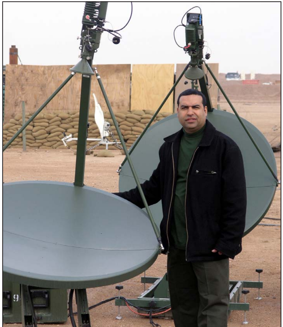
Efren Morales is shown here in Kuwait with Combat Service Support Very Small Aperture Terminals of the type the Product Manager, Defense Wide Transmission System provided to support Hurricane Katrina relief efforts. CSS VSATs along with Combat Service Support Automated Information Systems Interfaces together make up the CSS SATCOM system, the same seamless solution PM DWTS is providing to Soldiers in Iraq and elsewhere around the world to support the Army G-4's 'Connect Army Logisticians' initiative.
