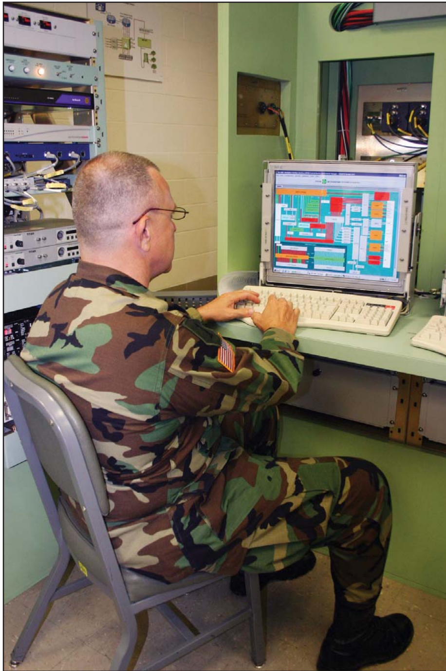
WO Francois Pelletier, Company B, 442nd Signal Battalion, monitors the Warfighter Machine Interface of the Joint Network Node. The WMI displays all of the JNN activity and maps out the physical locations of the JNN modules. Pelletier describes the JNN as "an (Internet Technology) department on wheels."
