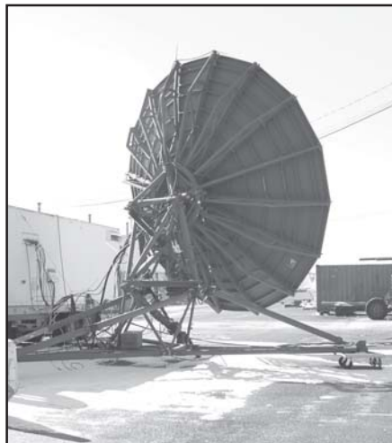
(Right) AN/TSC-86A terminals can receive, transmit and process medium and high capacity multiplexed voice and data.
