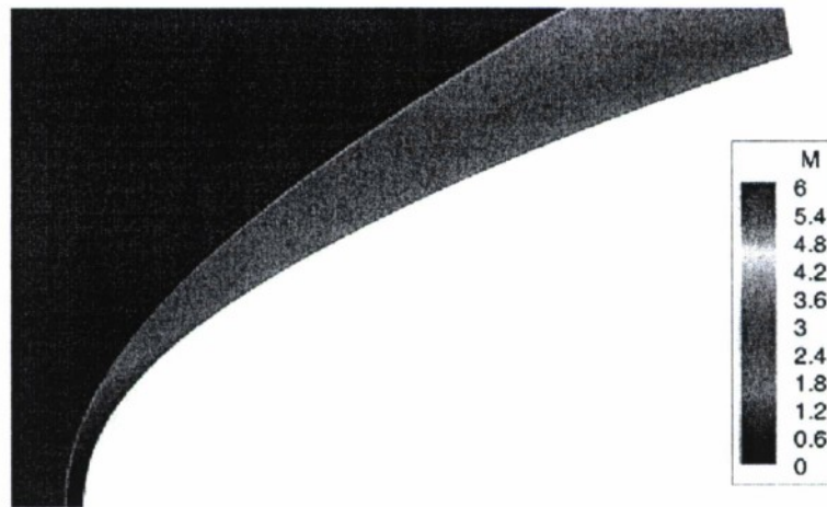
Figure 3: Sample CFD-simulation (Mach number contours) of the re-entry body flowfield
