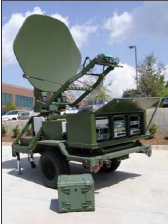
(Above) The RWS Data Package houses the brains of the system. A Promina 400 platform provides NIPR, SIPR, Voice and VTC capabilities.
