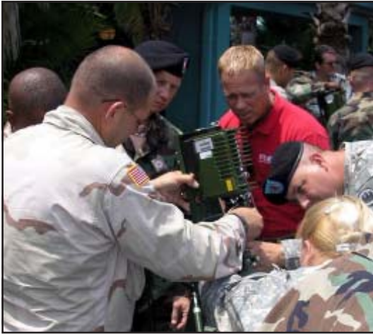
Product Manager, Defense Wide Transmission Systems fielding team member Rick Ackerley (second from right) assists National Guard Soldiers to connect the antenna feed horn assembly to a Combat Service Support Very Small Aperture Terminal on May 10 in Orlando, Fla.
