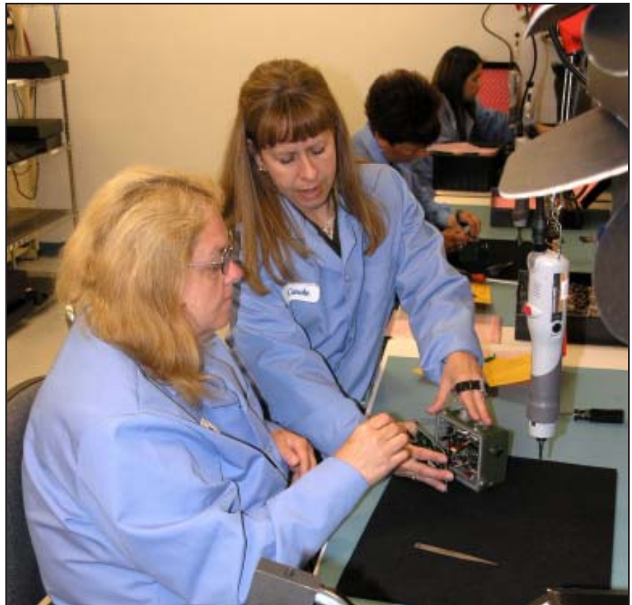
Workers assemble a crew station light box – one the modules of the Vehicle Intercom System– at the new Cobham Defense Electronic Systems VIS production facility in Manchester, N.H.
