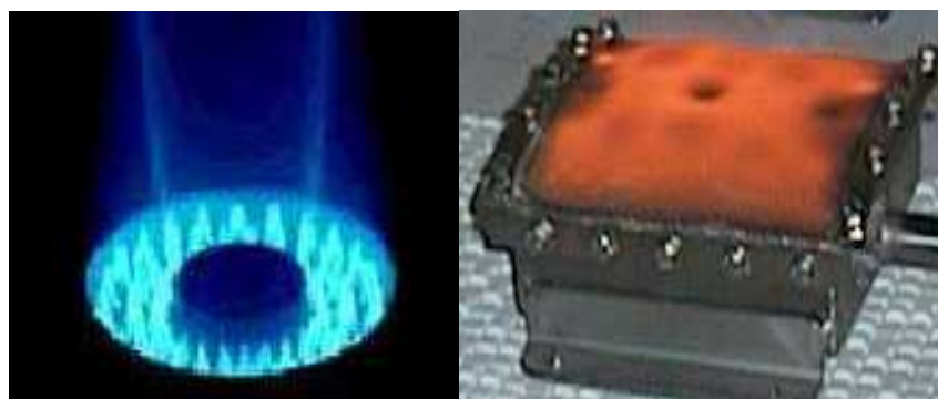
Figure 5: A close-up photograph of Sydney University's 'blue-flame' burner (left) and DSTO's Porous Radiant Burner (right).
