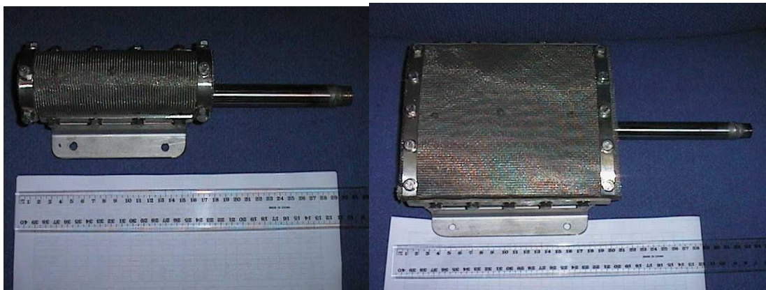
Figure 1: Close-up photographs of semi-cylindrical wire-mesh (left) and flatbed (right) burners.
