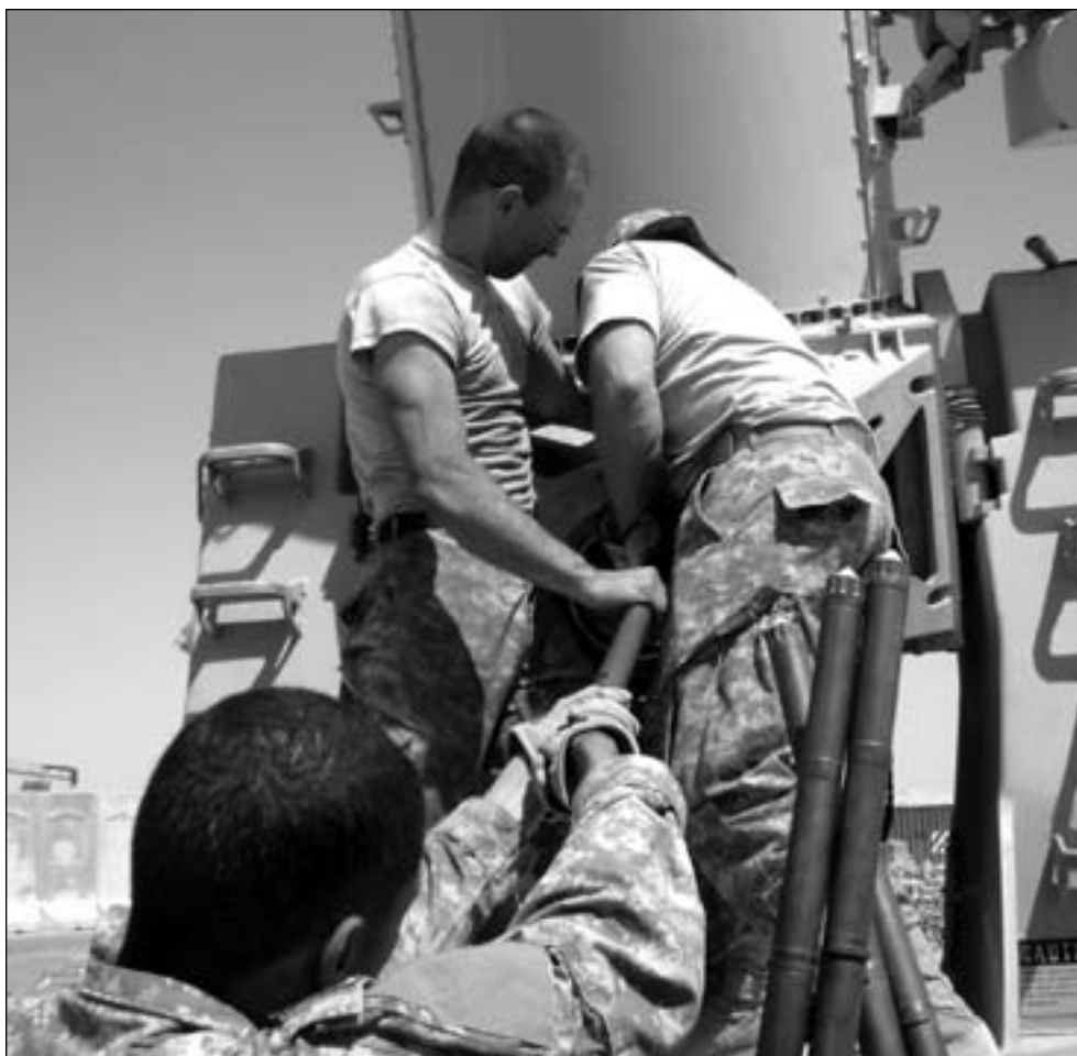
During routine maintenance on a Land-Based Phalanx Weapon System, US Navy Sailors FC1 (SW) Yusuf Kezala hands a barrel to FC2 Robert Armstrong (left) and FC2 Jeremiah Stellpflug, members of the Joint Intercept Battery Task Force (TF) Iron Shield, composed of both Army and Navy members, in Baghdad, Iraq, 24 July. (Photo by FCCS [SW] Donald Leppert, TF Iron Shield)
