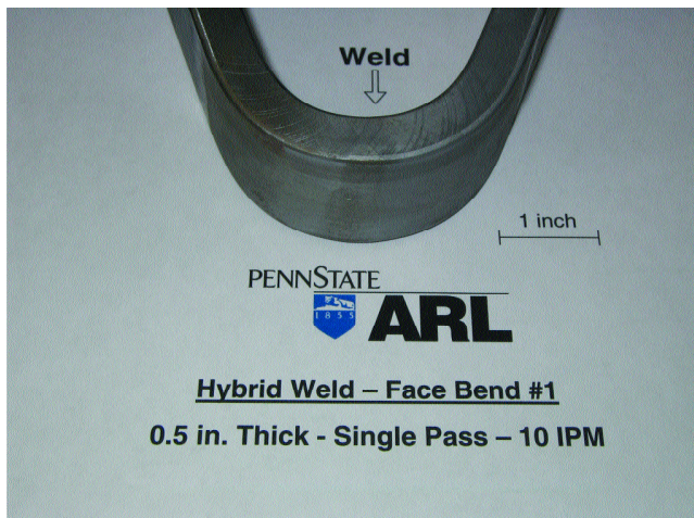
Fig. 10 — Mechanical testing of hybrid weld in 0.5-in.-thick mild steel indicated adequate mechanical properties.
