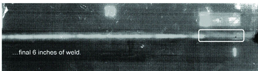
Fig. 11 — Radiographic testing of hybrid weld in 0.50-in. (12.7-mm) -thick mild steel reveals a small amount of porosity confined to regions near the end of the weld.
