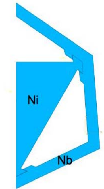
Figure 17: Dovetail configuration of lattice cell
