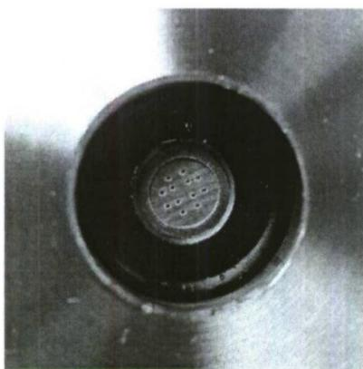
Fig. 2. The 12 fuel injector ports for our prototype reactor. The fuel injector is inserted into a specially modified 2.75 inch conflate flange.
