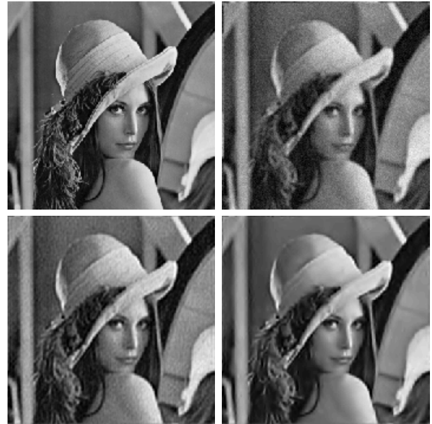
Figure 3: Upper left: Lena image x ( 256 \times 256 ). Upper right: Observed image y ( MSE=0.457 ). Lower left: Wiener filter estimate ( MSE=0.199 ). Lower right: WaRD with \alpha = 0.27 ( MSE=0.182 ).
