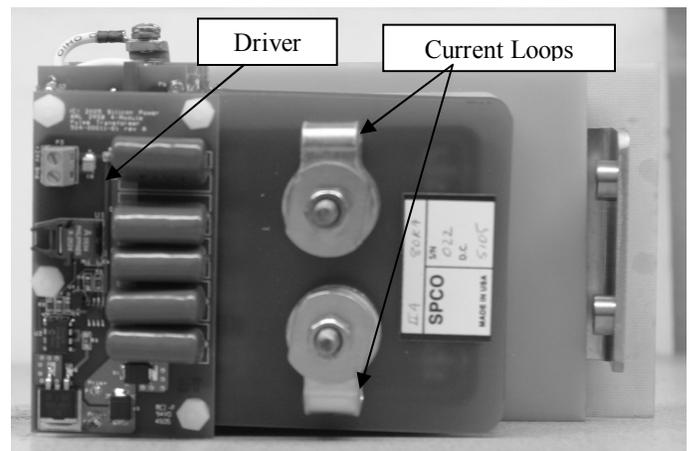
Fig. 3. Top view of 80 kA, 10 kV switch with driver and current loops attached.
