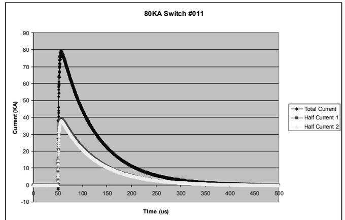
Fig. 8. Data from the ring down circuit at 80 kA and 7.5 kV. This graph shows the total current as well as how well each of the two cathode current loops shared the total current.
