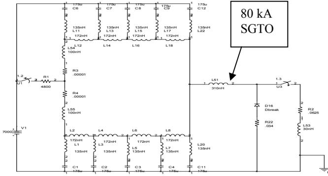
Fig. 6. A Pspice schematic of the 5 stage parallel PFN used to test the 80 kA, 10 kV switch.
