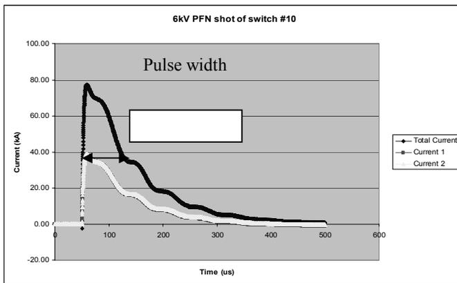
Fig. 10. Data from the successful PFN test shot with the total current waveform as well as how well each half of the module shared the total current.
