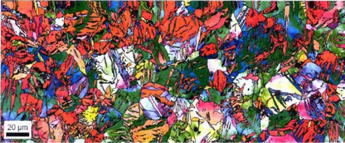
Figure 10: Orientation Imaging Microscopy map showing significant twinning activity (45% volume fraction) in the  $\alpha$ -titanium sample deformed to 20% strain in simple compression along the rolling direction.
