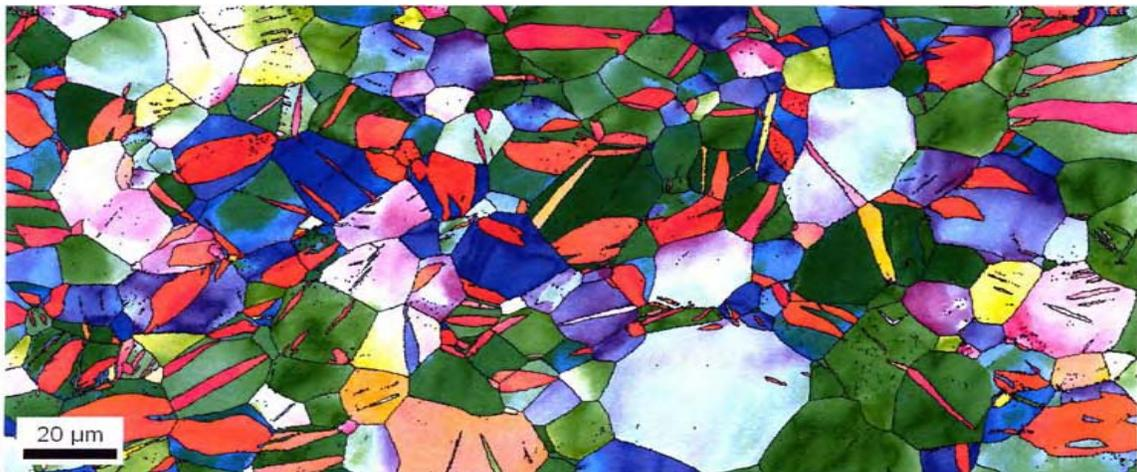
Figure 9: Orientation Imaging Microscopy map showing the evidence of twins (in red) in the specimen deformed to 10% strain in simple compression along the rolling direction. The twin volume fraction is 17%.
