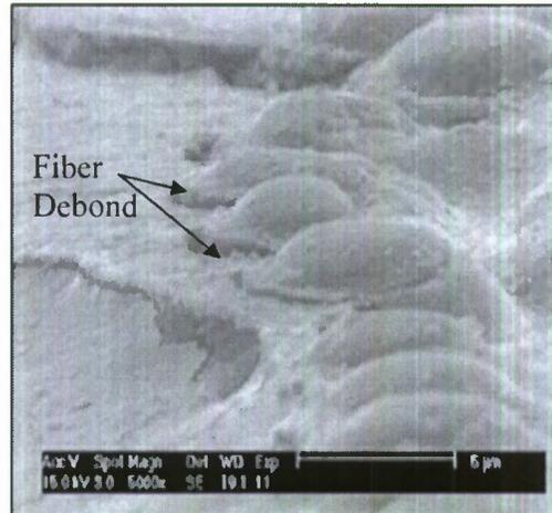
**Figure 1.** Micrograph of fiber/matrix debond due to thermo-oxidation in G30-500/PMR-15 composite at 288 °C in air. [10]
