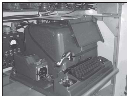
FIG 1. Circa 1959 the TT-76 reperforator-transmitter provides perforated tape copies of teletypewriter messages received, or transmits messages pre-recorded on perforated tape.
