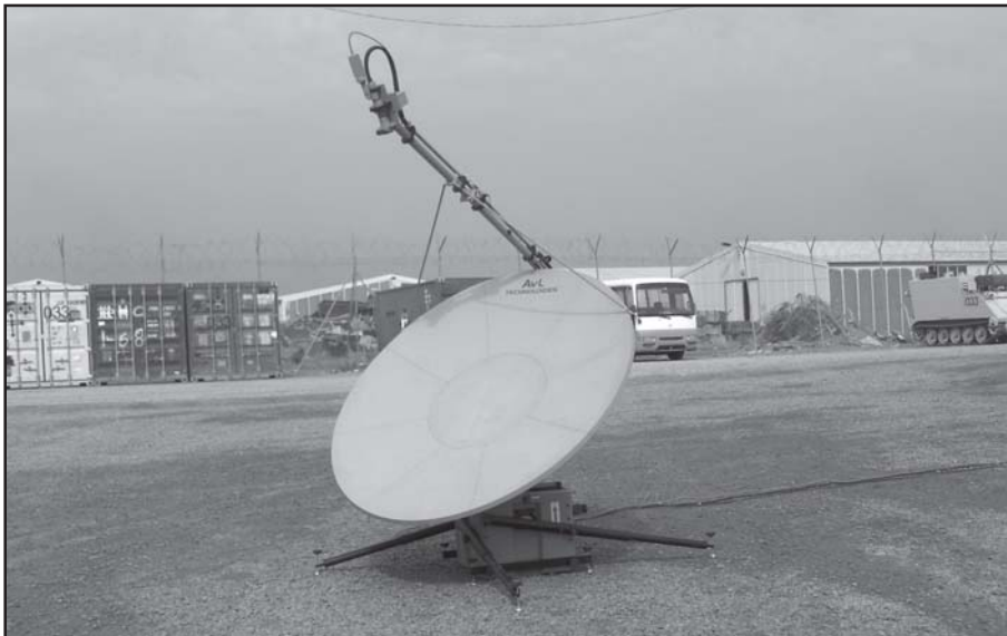
Figure 3. An SIPR Point of Presence sits outside a battalion headquarters providing communications support where MTOE equipment was not available.
