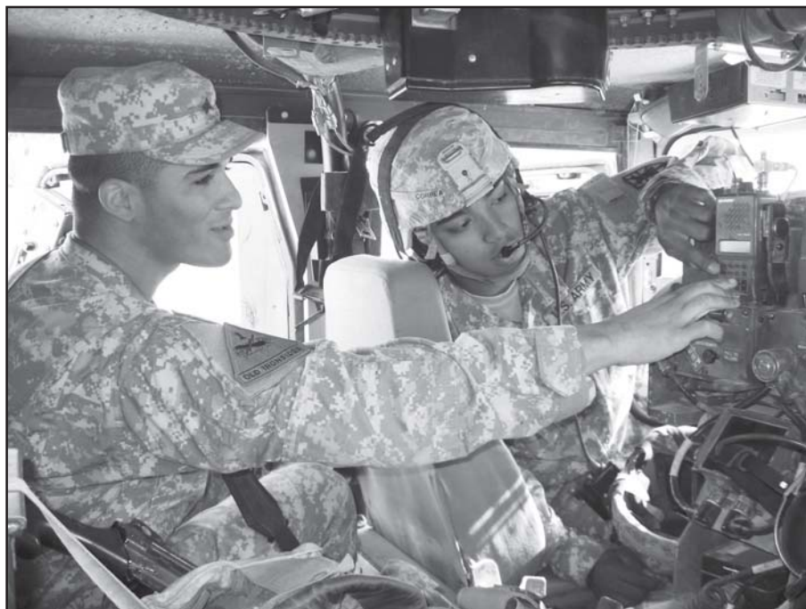
SSG Michael Browley, COB Adder RTO, gives instruction and observes as SGT Michael Correa (right) troubleshoots the AN/VRC-152 Harris radio system.
