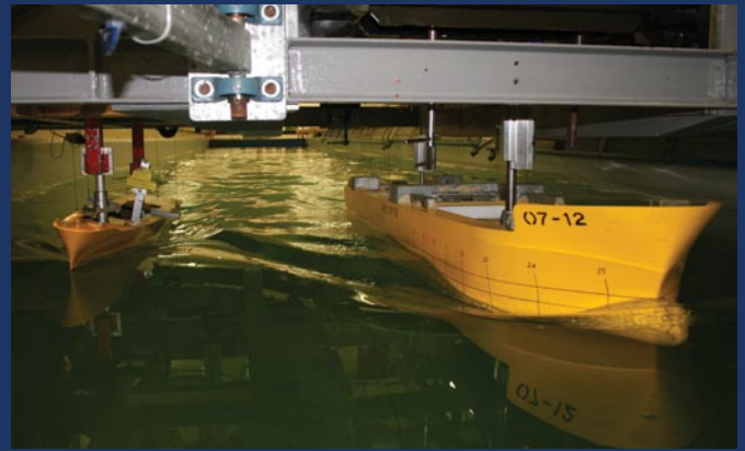
Above: tank testing for RAS research at the Australian Maritime Hydrodynamics Research Centre in Tasmania.
