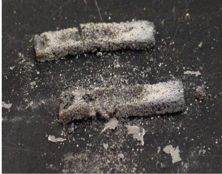
Figure 19: Destroyed Hexaaluminate Combustion Catalyst coated FeCrAlloy Foam
