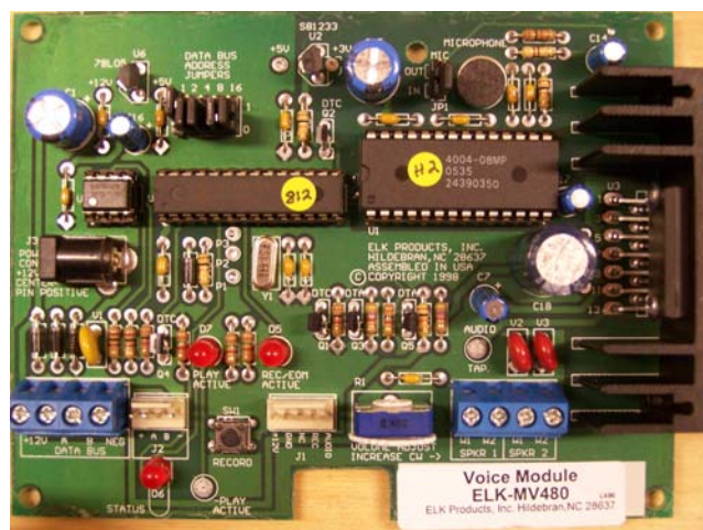
Figure 5. MV480 Recordable Voice Module
