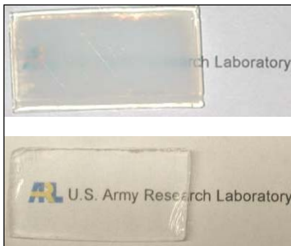
Figure 4. PMMA-filled Vycor specimens polymerized quickly outside of the solution (top) and polymerized slowly in solutions of decreasing initiator concentration (bottom).
