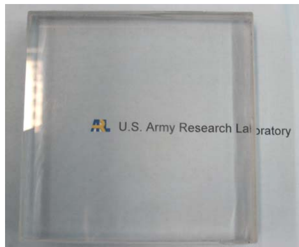
Figure 7. Laminate of polycarbonate and borosilicate glass (9 mm) and polycarbonate (5 mm) with Vycor-PMMA interlayer (3 mm).
