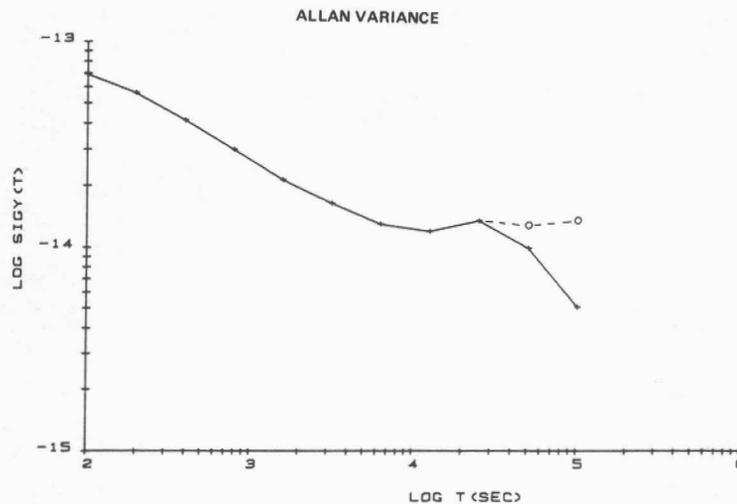
Figure 8. Root Allan Variance. The broken line is for the data of Figure 6, the solid line for that of Figure 7.
