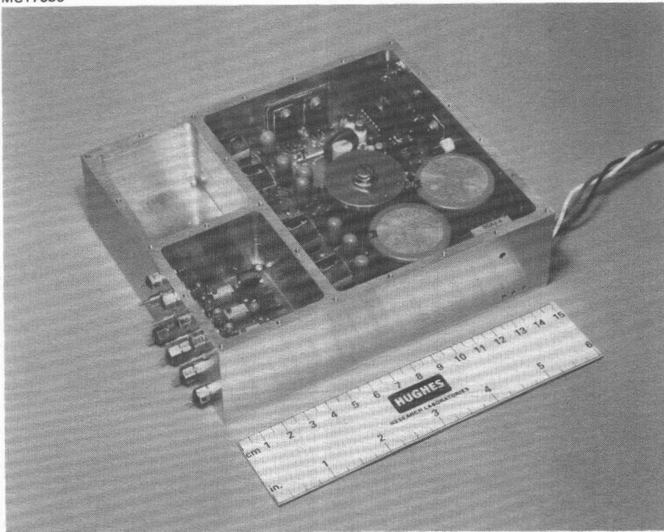
Figure 9. Low-noise multiple-output 100-W switching power supply.
