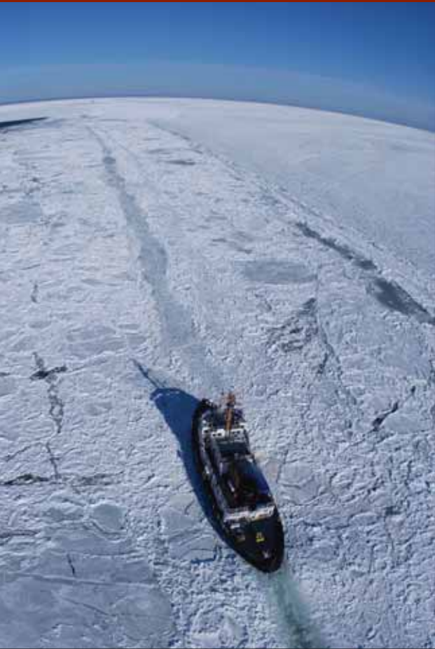
Coast Guard Cutter MORRO BAY, a 140-foot ice breaking tug, opens a shipping lane in the ice-bound Nantucket Sound.
