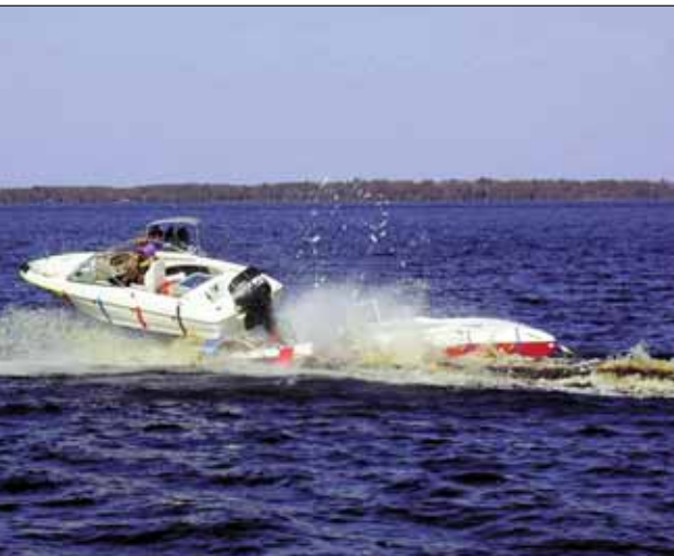
Two boats collide during a crash test to gather data on the applicability and effectiveness of federal recreational boating safety regulations.
