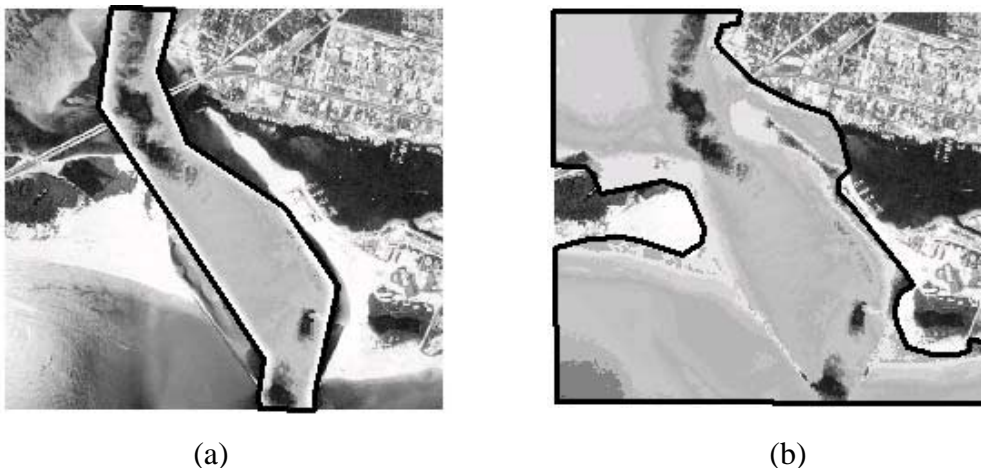
Figure 1.1: Conventional USA project survey plan (a) versus airborne lidar survey plan (b).
