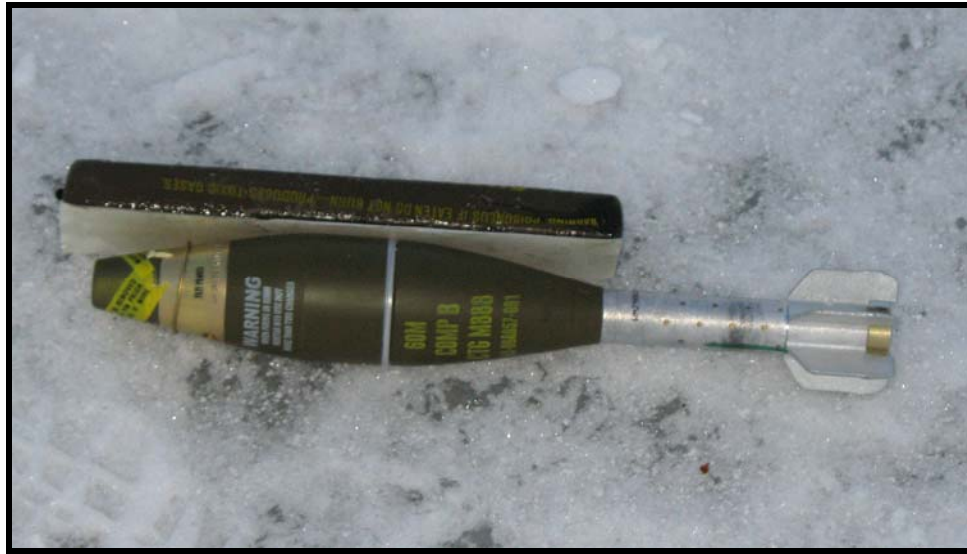
a. M888 60-mm HE cartridge with M112 donor charge on ice surface.
