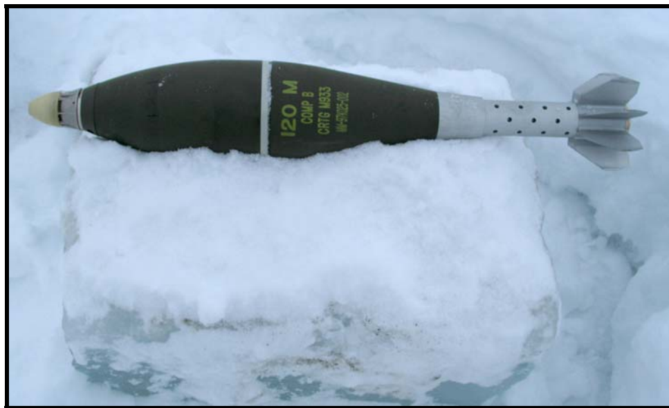
b. M933 120-mm HE cartridge on ice block.
